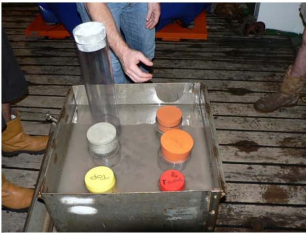
Box core from station JC18-8 with multiple sampling tubes inserted. Note, clear water on top indicates good preservation of sediment-water interface.
