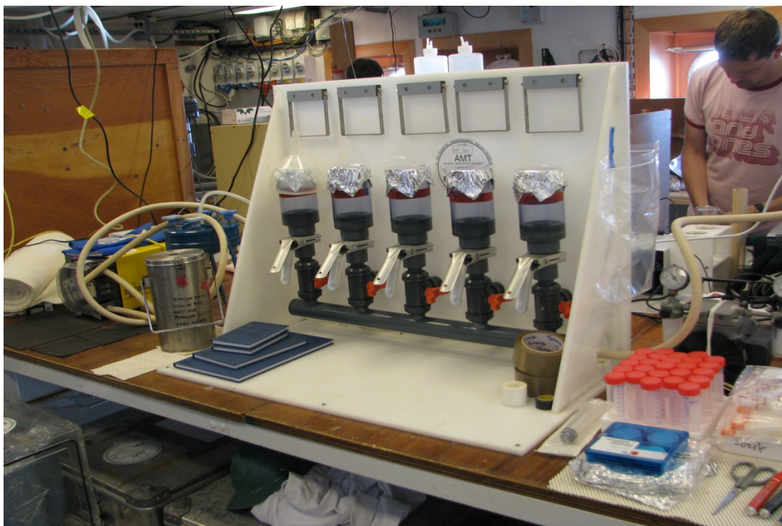
Fig. 1 The rack used for the filtration of the five depths sampled daily along the AMT-20 transect.
