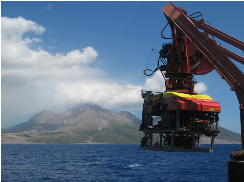
**Figure 5.** Isis with vibracorer attached.
