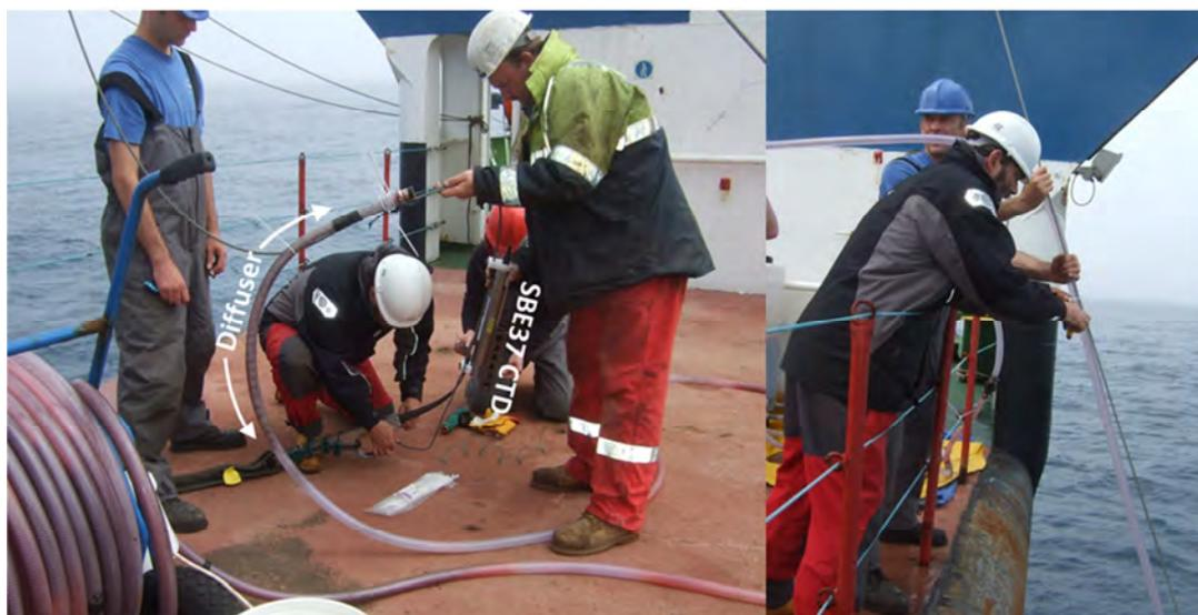
**Figure 1.1:** Hose, diffuser and CTD configuration for release #1. Photo: Jaimie Cross.
