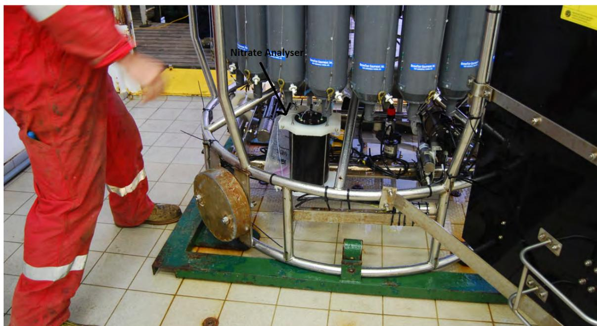
**Figure 6 Nitrate analyser mounted on a CTD**
