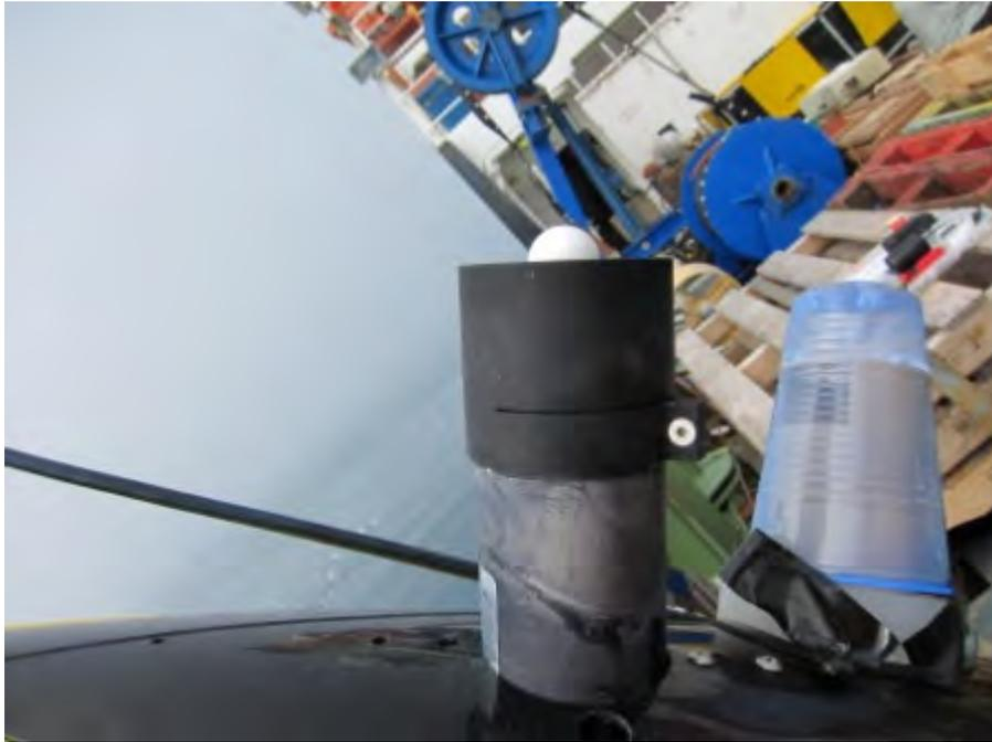
Fig 2. PAR sensor with light shield in deployment position. (The drinking cup in the right back ground is to prevent airbourne debris from damaging the NOCS Fast CT sensor.)
