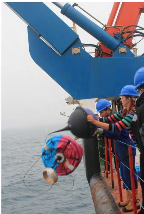
Figure 1: The deployment of one of the 15 m drifters from the stern of the ship.
