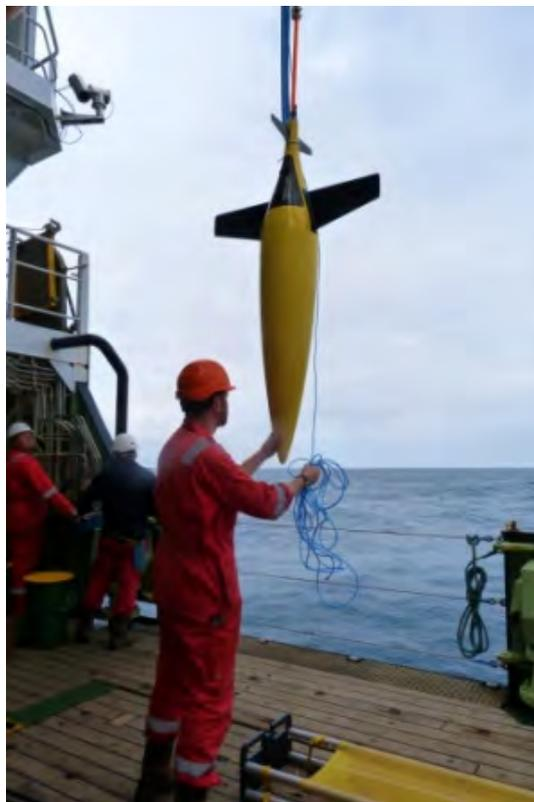
Fig 1. Vertical deployment method for the Sea glider. (Note blue alcaten pipe on the lifting rig, to prevent the lines twisting and snapping the antenna.)
