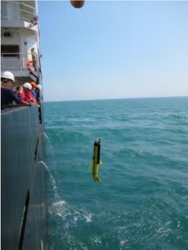
Fig 11. OMG glider being lifted on winch on stbd gantry. Line well clear of the turbulence sensors.
