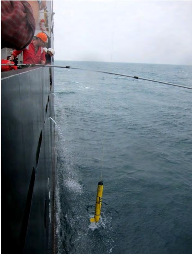
Fig 6. Glider being lifted from the water via the nose recovery line. (This line was shackled onto the rozler winch Kevlar line on the stbd gantry.)
