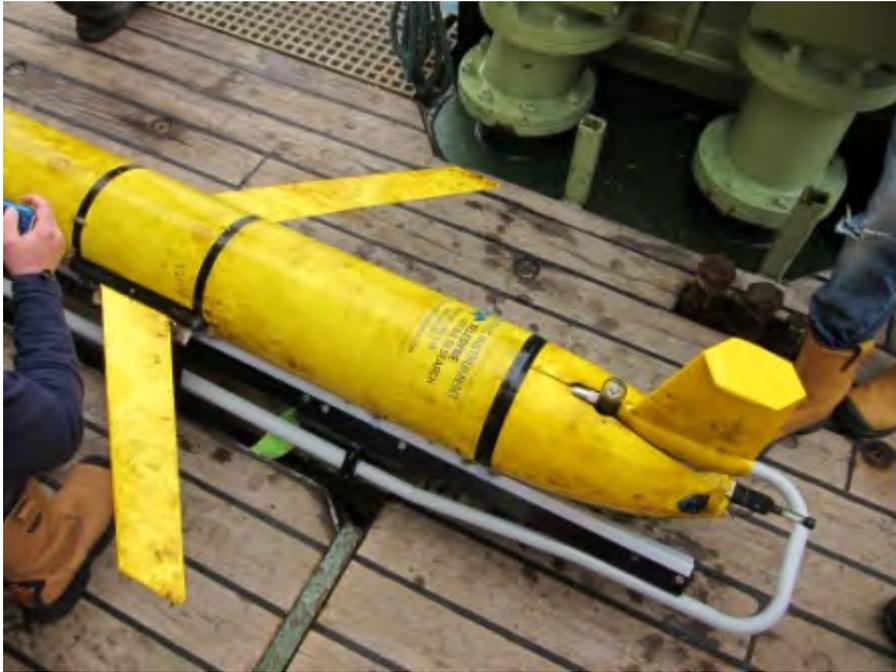
Fig 7. Bio fouling on the glider was fairly minor on most surfaces. Light coating of algae with some goose necked barnacles.
