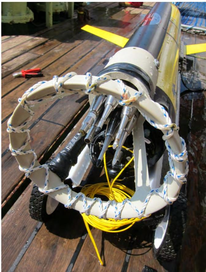
Fig 12. Photo of turbulence sensors, complete and having sustained no visible damage in recovery.
