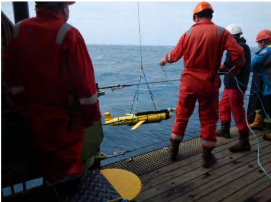
Fig 4. OMG glider being lowered to water line to be deployed.
