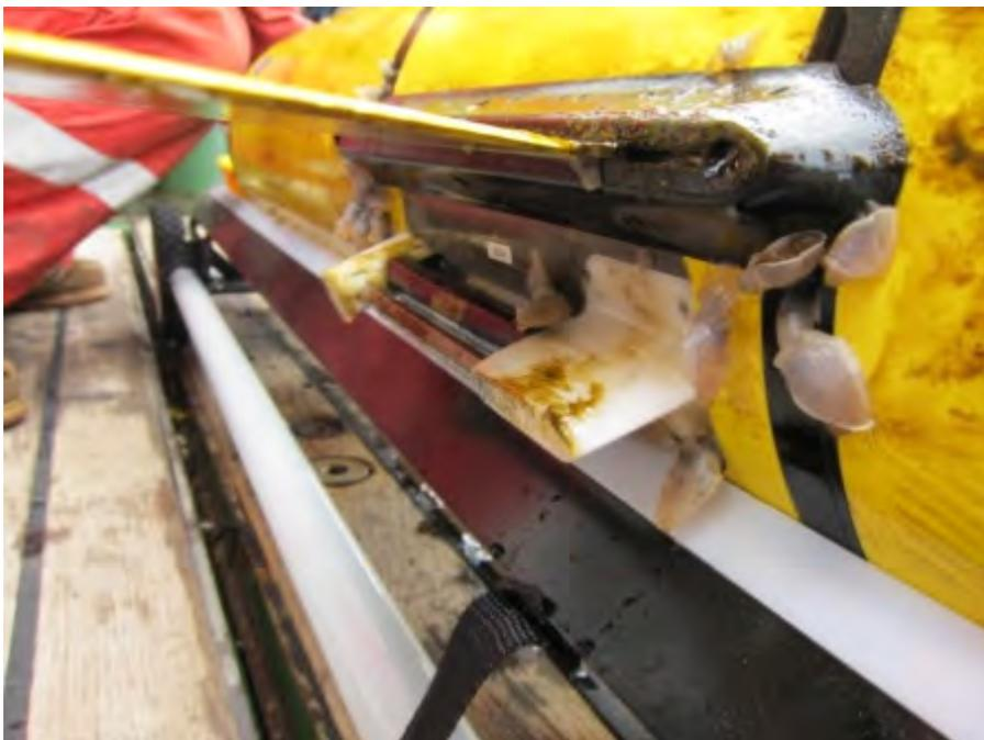
Fig 8. Close up of barnacles around the Seabird CTD. No significant bio fouling was noted on the intake/outtake ports.
