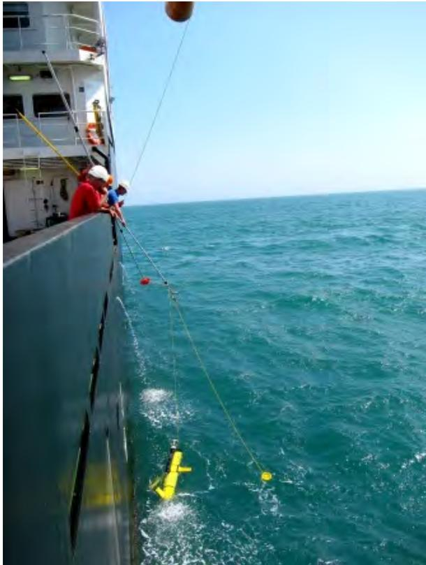
Fig 10. OMG glider with nose cone released, recovery line picked up with modified boat hook.
