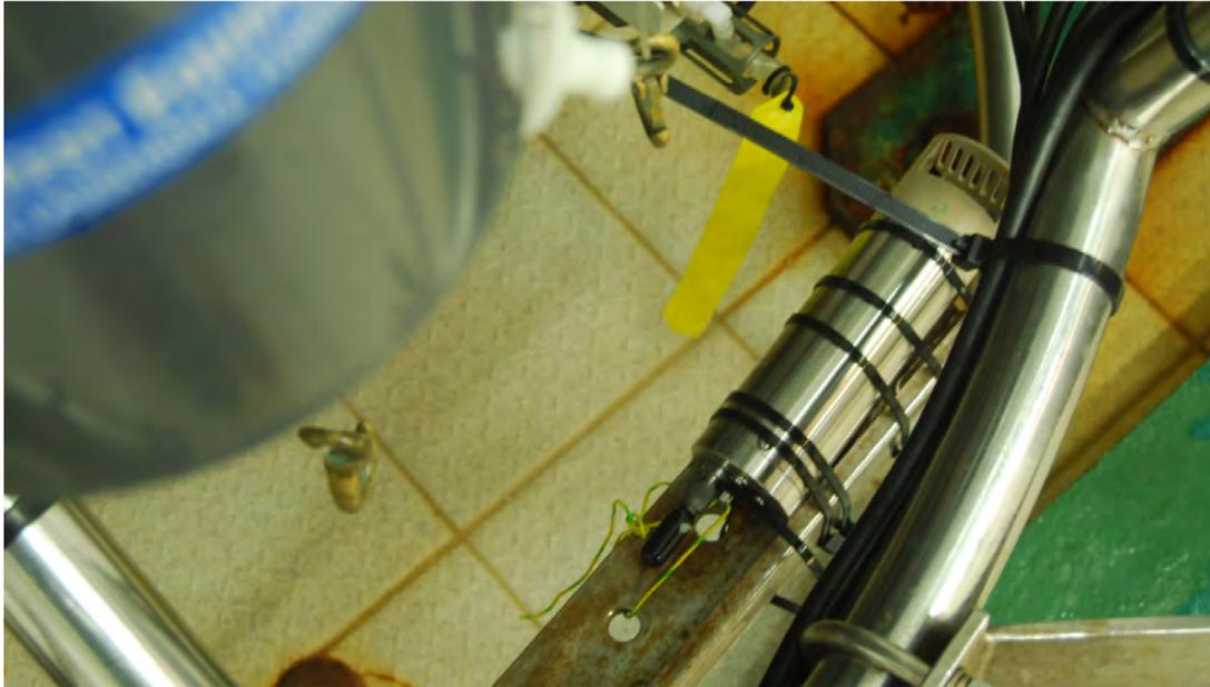
Figure 3 fast CT sensor mounted on a CTD
