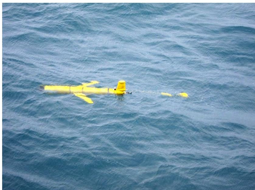
Figure 5. U 345 with nose cone released (seen on the right hand side of the image), with line paying out behind the glider. Note that the recovery line is not fully streamed.
