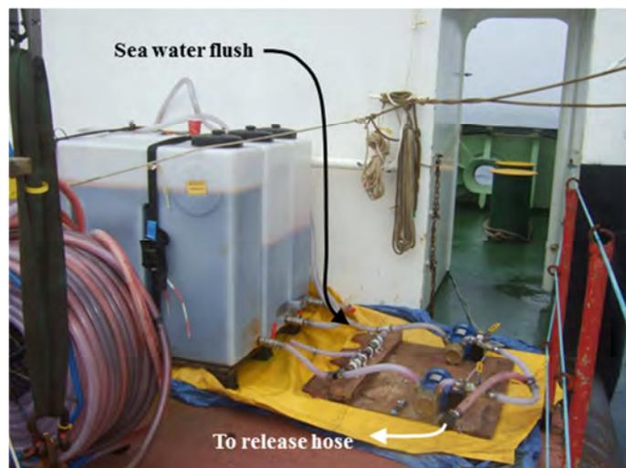
**Figure 1.2:** Plumbing configuration for release #1 (from the nearest tank, Tank A). Photo: Jaimie Cross.
