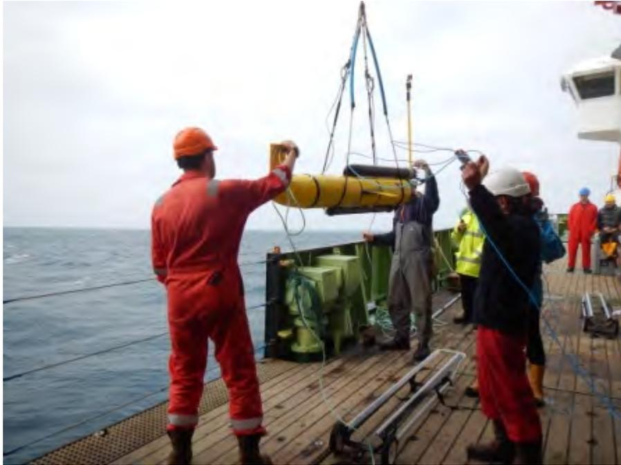
Fig 3. OMG glider being lifted into deployment position. Note weighted free running spreader bar underneath glider.
