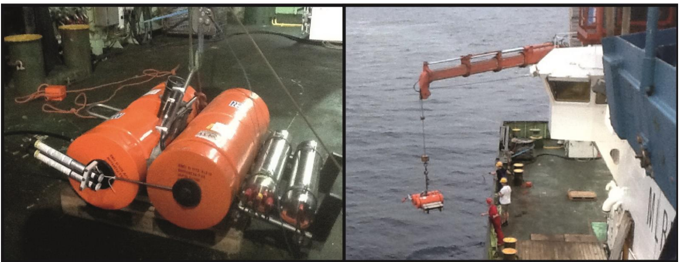
Figure 6 Photograph of a DEPAS BBOBS on deck and during initial deployments.
