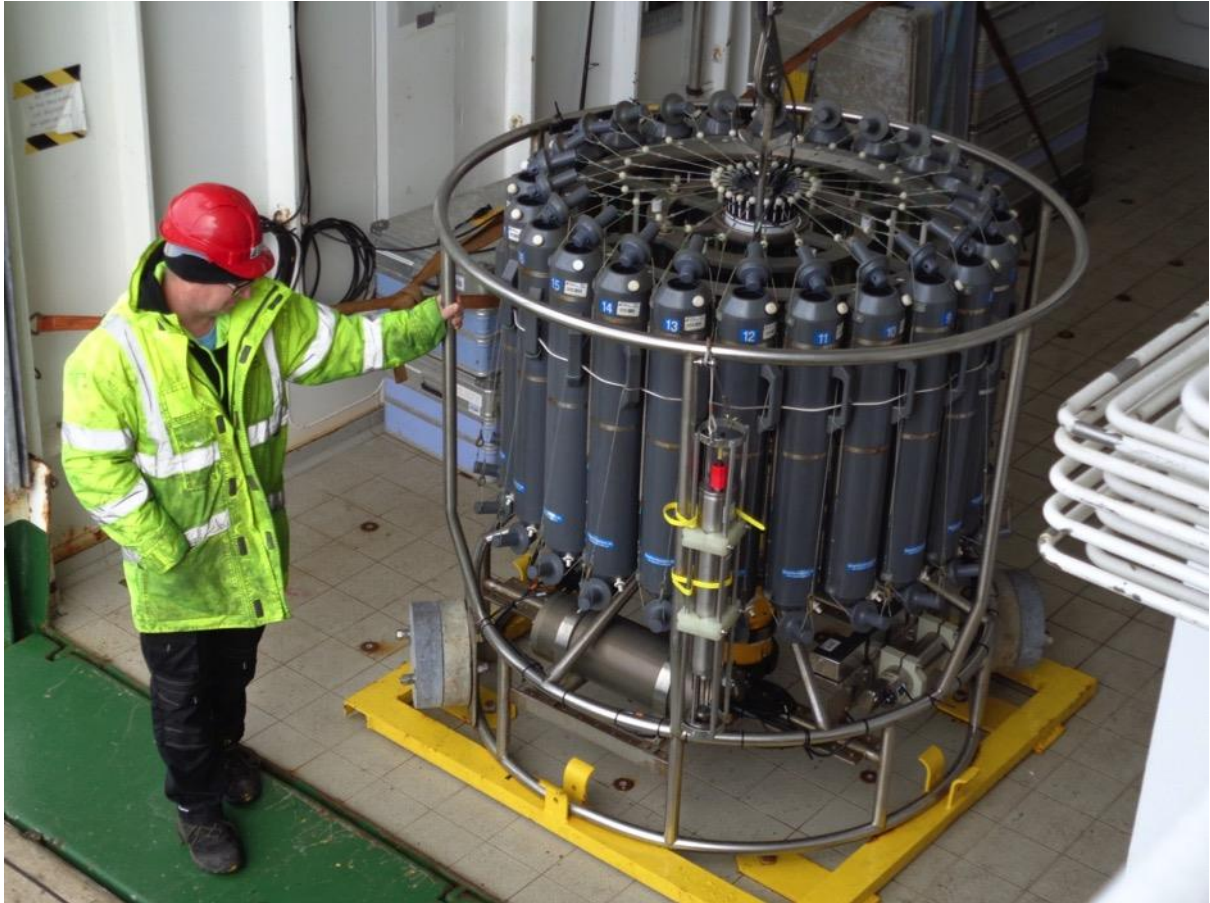
Figure 7.23: CTD zone Sea-Bird 9plus with downward-looking LADCP.
