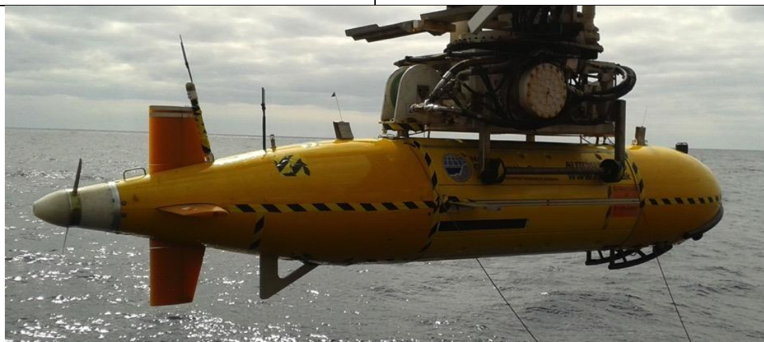
Figure 6.4: Autosub6000 on gantry before launch during the JC136 cruise.
