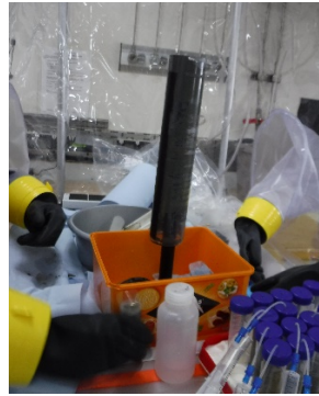
Figure 8.2 a) nitrogen filled glove box in CT lab; b) extruding and slicing a core inside the glove box; c) and d) porewater extraction from sediment slices with rhizon and syringe.
