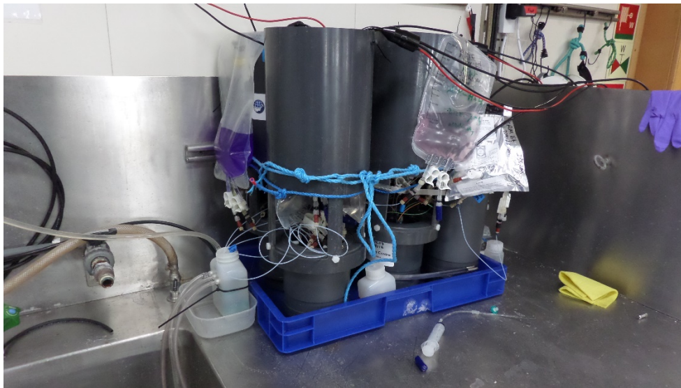
Figure 10.7. 5 LOC sensors sampling from the ship's underway system.
