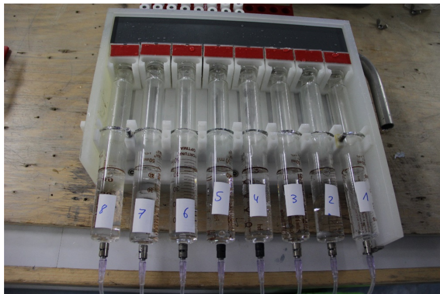
Figure 11.3. The eight syringes filled with seawater in the syringe sampler (benthic chamber 2, deployment 1, May 15, 2019 at 7 pm). On this photo, syringes are numbered according to sampling order (sampling interval: 3 h 23 min).
