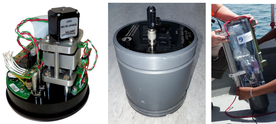
Figure 10.1. (Left) Interior of a lab-on-chip nitrate-nitrite sensor; (middle) sensor in a housing; (right) sealed sensor with a reagent housing on top
