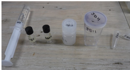
Figure 8.3 vials used for sub-sampling; from left: water extracted with syringe; glass vials for DIC/ \delta^{13}\text{C} and \delta^{18}\text{O}/\delta\text{D} ; acid-washed Nalgene bottle for cations; plastic pot for TA and nutrients; Eppendorf tube for anions.
