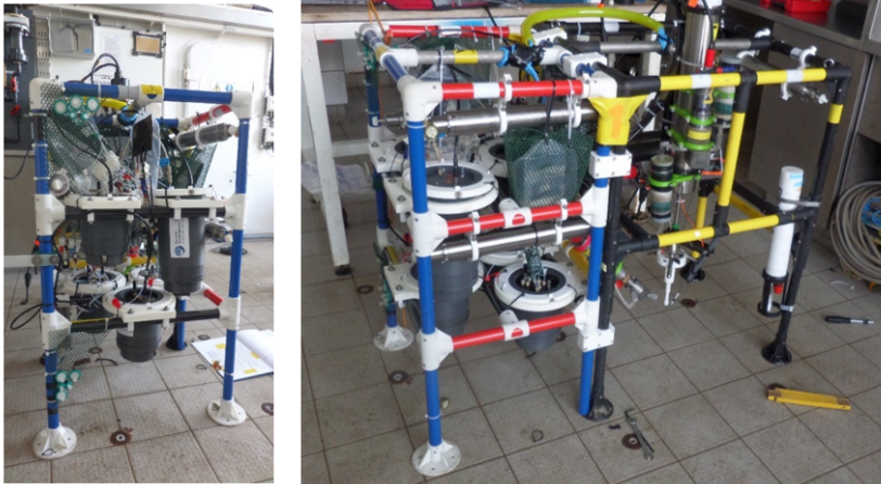
Figure 10.5. MPI BBL lander with the LOC sensors mounted on the blue and red portion of the frame. The photo on the left shows the (as-deployed) east side of the frame with the sensor intake filters at the top and bottom of the left-hand side of the lander. The right photo shows the north face of the lander.
