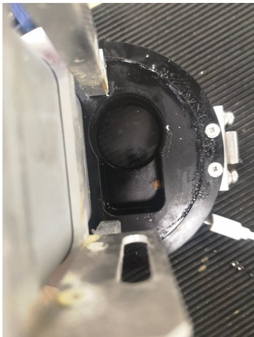
Figure 6.3. An internal view of the camera housing revealing the fatal screw that allowed water to enter. This was initially hidden from view as the Sony Action cameras sat directly over it.
