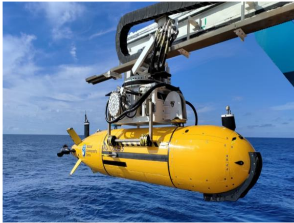
Fig. 5.9.1: Picture showing Autosub 5 vehicle on gantry before launch.
