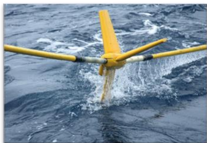
Fig. 5.3.2: Sercel streamer and a bird during deployment.
