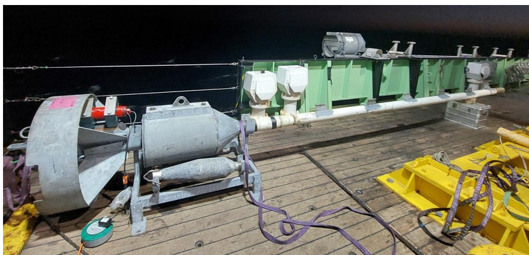
Fig. 5.11.1: Gravity corer with MTL mounts, welded onto the core barrel.
