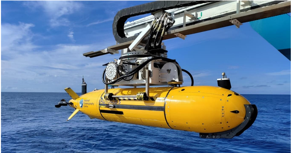
Fig. 7.1 Picture showing Autosub 5 vehicle on gantry before launch.
