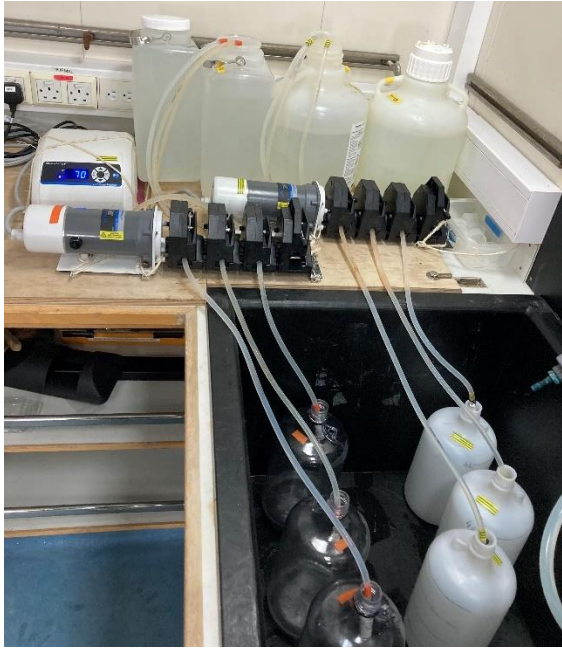
Fig. 6.91 Filtration setup in the lab using 2 peristaltic pumps.
