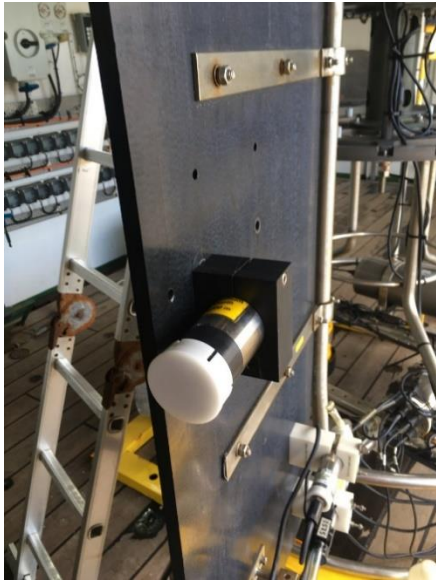
Fig. 7.118 WETLabs BBrtD Backscatter Sensor Mounting Location
