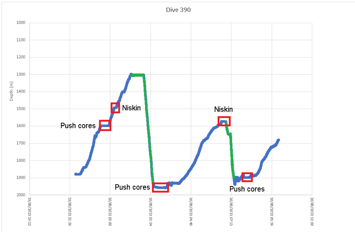
Fig. 6.49 Depth profile against time for ISIS ROV Dive 390, annotated with sampling events (red boxes) and mid-water transits (green track)
