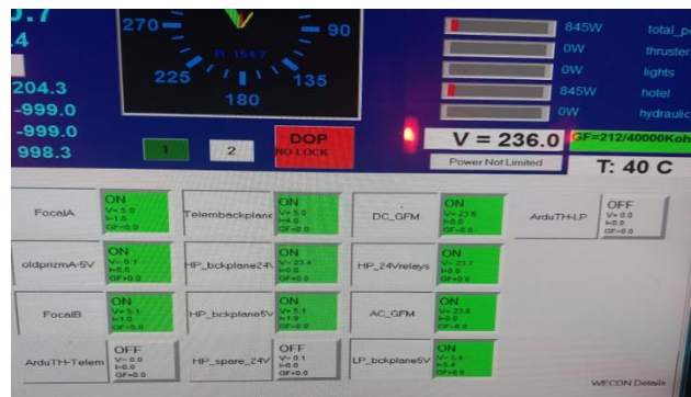
Fig. 7.112 Normal operation of the HOTEL tab and GUI with standard GF
