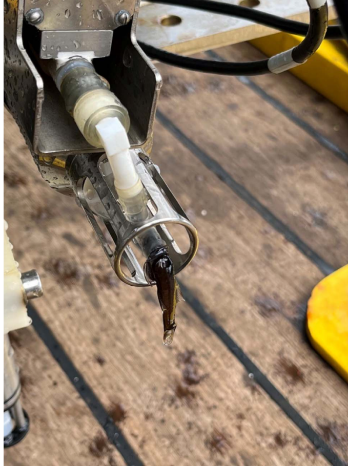
Figure 6.1 Fish blocking primary SBE 3P inlet.
