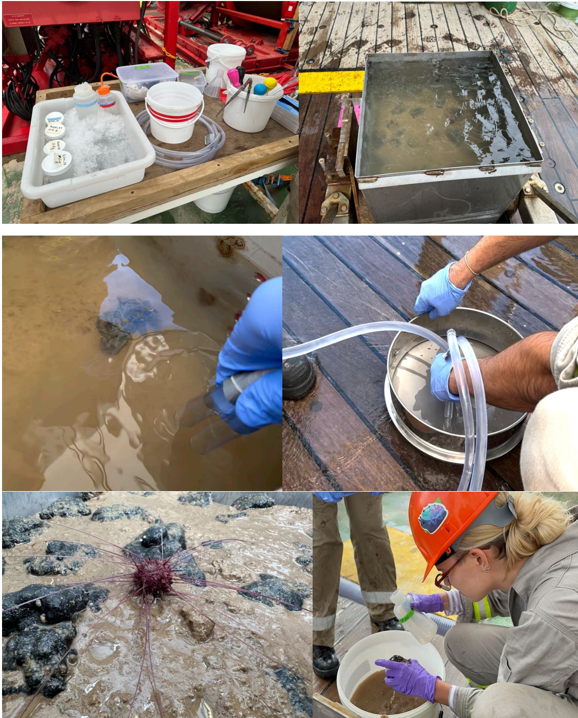
Figure 17.6 Deck processing of box cores on JC241 (1 of 2) Left to right from top row: 1) preparation of jars, ethanol, ice, camera equipment, 2) box core with clear topwater being moved to shade, 3,4) draining of topwater, 5) megafauna ( Plesiadiadema sp.) sitting on surface of box core after draining, 5) washing nodules into live-sort bucket. Photos by AG Glover.
