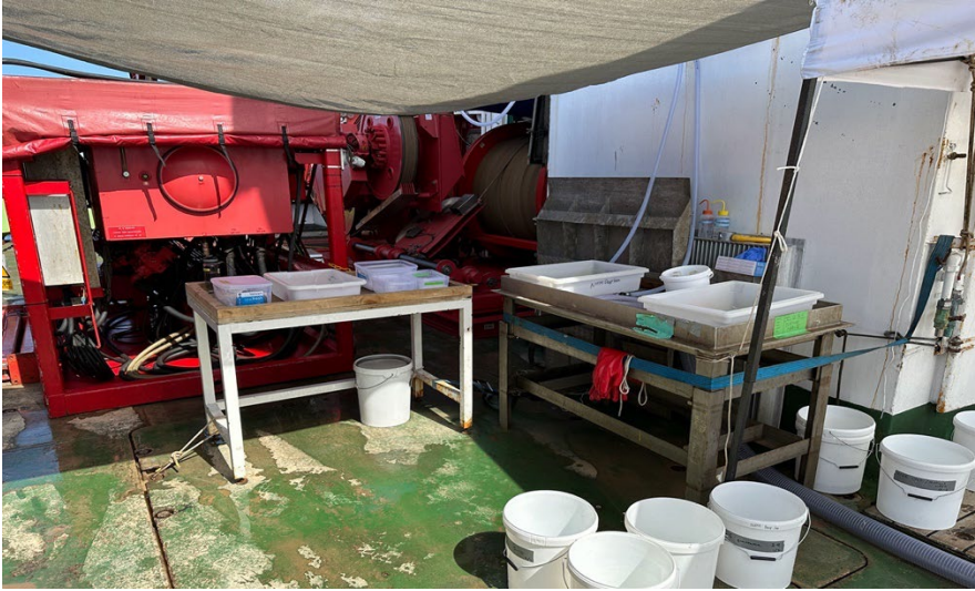
Figure 17.5. Complete sieving station with sieve trays, buckets, wash table and extra storage table. Note the sunshade essential for work in the tropics, and the large volume drainage hose running across the starboard deck. The box core was stored on the right next to the white buckets during sieving operations. Photo: AG Glover.
