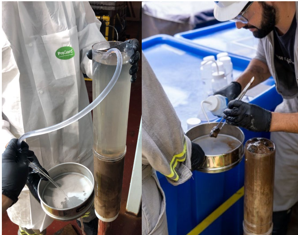
Figure 18.4 Steps 7 and 8 of the core extrusion protocol.
