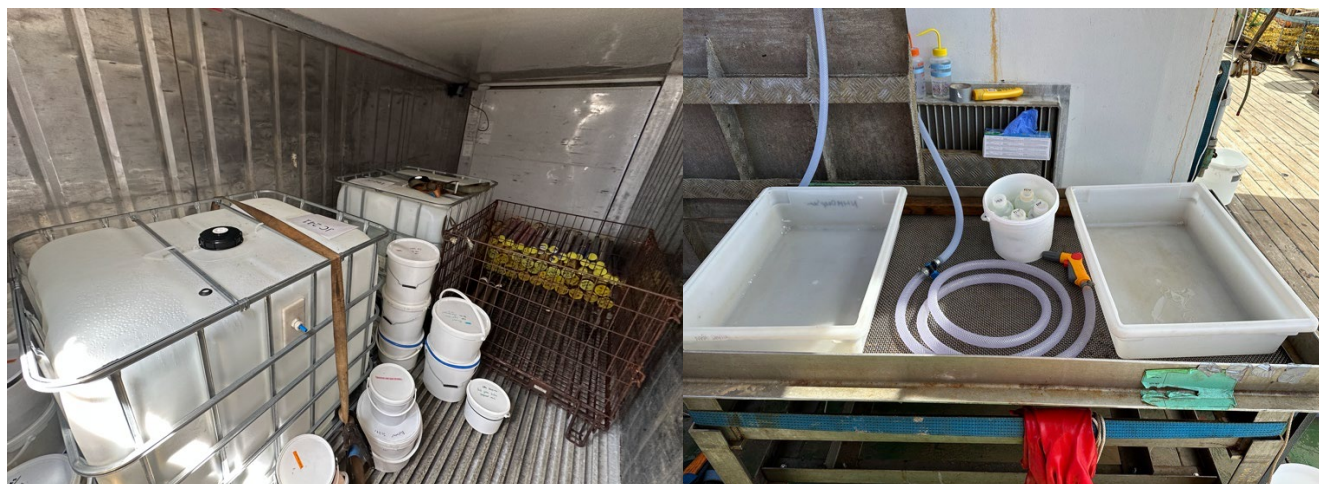
Figure 17.4. Left- 2 x Cold Filtered Seawater (CFSW) 1000L tanks setup in the 4C reefer van, Right - CFSW supply with 2 hoses to the Sieve table on the aft deck, starboard side. Photo: AG Glover.
