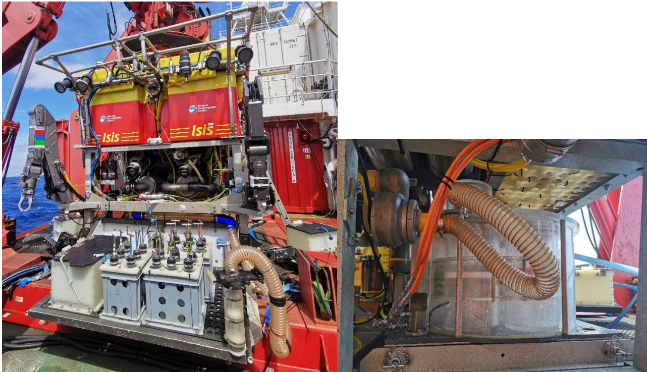
Figure 15.3.1.1. Left: ROV Isis configuration for sampling dives. Three bioboxes are mounted, a larger one on the front tray (grey biobox), and two smaller ones, one on each port and starboard swing arms. The slurp gun was also available on all sampling dives. Right: Canisters for collecting specimens with the slurp gun on the ROV Isis. The carousel is located at the back on the starboard side. Credit: G Bribiesca-Contreras.
