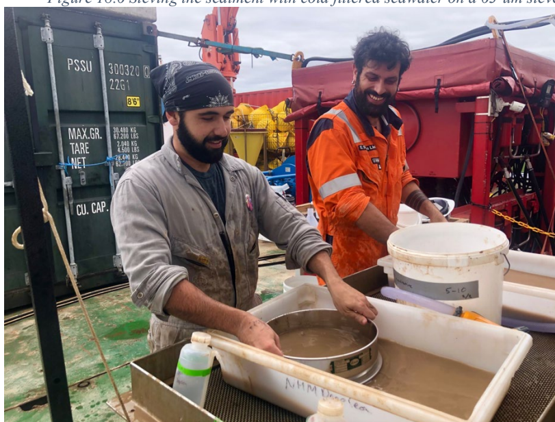
Figure 18.6 Sieving the sediment with cold filtered seawater on a 63-um sieve.
