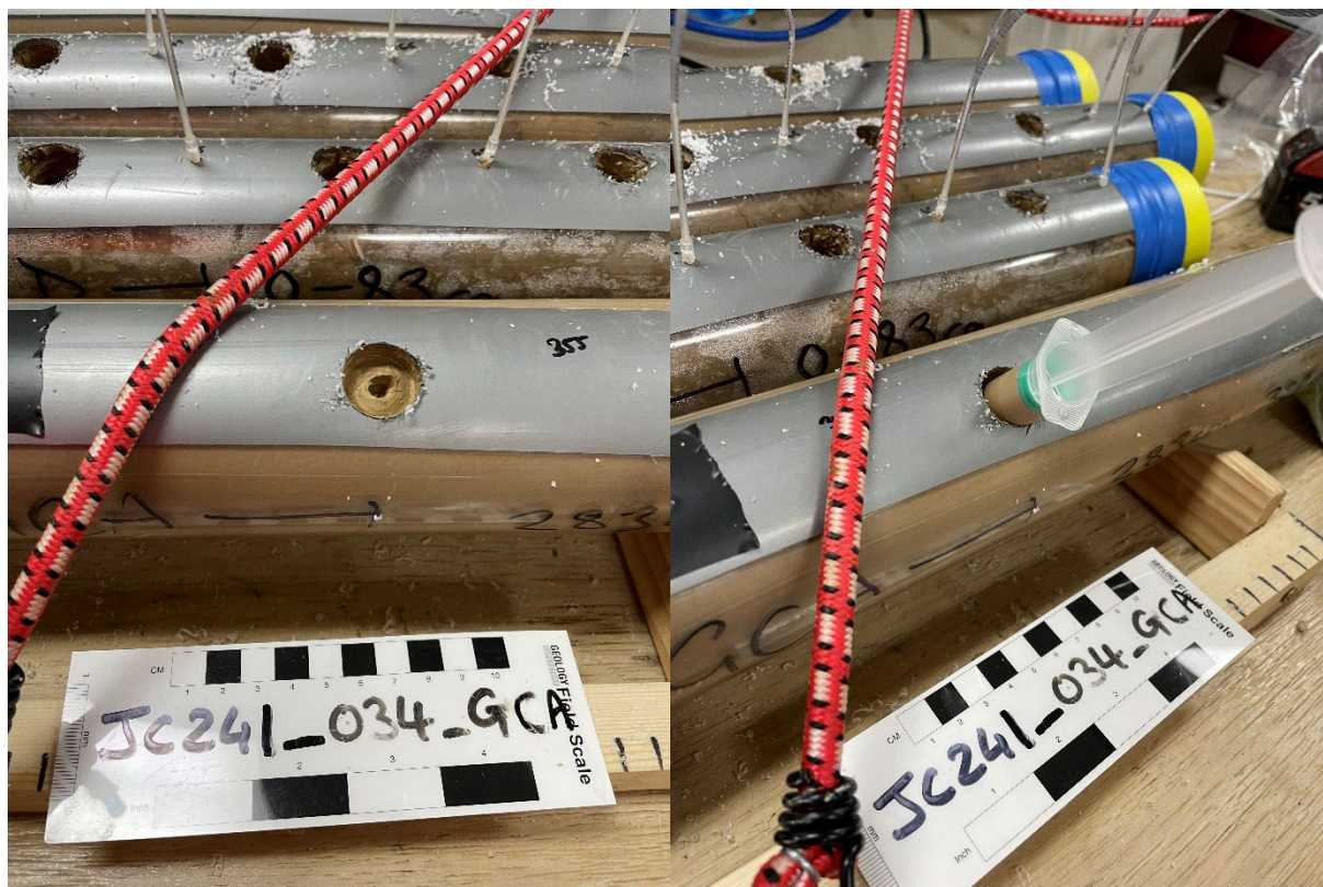
Figure 11.9: Example of sediment plug sampling from a gravity core.
