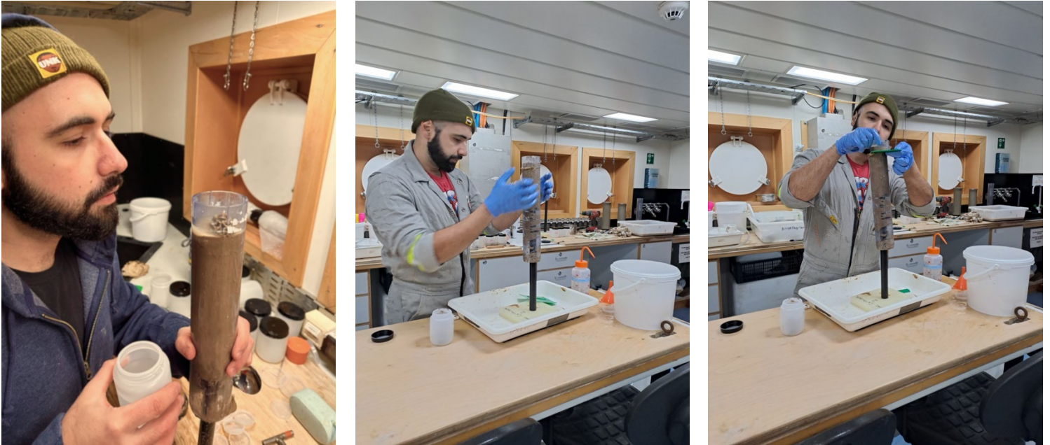
Figure 18.5 Steps 10, 11, and 12 of the core extrusion protocol.
