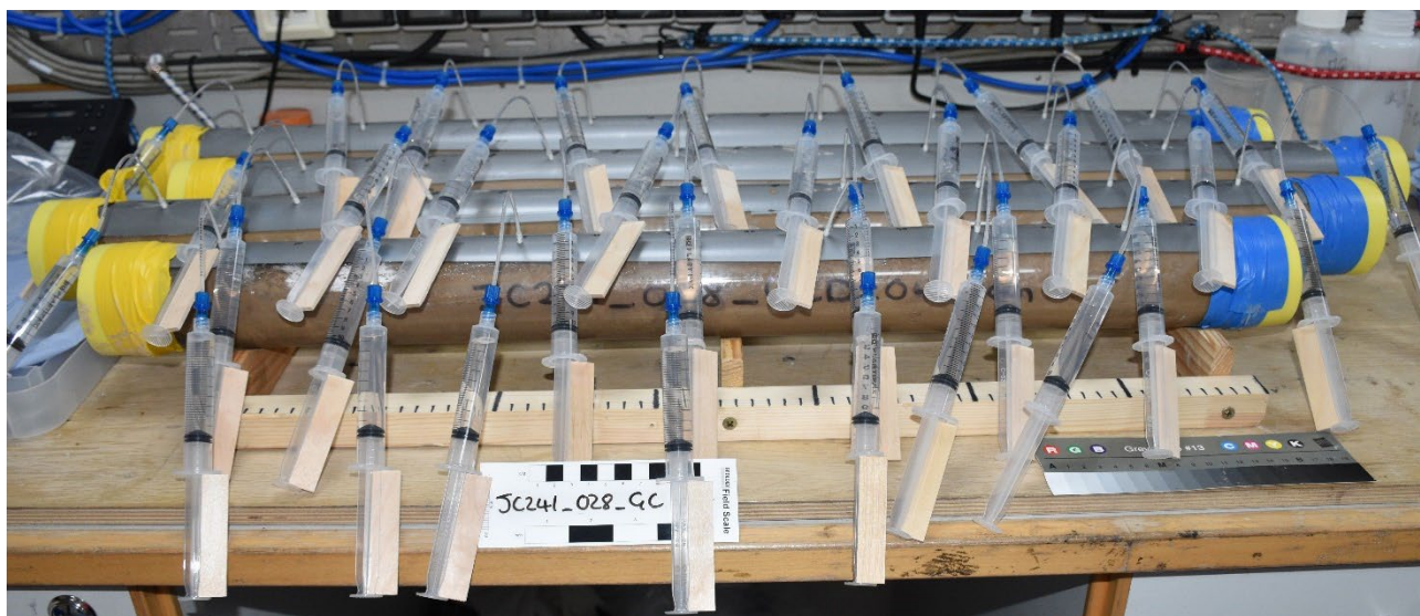
Figure 11.8: Pore water extraction example from a gravity core.
