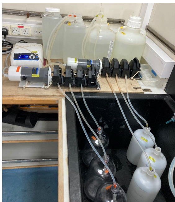
Figure 19.5. Filtration setup in the lab using peristaltic pumps.
