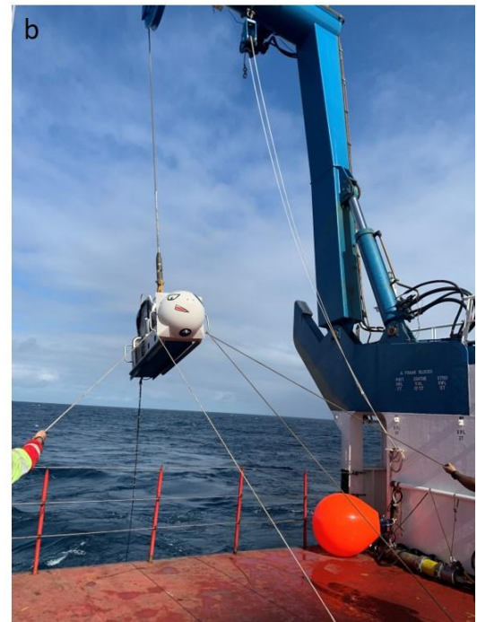
Figure 4: a) The LEM launcher getting ready to be deployed using the A frame. b) the same instrument being deployed.
