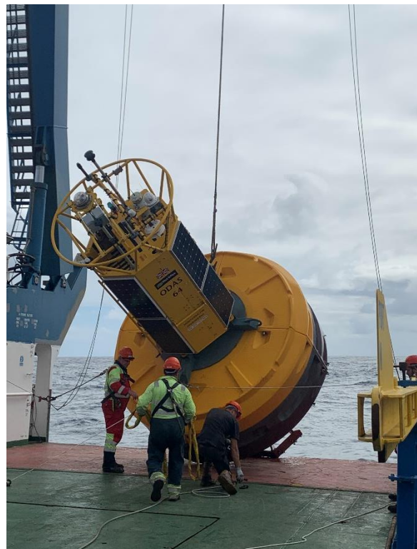
Figure 10: PAP buoy recovery.
