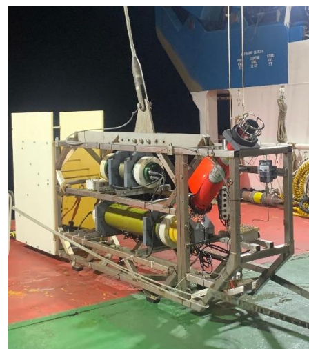
Figure 7: DASI on the aft deck before deployment. The front USBL and two tubes of DASI are visible.
