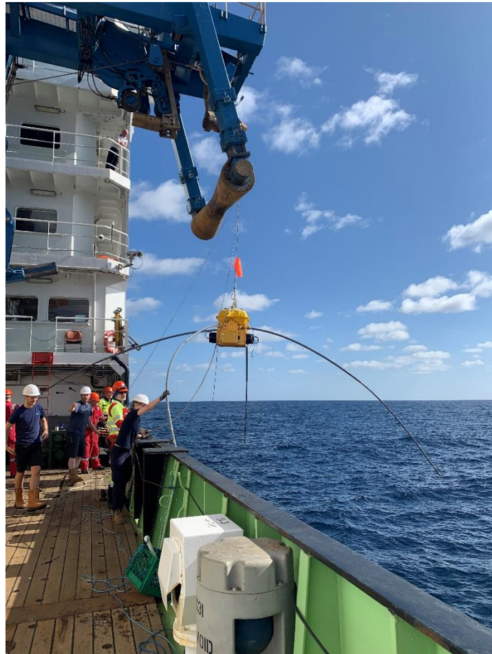
Figure 8: Recovery of a OBIC instruments using the starboard winch.
