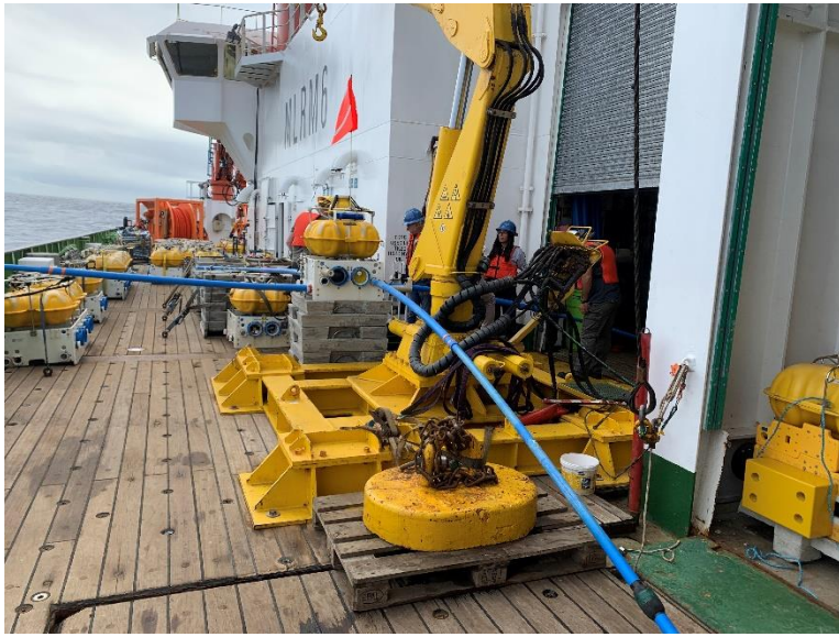
Figure 3: a) A Scripps OBI being prepared for deployment using the starboard crane. b) The same Scripps instrument is being deployed.
