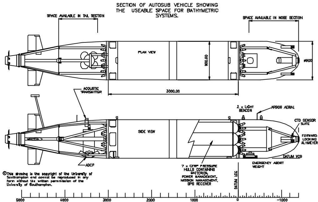
Figure 2.4. Vehicle layout showing sensor space and datum.
