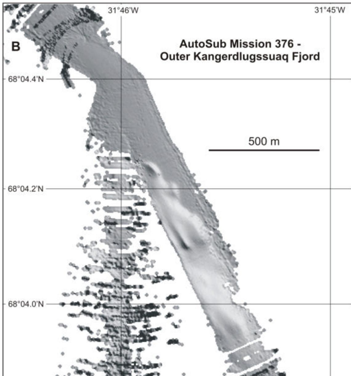
Figure 4.10. EM2000 shaded image of bathymetric data acquired during mission 376 of AutoSub in outer Kangerdlugssuaq Fjord.
