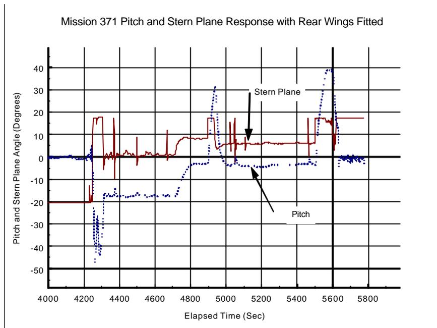
Figure 2.8. The time period from 5100 to 5400 seconds show the time of level, steady flight, this time with a less pronounced stern plane angle.
