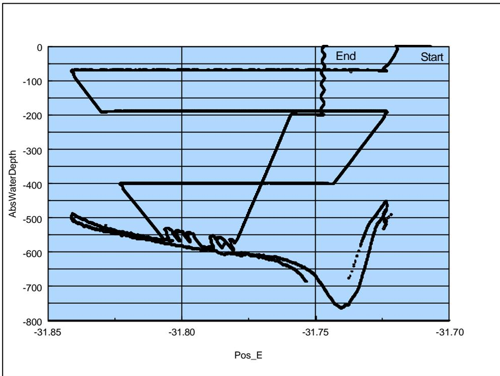
Figure 2.2. Mission 377. Final Autosub Mission of JR106b. Shows depth profile of Autosub track (verses longitude). Lower brown track is the seabed profile measured using the Autosub's downward looking ADCP.
