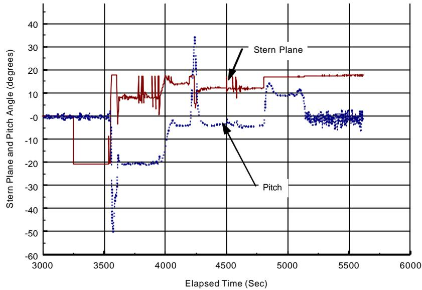
Figure 2.6. The time period from 4300 to 4700 seconds show the time of level, steady flight, the stern plane angle of 12 degrees is close to its full travel (17 degrees).
