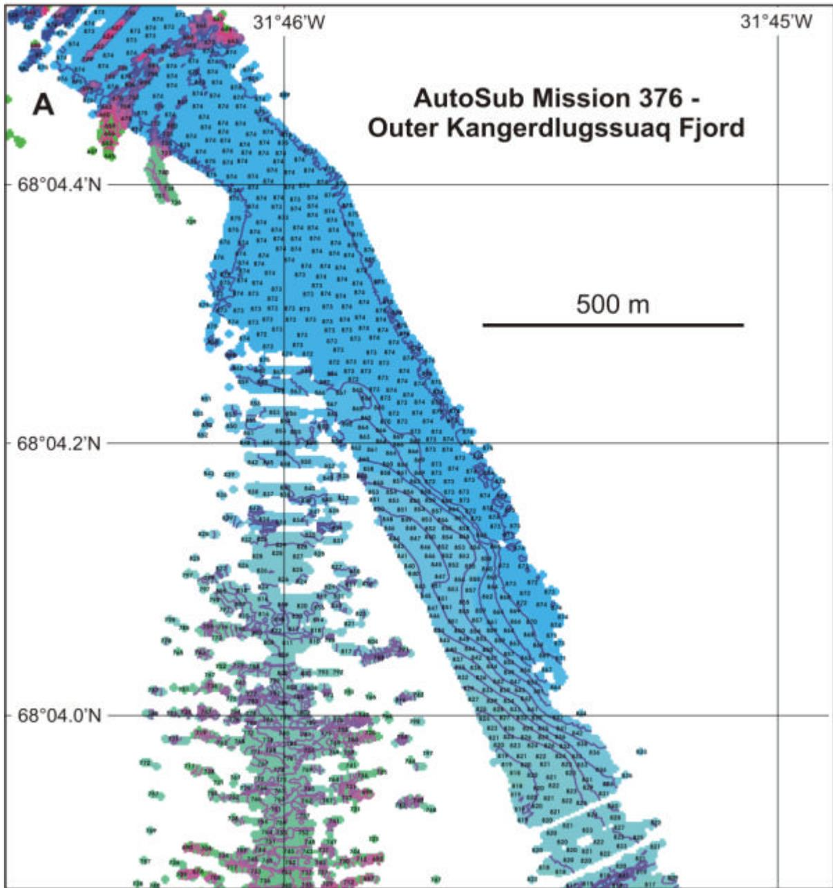
Figure 4.9. EM2000 bathymetric map compiled from data acquired during mission 376 of AutoSub in outer Kangerdlugssuaq Fjord. Water depths are shown and contours are at 5 m intervals.
