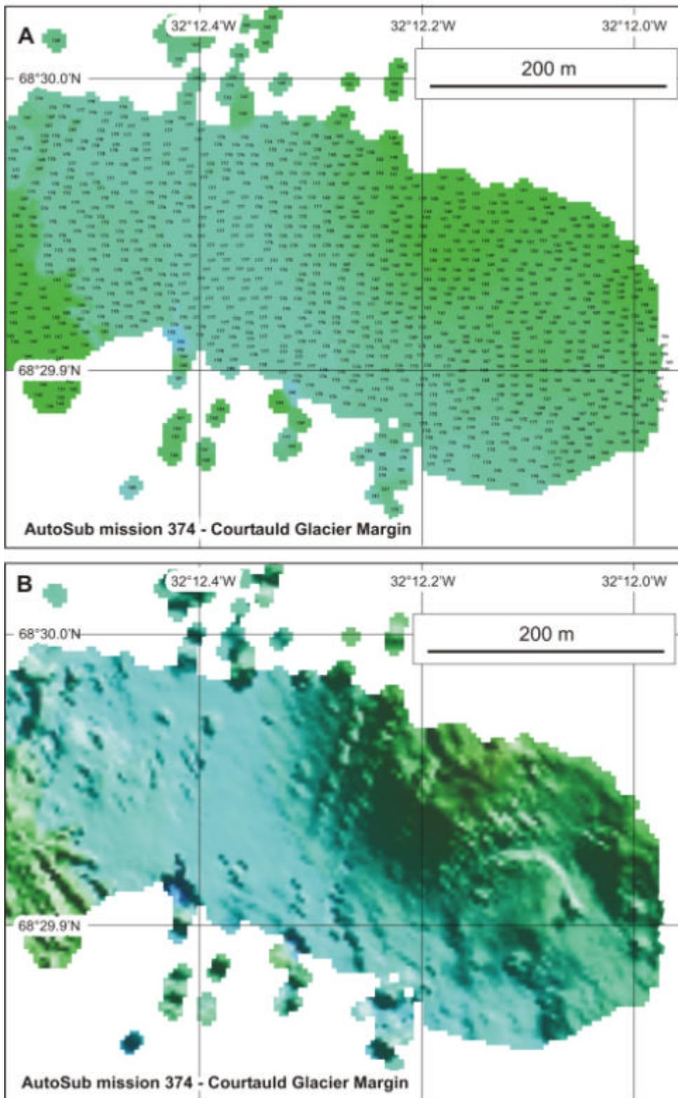
Figure 4.8. (a) EM2000 bathymetric map compiled from data acquired during mission 374 of AutoSub in front of Courtauld Glacier, Courtauld Fjord. Water depths are shown. (b) EM2000 shaded image of the sea floor compiled from the same data showing an irregular sea floor and a possible streamlined feature.
