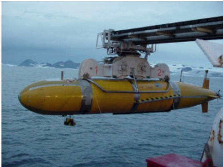
Figure 2.5 Slender wings fitted to rear half of the centre section
