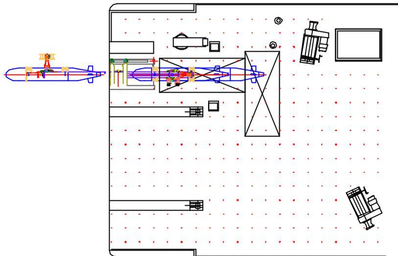
Figure 2.3 Plan layout of the containers on the aft deck
