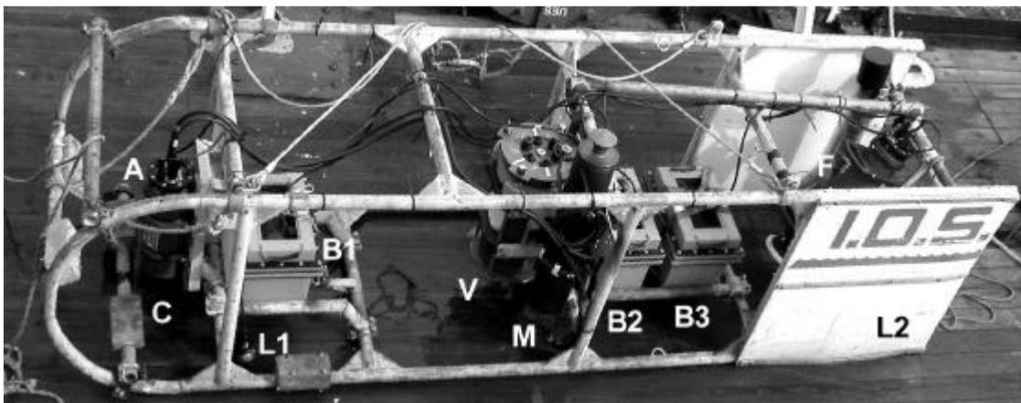
*The Southampton Oceanography Centre WASP vehicle, showing locations of A-altimeter, C-still camera, L-video lamps, B-batteries, V-video camera, M-monitor (acoustic telemetry) and F-flashgun.*
