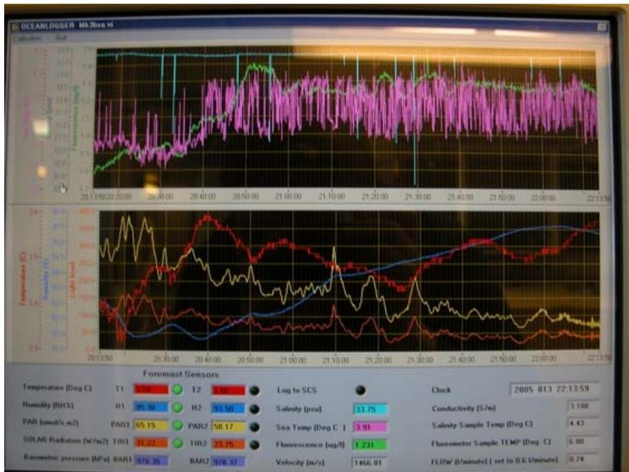
Photo showing Oceanlogger screen at 2215 GMT 13 January 2005. Temperature axis ranges from 3.5—4.1°C. Note the noisy sea temperature trace (magenta line).
