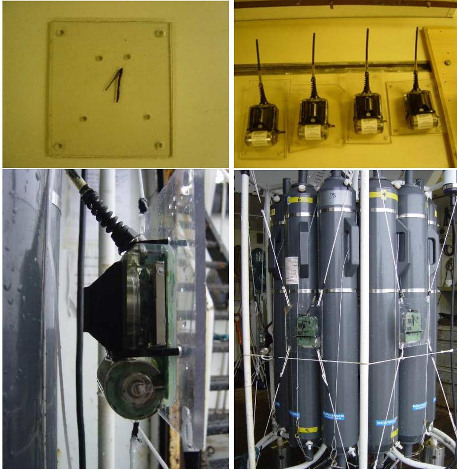
**Figure 1.1:** Plastic plates and how they were used to attach the tags to the CTD frame.
