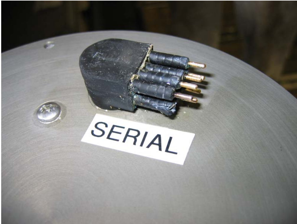
Pic. 1: corroded connector on WCP 1004
