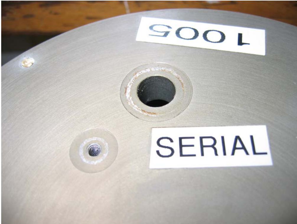
Pic 3: corrosion found around serial port and purge plug on WCP 1005
