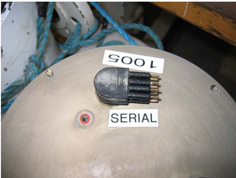
Pic 2: less corroded connector on WCP 1005 with purge plug removed showing disintegrated O-ring and corrosion around
