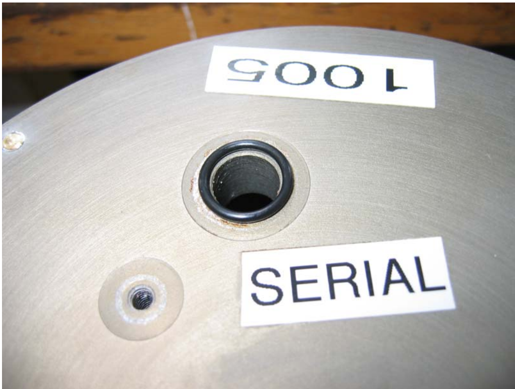
Pic 4: corrosion compared to location of O-ring of serial connector
