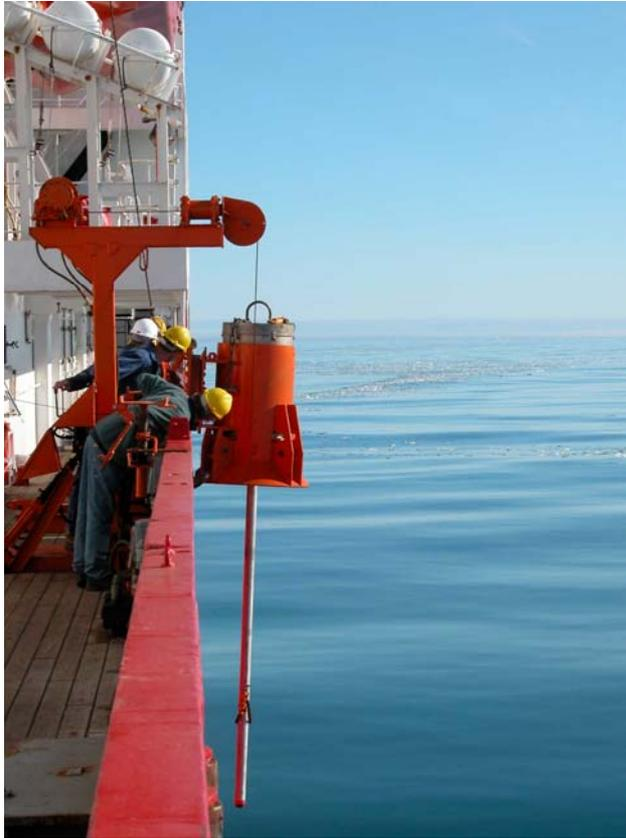
**Fig. 4.1. Gravity coring operations from the starboard side of the JCR in Hartogbukta, Nordaustlandet, eastern Svalbard.**
