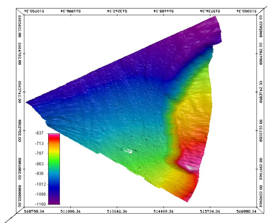
Fig.6.1. Shaded bathymetry (illumination from west) of the test site (line 0372 between 0511 and 0607). Switching from Deep to Medium ping mode occurred in the middle of the test area.
