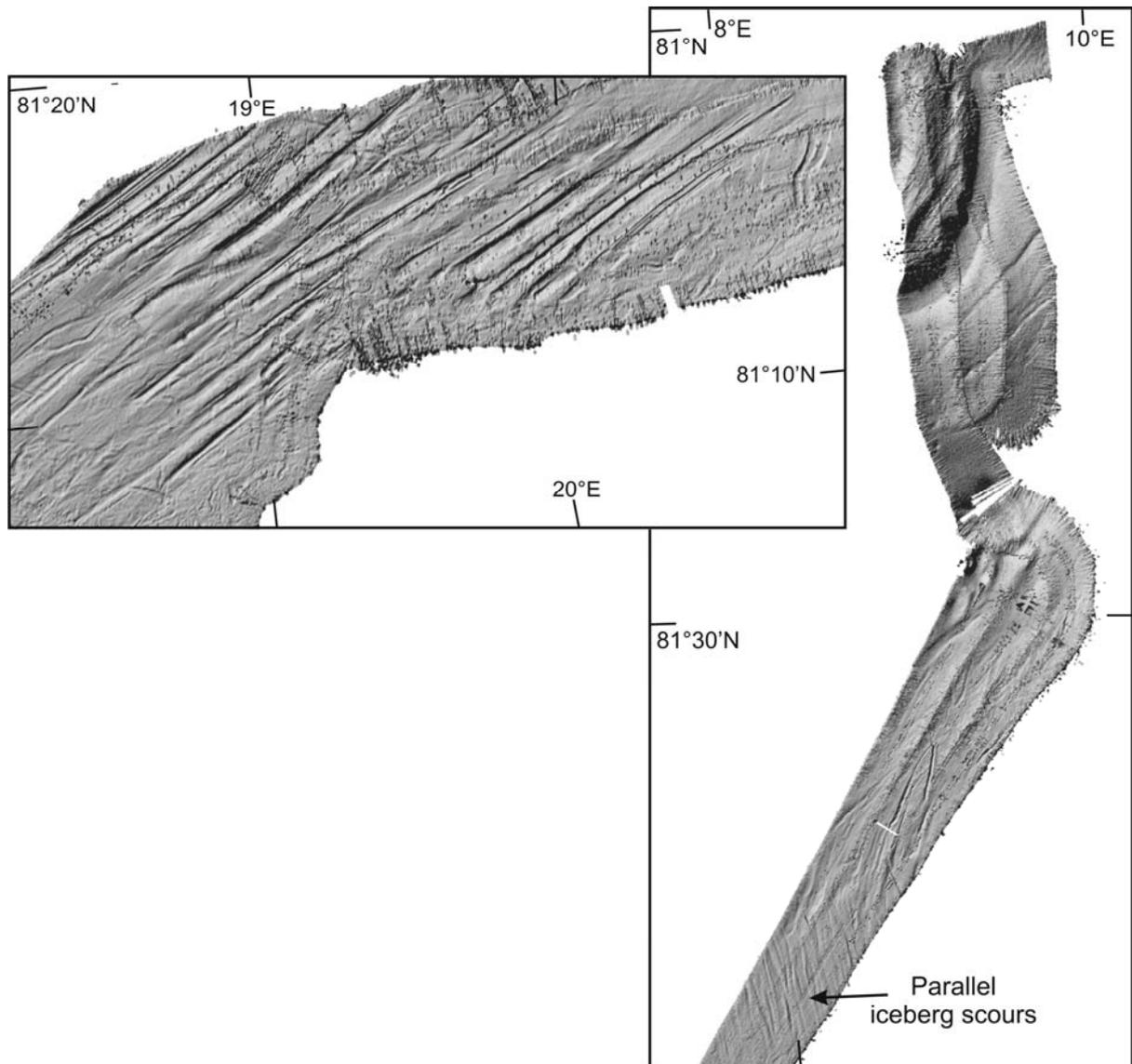
Fig. 5.4. Swath image of large iceberg scour marks on the sea floor in 500-600 m of water north and west of Svalbard on the Yermak Plateau. Note also the moat produced by the strong Spitsbergen Current in the right-hand image.
