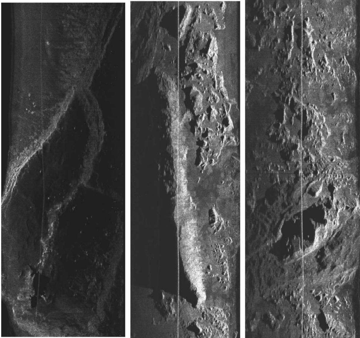
Fig. 5.3. Parts of the huge Hinlopen Slide, imaged by TOBI side-scan sonar. Each block of data is about 4 km across.
