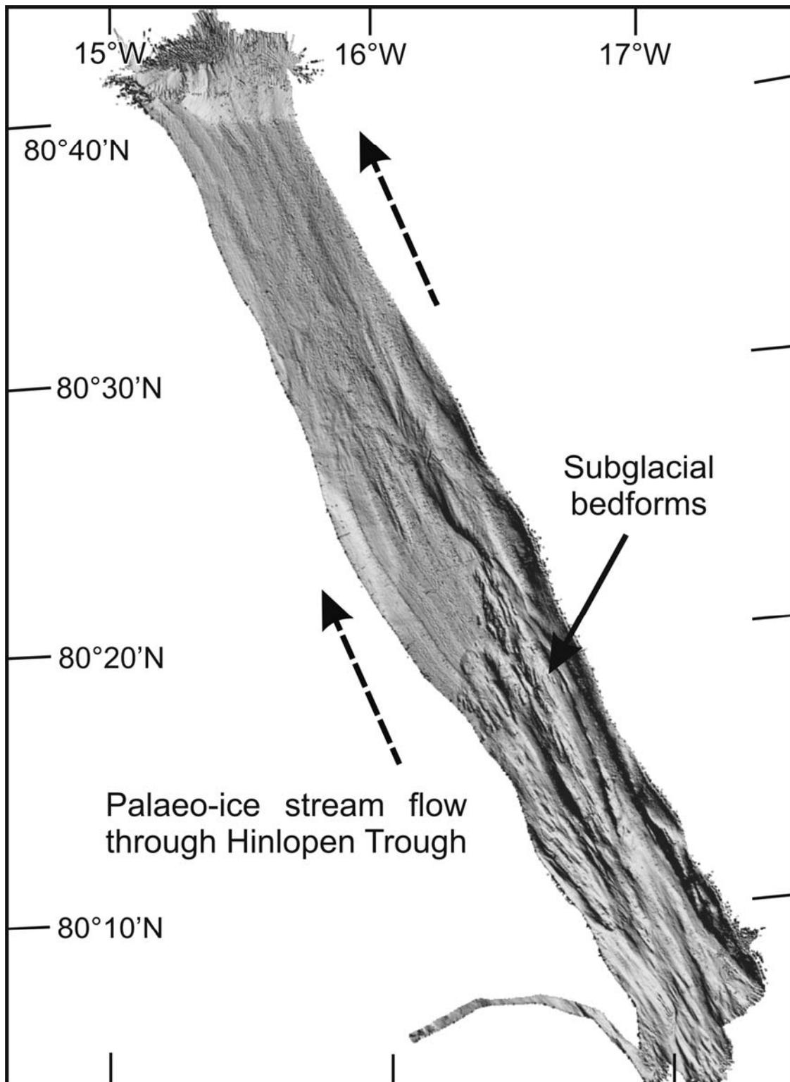
Fig. 5.2. Swath bathymetric imagery of Hinlopen Trough north of Svalbard. The trough is about 70 km long.
