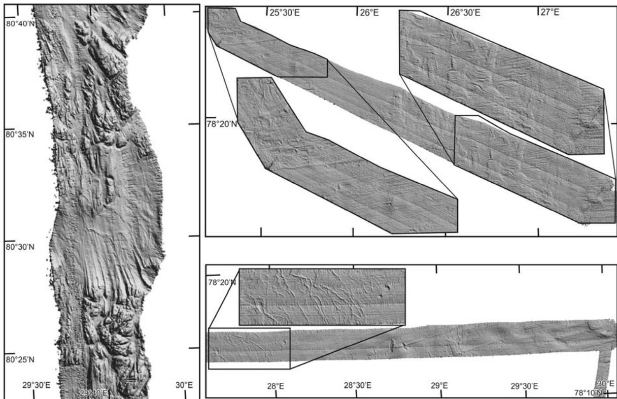
Fig. 5.1. Swath imagery from east of Svalbard: the Kvitoya Trough (left) and Olga Strait on the right. Note the streamlined sedimentary and bedrock features on the left and the series of submarine ridges on the right.
