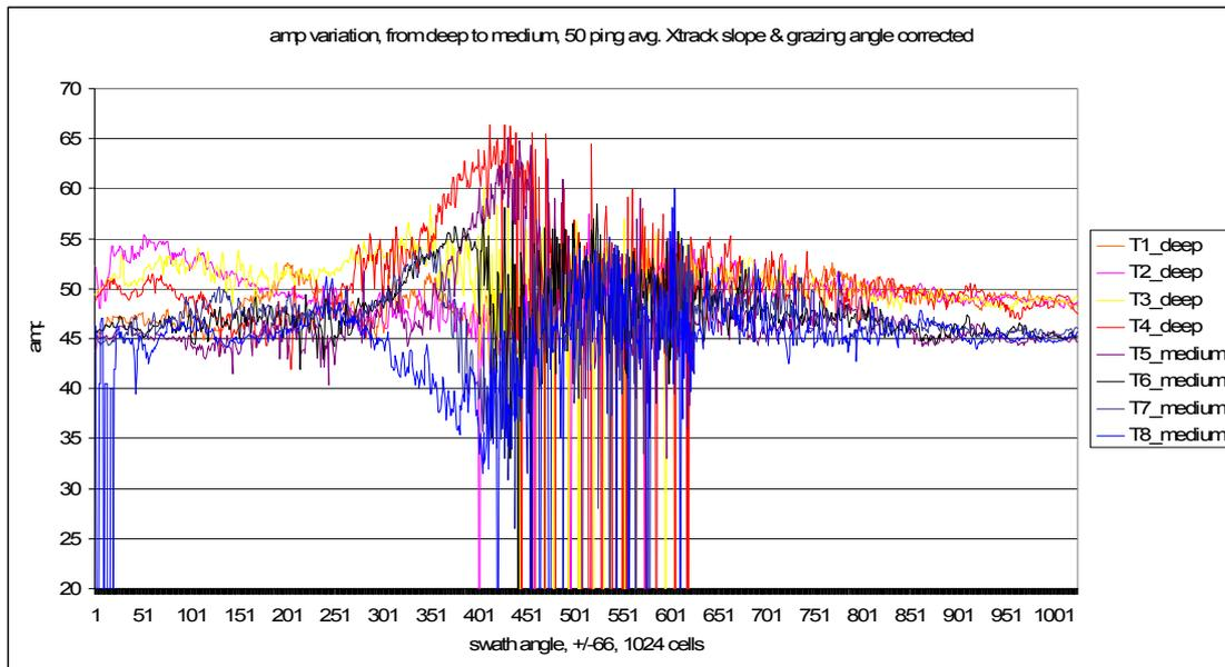
Fig.6.3. Beam amplitude levels sampled at 8 time steps, T1-T8 (for approx. locations see Fig.6.2). Samples T1-T3 and T5-T7 represent 50 ping average values, whereas T4 and T8 are averages of 41 and 31 pings, respectively. The central part of the swath features larger variability due to strong specular reflections. Cells with zero-value result from removal of “bad” bathymetry beams and possibly also from gaps in between beam footprints due to narrow (1x1 degree) beams.
