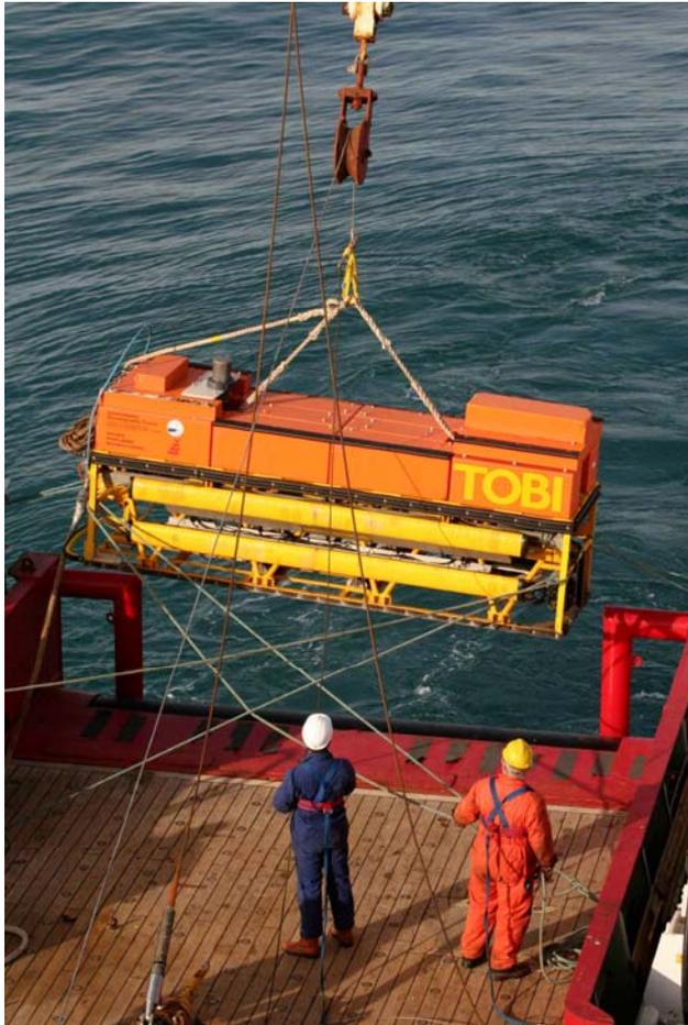
**Fig. 3.1. The deployment of the TOBI vehicle from the stern of the JCR off Svalbard.**
