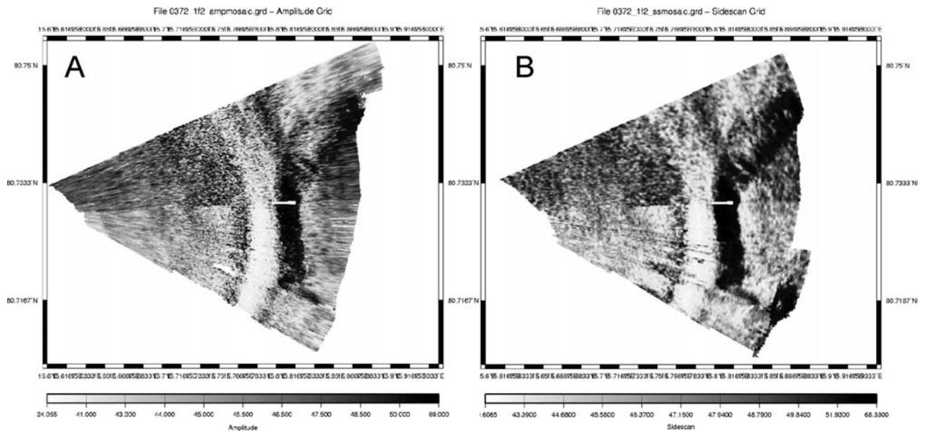
*Fig.6.4. Mosaiced amplitude (A) and side-scan (B) records of the same datasets as presented in Fig.6.2. In addition some low-pass filtering has been applied in order to reduce the random scatter and accentuate BS variability associated with seabed character.*
