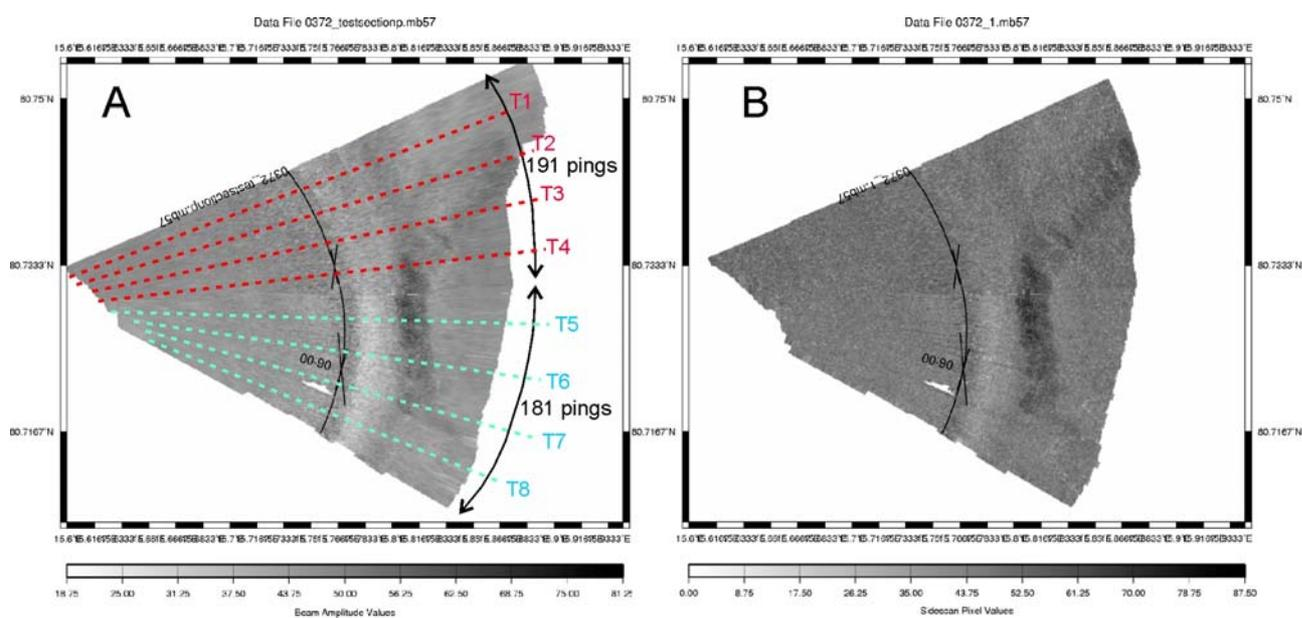
Fig.6.2. Raw amplitude (A) and side-scan (B) records from the same dataset consisting of 372 pings of swath data. Applied processing includes removal of beams with failed bottom
