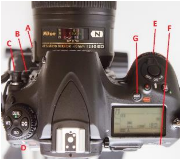
Figure 5.1. Nikon D810 showing location of major controls used in setting up camera for krill photography
