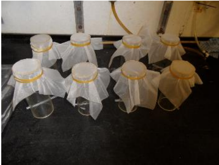
Figure 6.16: Internal plastic tube of gut evacuation bottles with mesh affixed to bottom to allow faecal material to pass out whilst retaining zooplankton
