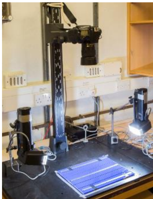
Figure 5.1. Krill photography set-up showing relative positions of flashes and camera to sample board
