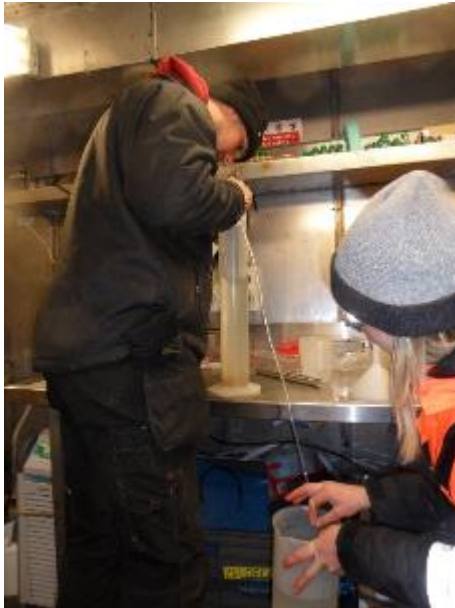
Figure 6.18 Siphoning zooplankton from the cylinder to a second container using a small silicone tube taped to a ruler as a weight and to enable deeper submersion in the cylinder
