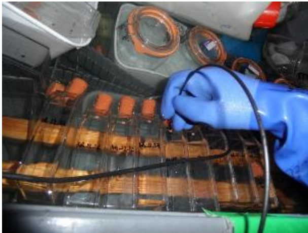
Figure 6.17: Taking \text{O}_2 readings from bottles submerged on a stable platform in the incubator Following this, a second incubation was set up with the contents of the gut evacuation bottles. The same procedure was followed as described above, with controls taken from the remaining sample water passed through a 100 \mu\text{m} mesh sieve.
