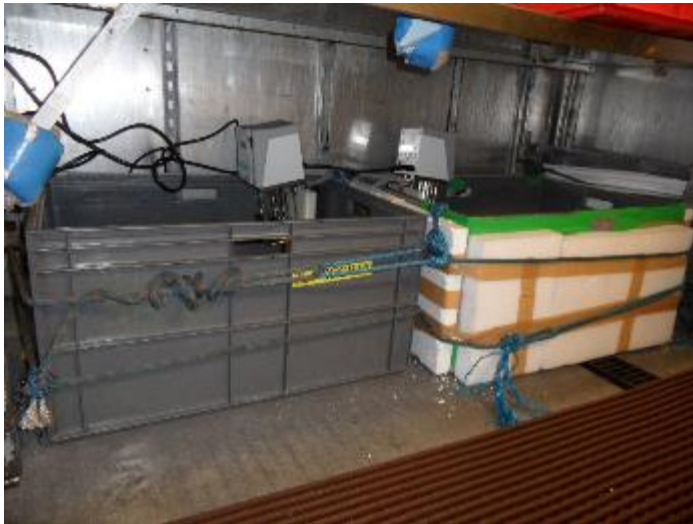
Figure 6.13: Photograph showing the incubator set-up and insulation of the 1\text{ }^{\circ}\text{C} tank (with the chiller unit sitting to the left hand side of the left hand tank)
