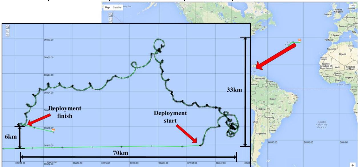
**Figure 6 - Deployed wirewalker mooring surface buoy track**
