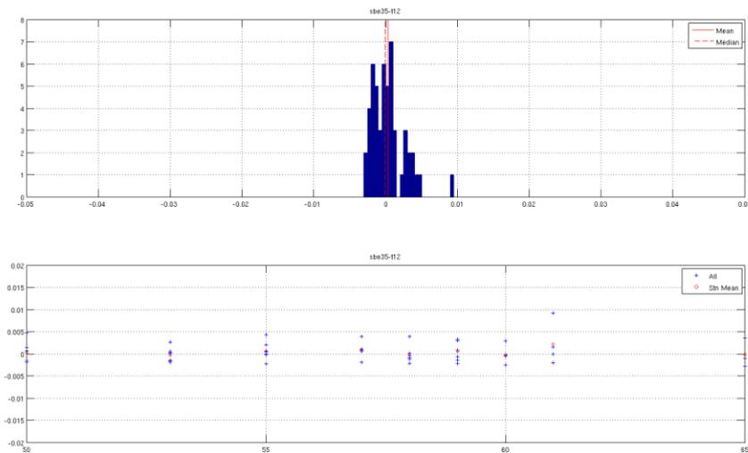
Figure 3: SBE35 minus the second primary temperature sensor after calibration for depths greater than 2000dB. (a) Histogram of temperature difference with the mean and median marked with red lines. (b) Temperature difference by station, with the station mean marked in red.
