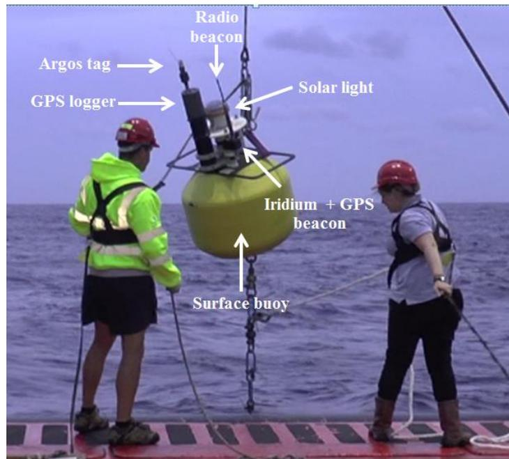
**Figure 3 - Wirewalker mooring surface buoy key features**
