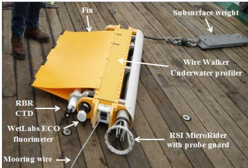
Figure 2 - Wirewalker underwater profiling system key features
