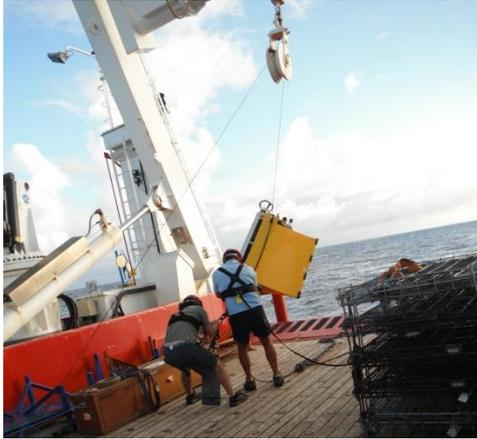
a subsurface weight, wire and wirewalker profiler recovery
