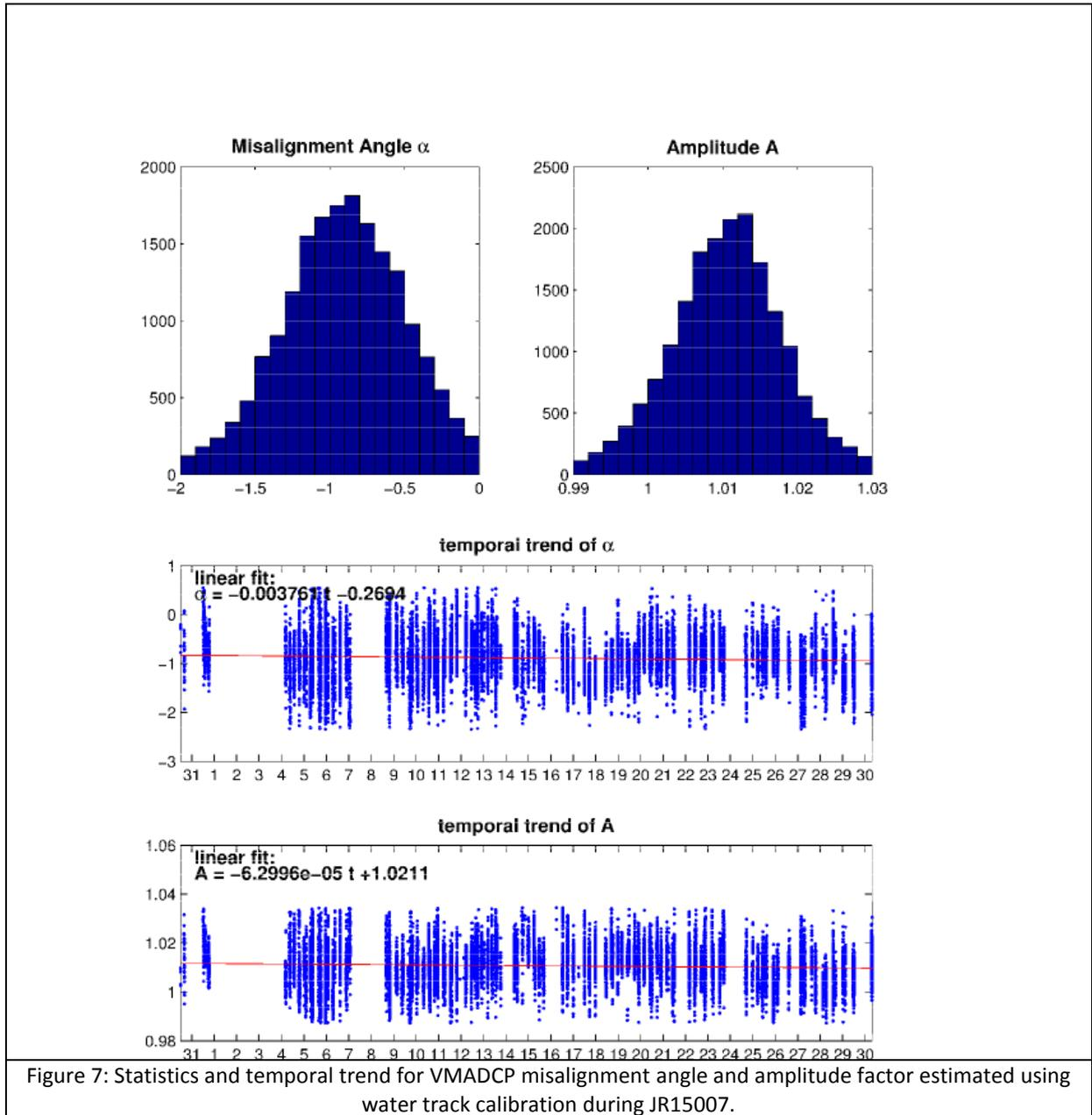
Figure 7: Statistics and temporal trend for VMADCP misalignment angle and amplitude factor estimated using water track calibration during JR15007.
