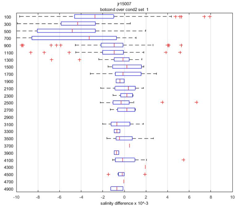
Figure 10: Series of box plots calculated in 200m bins post calibrations for the preferred sensor (secondary). The red lines indicate the median, the blue boxes the interquartile range and the black lines the full range. Data points more than 1.5 times the interquartile range away from q1 or q3 are excluded.
