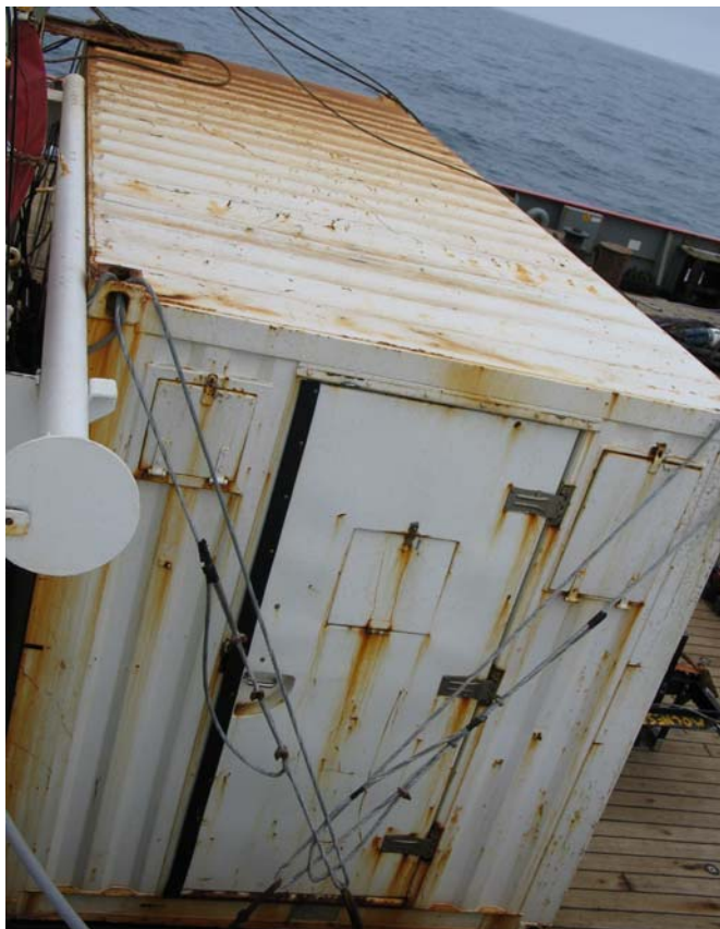
Picture 2, clean container covered in iron spray.
