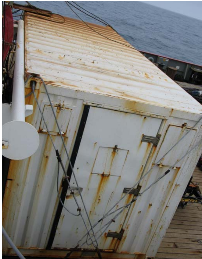
Picture 1, clean container covered in iron spray.
