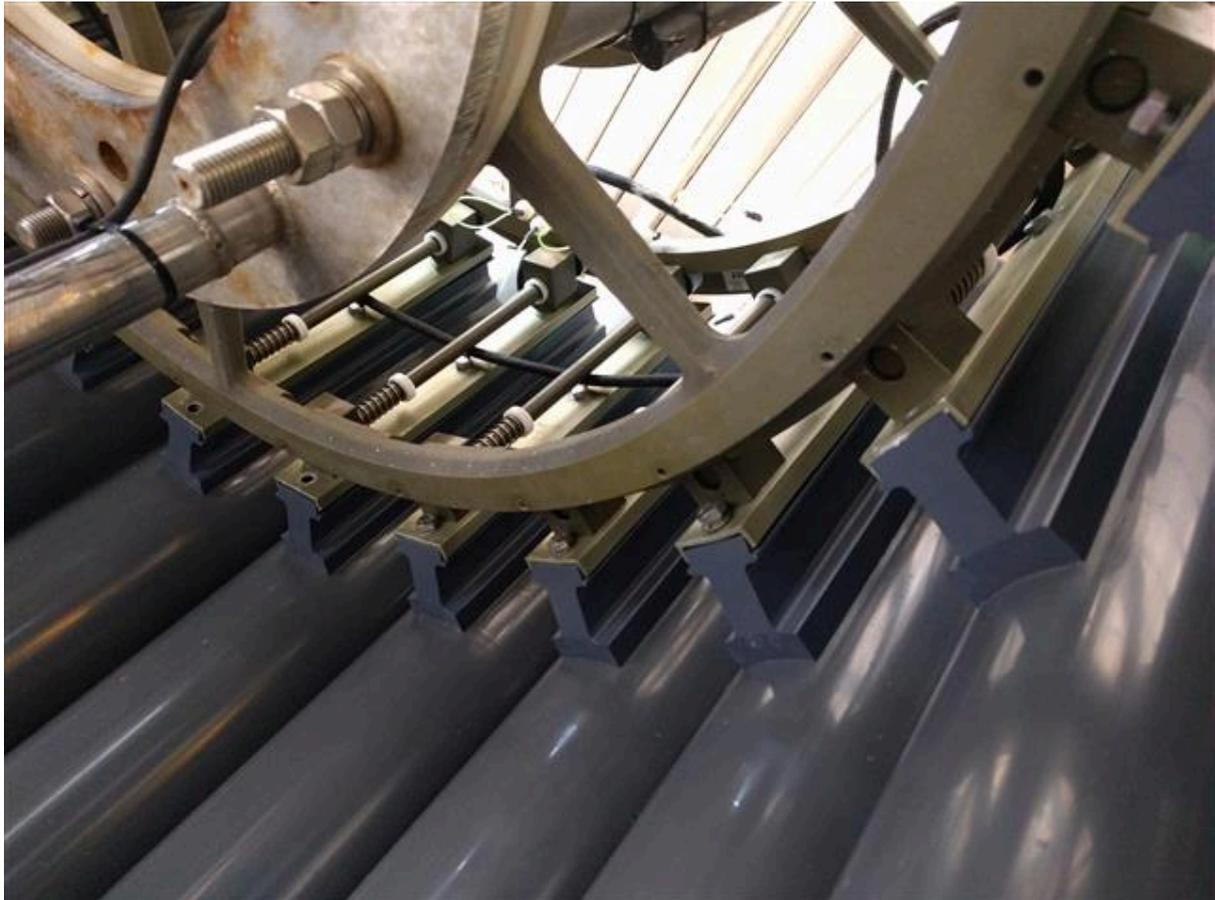
This presents even greater risk of bent brackets, smashed bottles, or lost bottles (specifically as the 'safety rope' used to ensure bottles do not fall off, is threaded through the insides of the brackets.
