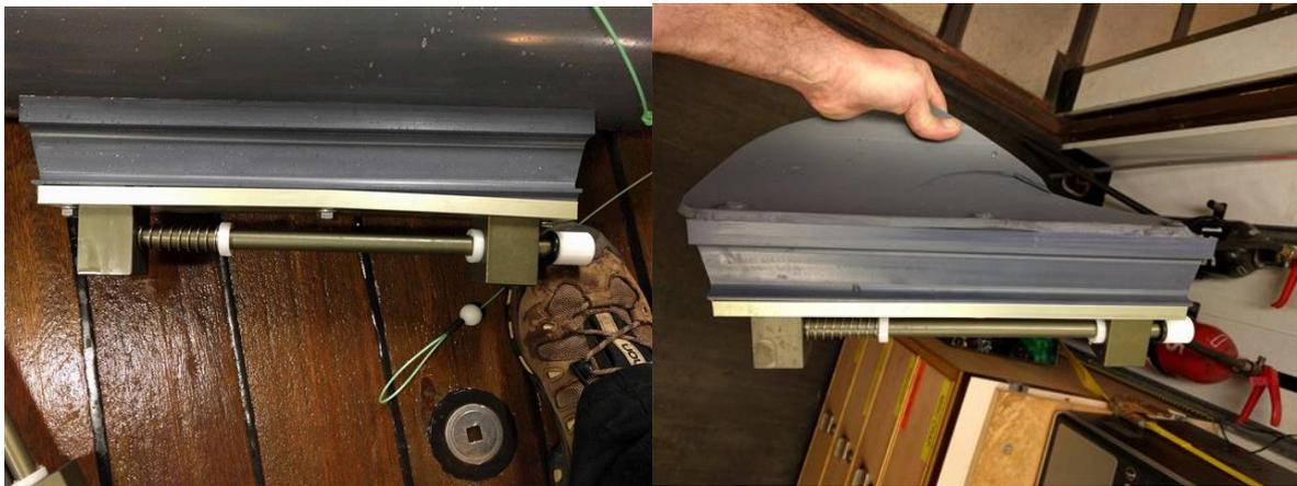
Throughout the cruise there have been bottles failing to seal properly and leaking when recovered. This has been seemingly at random, so addressing the fault for specific bottles has not been possible. Hopefully when new product specific springs are attained, bottle closure will be a bit more constant, and dependable (and there will no longer be issues relating to internal 'spring extension lanyards' snapping.)
