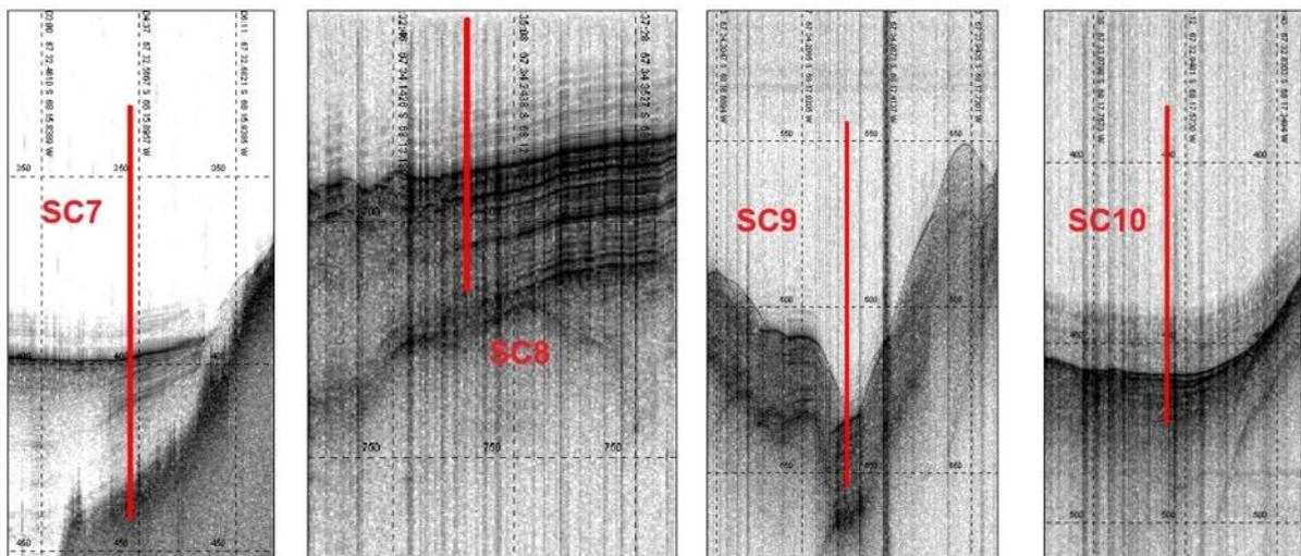
Figure 5.1.17: TOPAS profiles at stations SC7, SC8, SC9 and SC10 from Sheldon Cove, Adelaide Island. Red lines indicate the location on the profile that was targeted by gravity coring, and are summarised further in Table 5.1.7.
