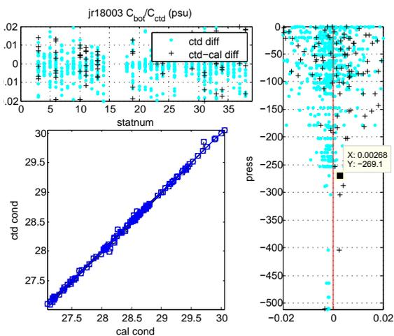
Figure 5.2.4 Comparison of bottle and CTD conductivity sensor 2 (in salinity equivalent units) before (left) and after (right) calibration. The top left panels show residuals as a function of time. Cyan dots are the differences between the two CTD sensors.
