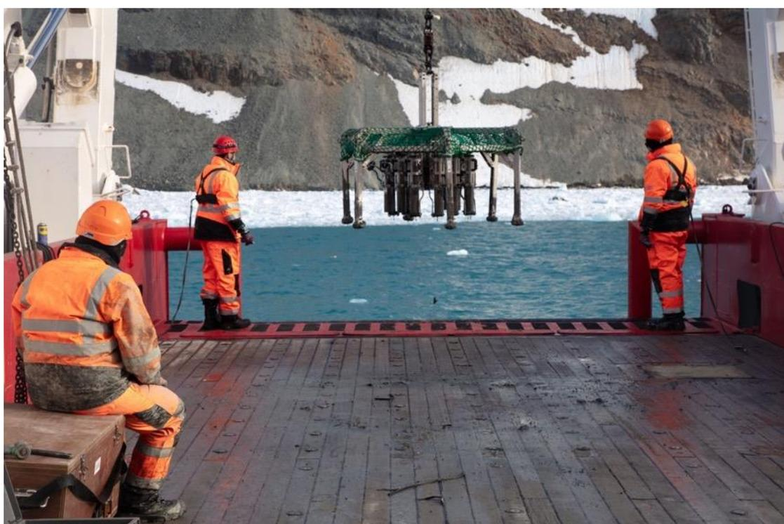
*Figure 5.4.1. Deploying the multicorer from the aft gantry in Marian Cove. Following the failed deployments the multicorer was deployed from the starboard gantry.*
