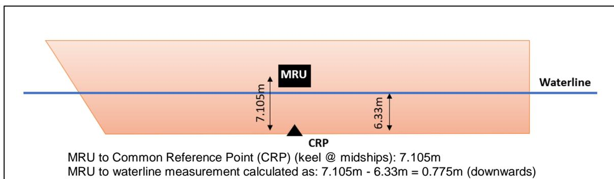
Figure A1.2 MRU to waterline calculation on departure from ECMP.
