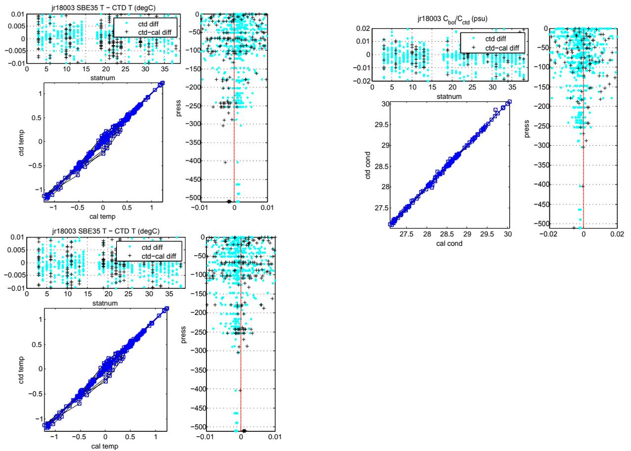
Figure 5.2.3 Comparison of SBE35 and CTD temperature sensor 2 (in salinity equivalent units) before (left) and after (right) calibration. The top left panels show residuals as a function of time. Cyan dots are the differences between the two CTD sensors.
