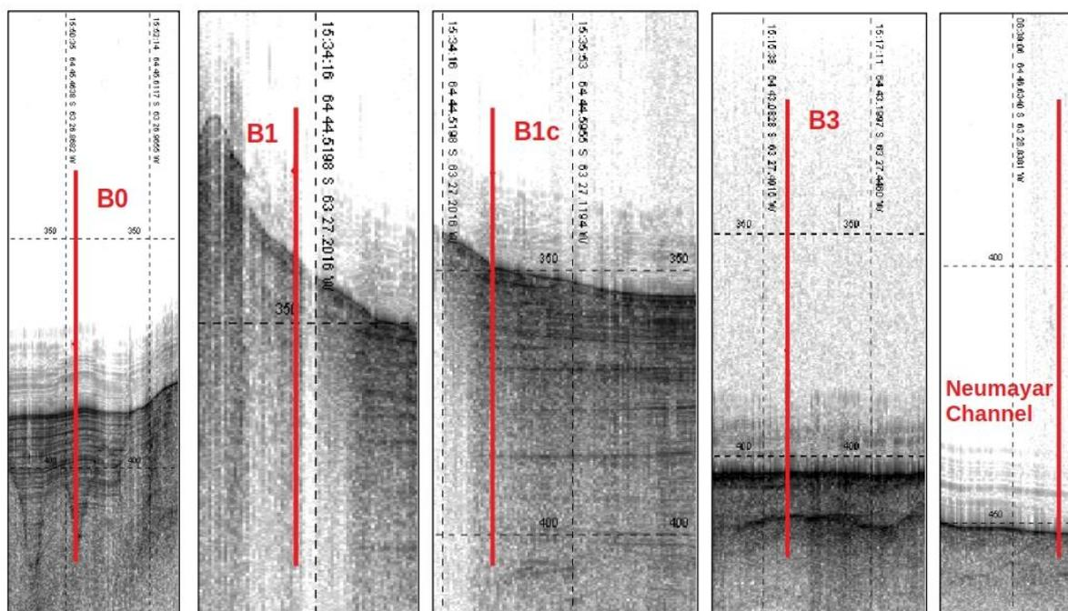
Figure 5.1.16: TOPAS profiles at stations BB0, BB1, BB1c, B3 and Neumayer Channel from Börgen Bay, Anvers Island. Red lines indicate the location on the profile that was targeted by gravity coring, and are summarised further in Table .
