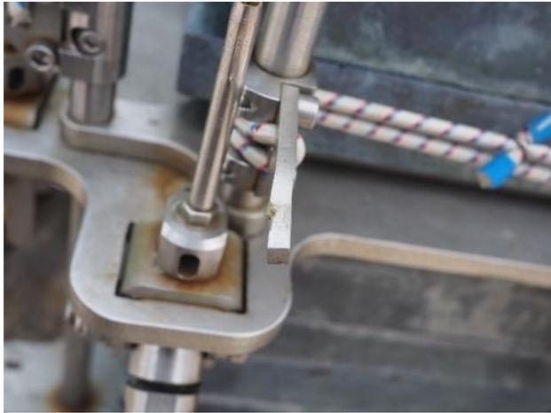
On a few occasions the corer fired but the mechanisms weren't closing with enough force to create a good seal and samples were being lost. The sliding surfaces and spring cylinders were greased, this significantly improved the action of the corer and the retention of samples in core tubes. It also made the cores easier to remove. If the corer remains unmodified we need to take spray grease (Rocol Biogen) on its next cruise.
