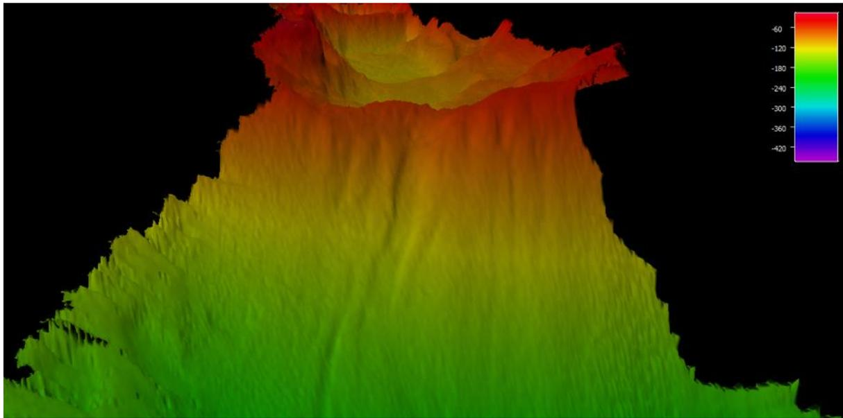
*Figure 5.1.6 Distal sill feature at Marian Cove. 3D view looking North East. Scour or channel feature is evident and similar to that observed in Børgen Bay.*
