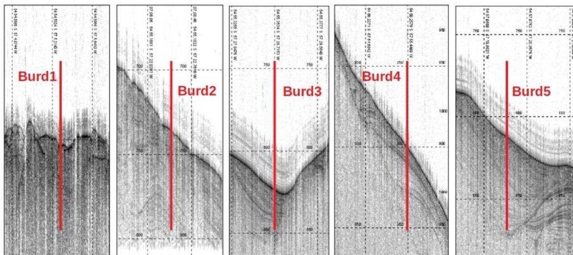
Figure 5.1.14: TOPAS profiles identifying potential targets for gravity coring at Burdwood Bank. These sites are summarised further in Table 4.
