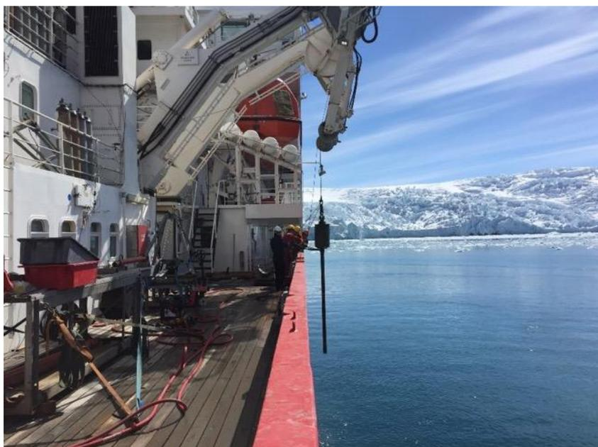
Figure 5.4.4 Once overboard, the gravity corer was lowered by one winch and disconnected, before being deployed by the second winch. The process was carried out in reverse once the sediment was collected.
