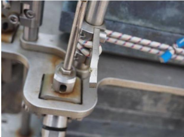
On a few occasions the corer fired but the mechanisms were not closing with enough force to create a good seal and samples were being lost. The sliding surfaces and spring cylinders were greased and this seemed to make a significant improvement. It also made the cores easier to remove. If the corer remains unmodified we need to take spray grease on its next cruise.
