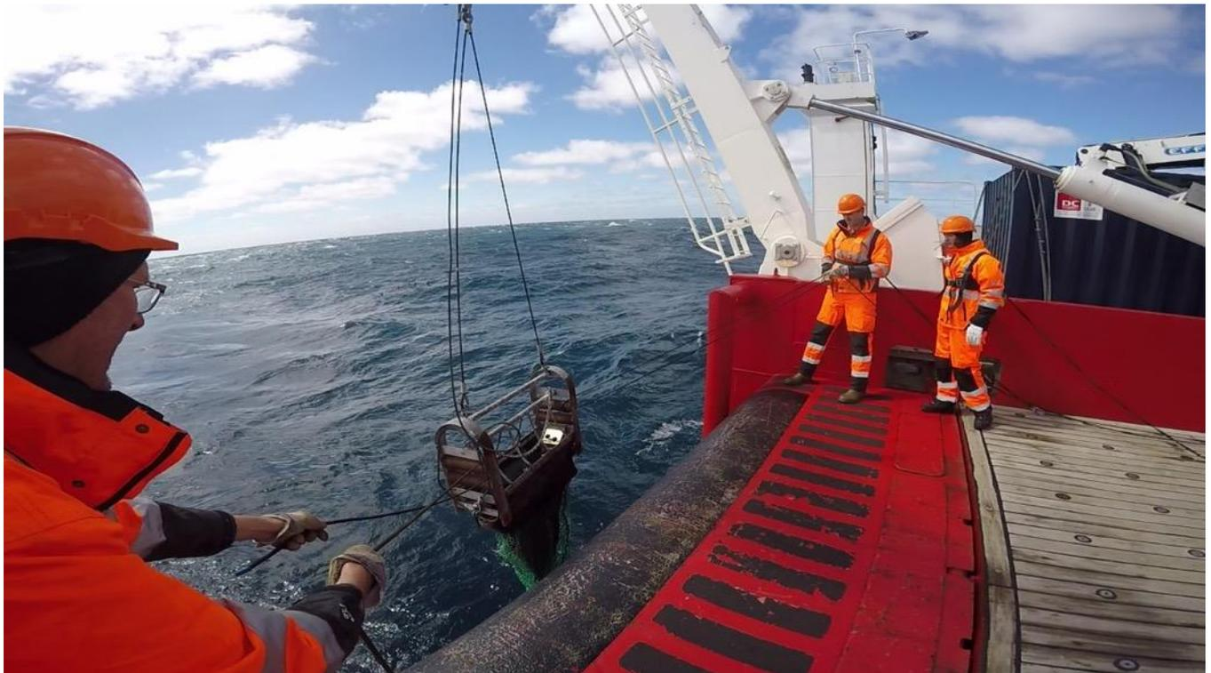
Figure 5.5.4 miniAGT being recovered. Fire hoses were used to wash out mud before landing the trawl on the deck.
