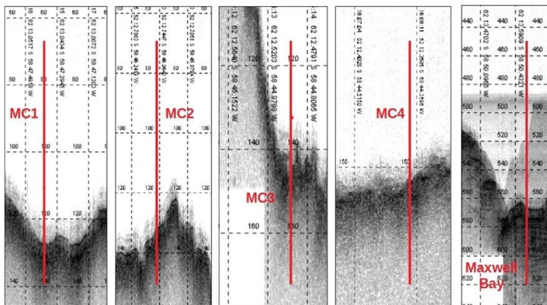
Figure 5.1.15: TOPAS profiles at stations MC1, MC2, MC3, MC4 and Maxwell Bay from Marian Cove, King George Island. Red lines indicate the location on the profile that was targeted by gravity coring and are summarised further in Table .
