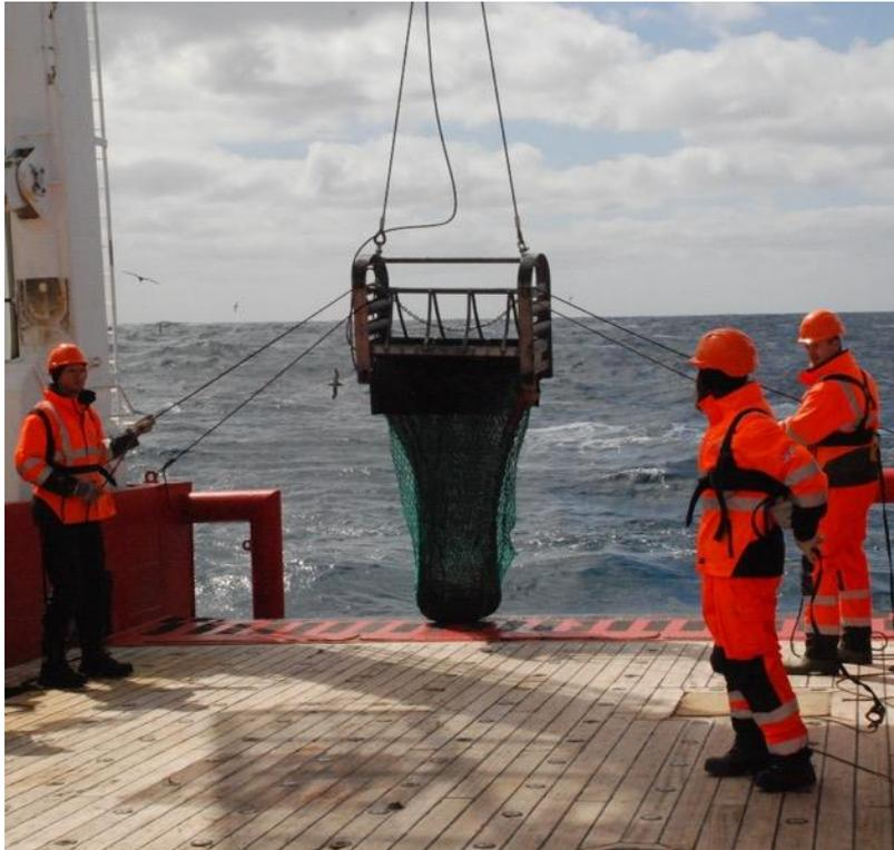
Figure 5.5.2 Agassiz Trawl being returned to deck while on the Burdwood Bank. Picture courtesy of S. Jenkins.
