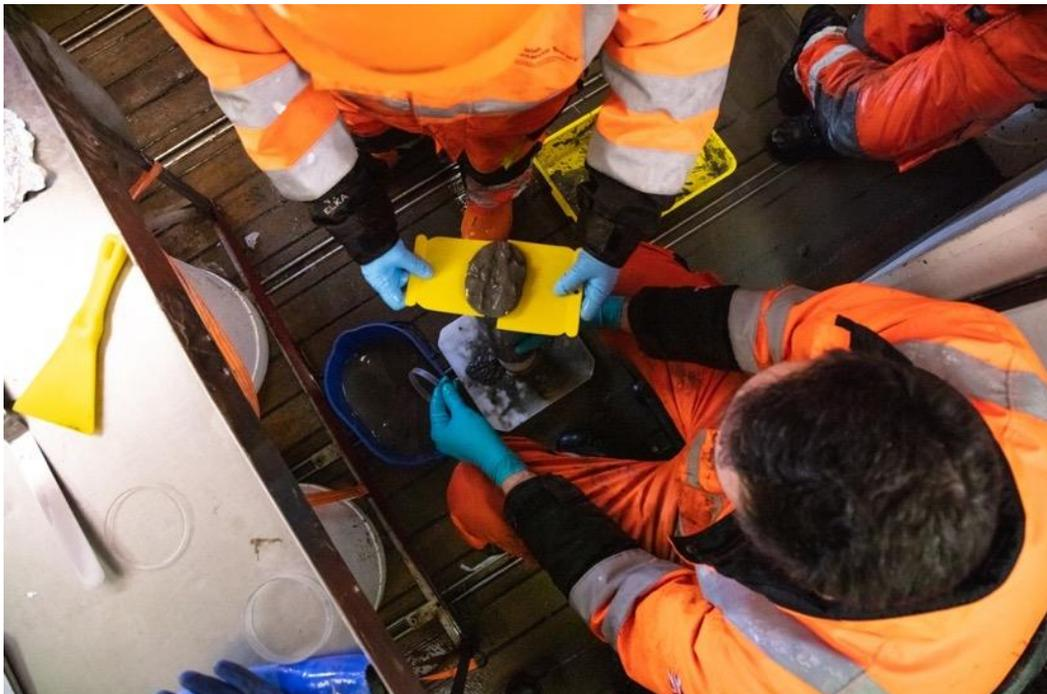
*Figure 5.4.2 Using plastic slicer to subsample multicores.*
