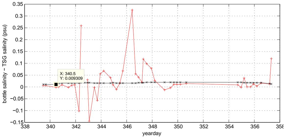
Figure 5.2.6: TSG and bottle salinities before calibration (top), with differences (bottom); the smoothed black function was used to calibrate the TSG record.
