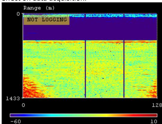
Figure A1.1 SIS Stave display showing 2 receive staves with reduced signal level (vertical blue lines)
