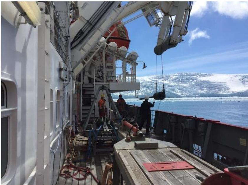
*Figure 5.4.3 The gravity corer was initially raised from its basket with both side winches whilst being held steady by two crew members.*
