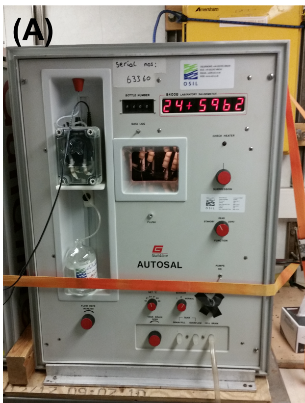
Figure 5: Salinometer Guildline Autosal 8400B s/n 63360 (a) and IAPSO standard seawater – batch P160 (b) used during the cruise JR18004.
