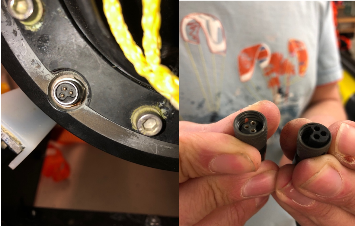
Figure 28: Rubber from the altimeter cable fused with rubber in the bulkhead socket (left). Right: A comparison between the end of the broken altimeter's cable (left; Unit 330's), and a working altimeter (right; Unit 352's).
