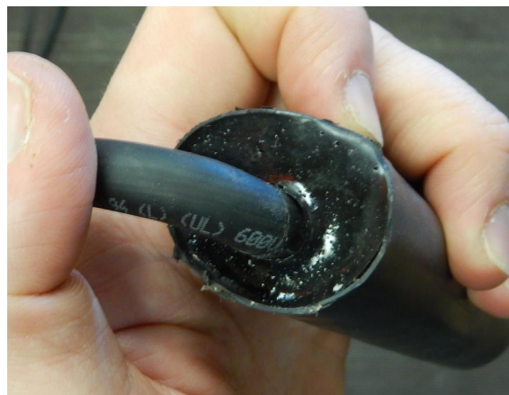
Figure 49: Conducting wire potting damage.
