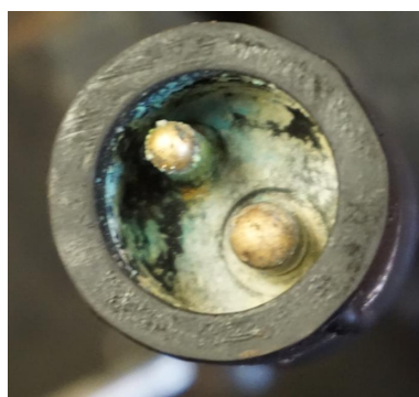
Figure 53: LADCP Cable Corrosion
