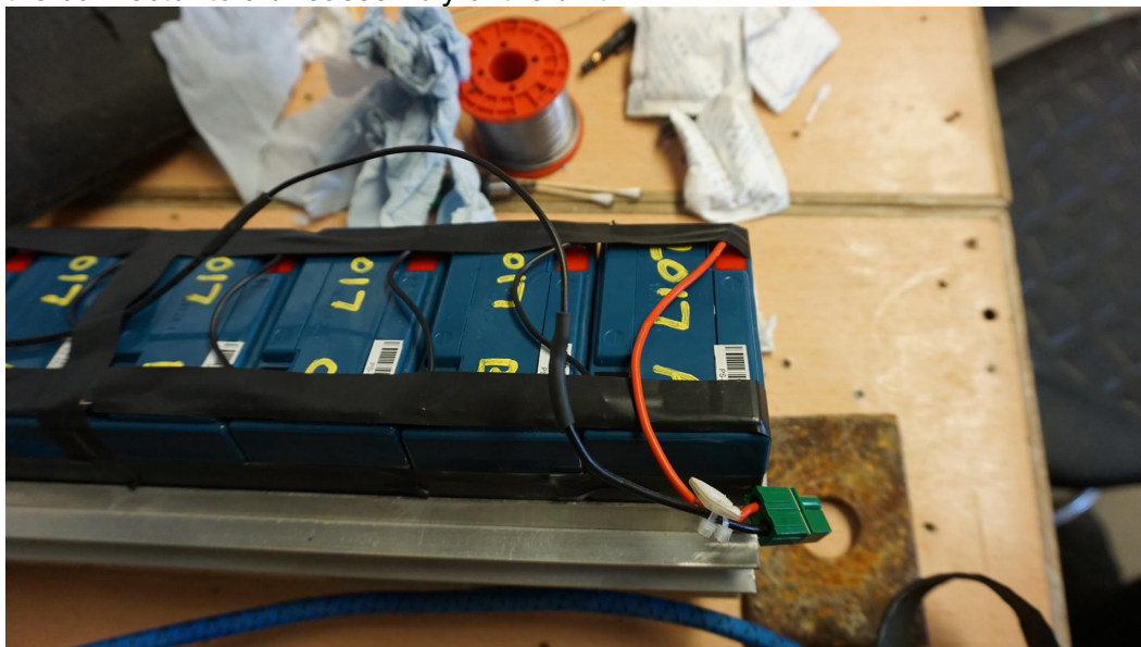
Figure 55: LADCP battery housing wiring after modification
