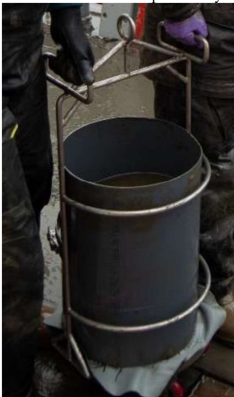
Figure 6.1b2 Transport of a core using the carrying frame and rolling platform across the deck
