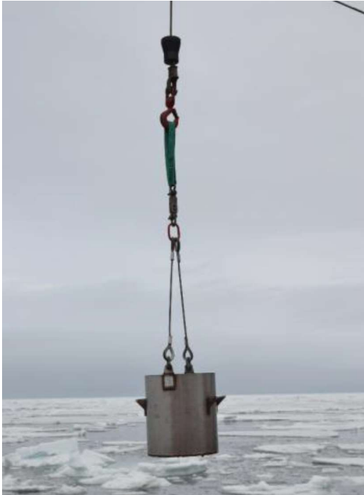
Figure 4.6b – Collection of sea ice using NMF ice catcher attached to the JCR’s hydraulic crane (Photo A.Reed).
