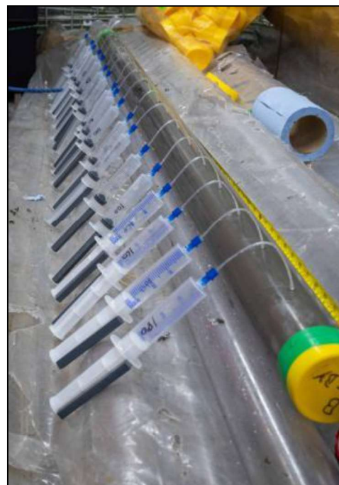
Figure 5.2a: Pore water extraction with Rhizone samplers and 30 mL syringes in the cold room. Photo: J. Faust
