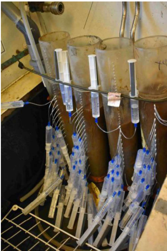
Figure 5.1b3: Pore water extraction with Rhizone samplers and 30 mL syringes in the sink of the wet lab. Photo: M. Zindorf
