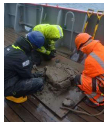
Figure 7.2b Image showing the manual inspection of the sample for infauna >1cm.
