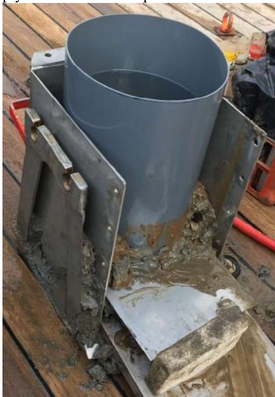
Figure 6.1b1 Removal of one of the sediment cores from the box corer box, while keeping the sediment matrix and overlying water intact. The box cores with removable side panels were in part funded through the Charles Boyden Award and allowed the sampling process to be faster and less labour intensive than it would otherwise have been.
