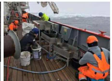
Figure 7.2c2 Image showing the sieve table set-up and the staged sieves.
