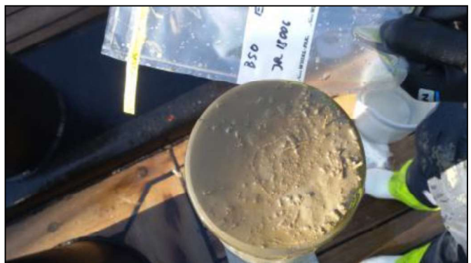
Figure 5.1b2: Intact sediment surface with benthic fauna in a Megacorer tube. Photo: M. Zindorf
