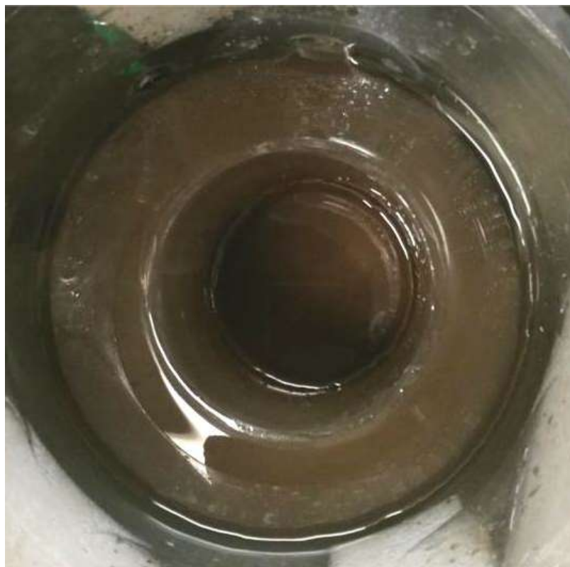
Figure 6.1b3 View from the top of the flume immediately after the end of the flume run, before syringe cores are taken. The flow channel around the outside exhibits elevated levels of suspended matter while the central section is unaffected by the resuspension experiment and can be used as a control sampling area.
