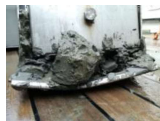
Figure 7.2c3 Image showing a rock and the damage it caused to the scoop.
