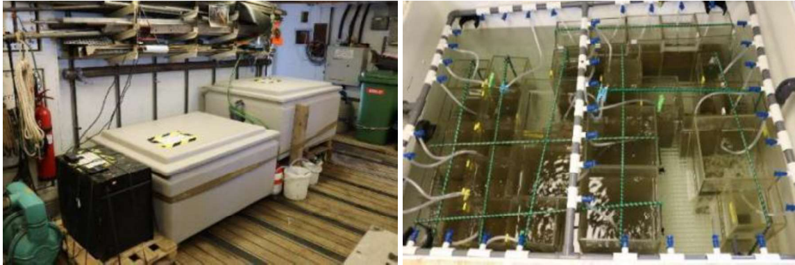
Figure 7.4b Temperature controlled water baths and mesocosms containing sieved sediment and benthic invertebrates.
