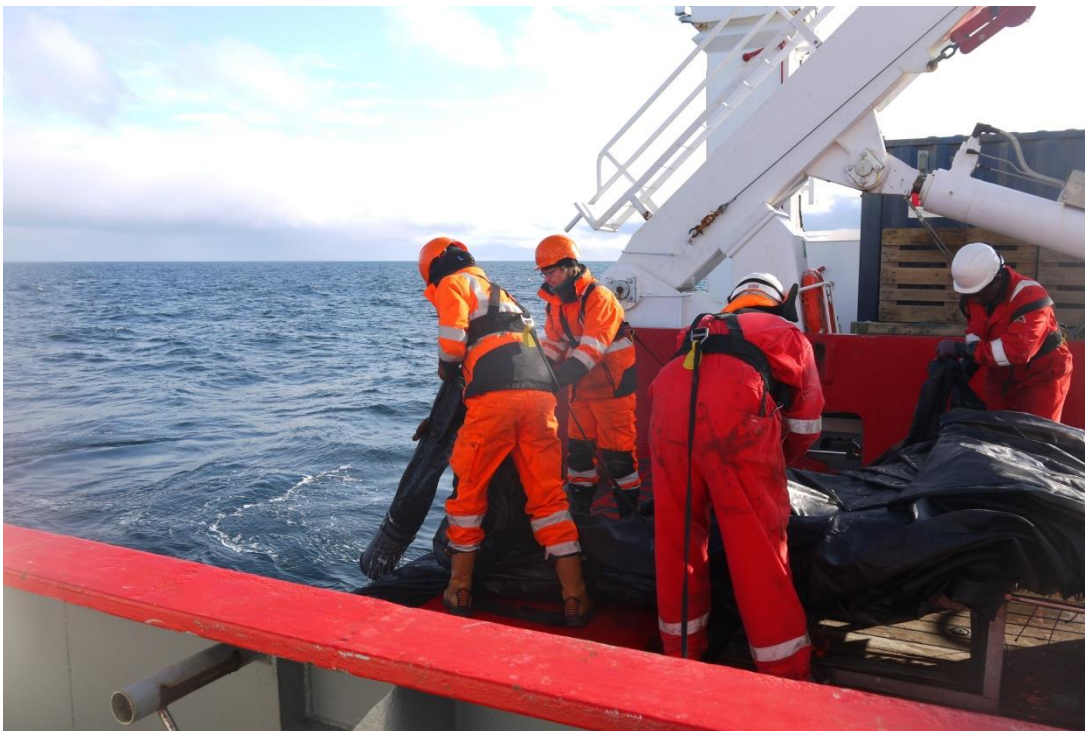
Fig. 5.2. Recovery of MOCNESS - codends being lifted over the stern ramp
