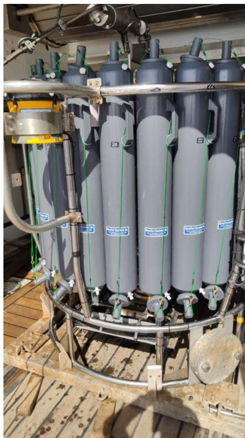
Figure 1: CTD 20L niskin lanyard problem.
