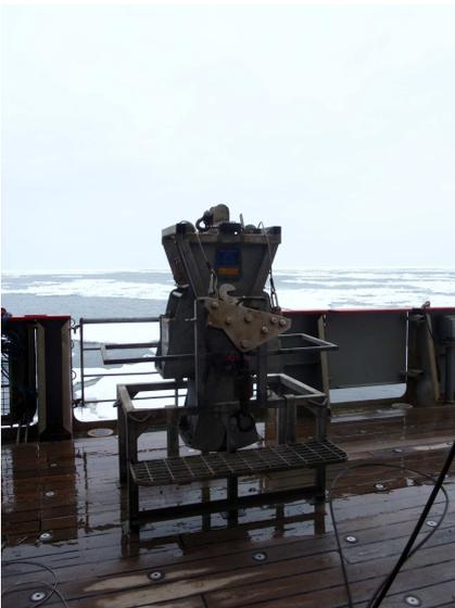
**Figure 7** The box corer.
