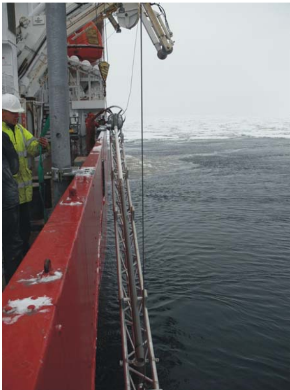
Figure. 8. Recovery of the BAS gravity corer on JR244. (Photo: R. Larter)
