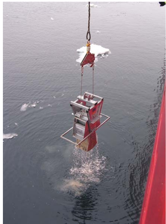
Figure. 9. Recovery of the BAS box corer. (Photo: unknown)
