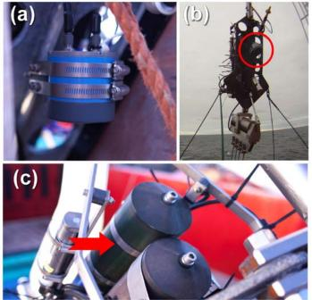
Figure 3 - (a) The echo sounder is shown mounted beneath the RMT cross. (b) The echo sounder's position (circled) is visible during net deployment and recovery. (c) The battery pack (highlighted) is shown strapped above the RMT electronics bottle.
