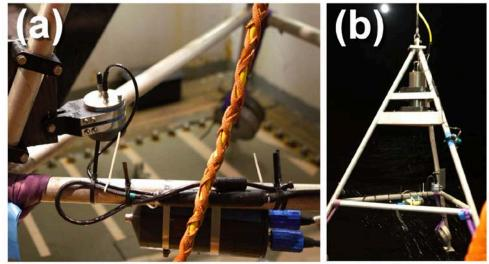
Figure 5 - (a) Echo sounder system mounted on the frame of the SUCS camera. (b) SUCS camera during recovery showing the setup of the echo sounder system.
