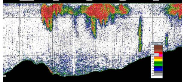
Figure 8. Acoustic data collected by the EK60 during event 95, showing krill swarms in the upper 60 m.
