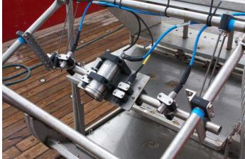
Figure 14 - Front of EBS with Camera (centre) Lasers (each side of camera) and Lights (on the outsides)
