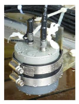
Figure 1 - ES853 echo sounder with serial cable connection.
