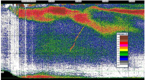
Figure 26 - EK60 120kHz showing krill following SUCS downcast
