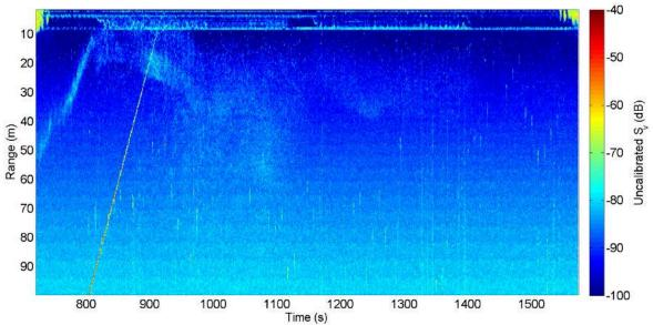
Figure 7. Uncalibrated Sv from Event 38, showing the interval when the echosounder was submerged.
