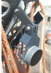
Figure 4 - The echo sounder is shown in a revised position, occupying the space previously held by the flow meter.
