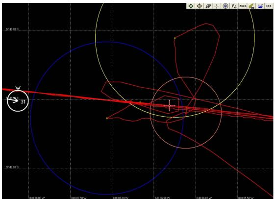
Figure 17 - P3 Mooring location: Calculated mooring position by triangulation.
