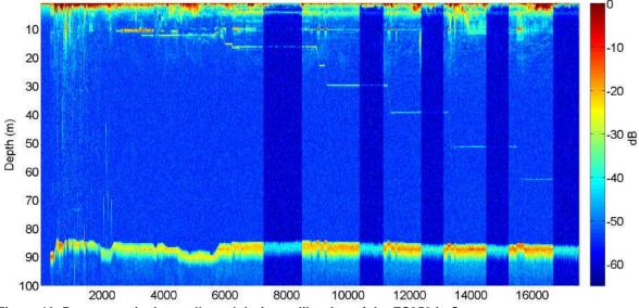
Figure 10. Raw acoustic data collected during calibration of the ES853 in Stromness.
