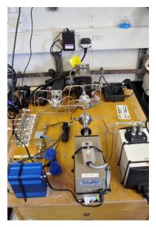
Figure 29 - Valve board, connecting the  $N_2O/CO$  analyser to the equilibrator headspace, marine air line and reference gases.
