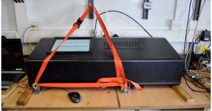
Figure 28 - N<sub>2</sub>O/CO analyser, Los Gatos Research, Inc.
