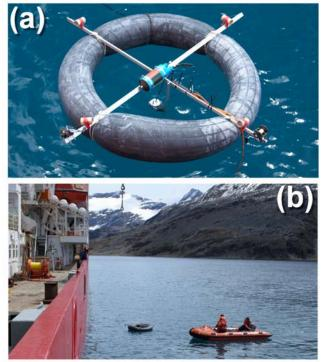
Figure 6 - (a) The doughnut platform with the support cross, fishing lines and echo sounder system. (b) The JCR, doughnut platform and support boat in Stromness Bay.
