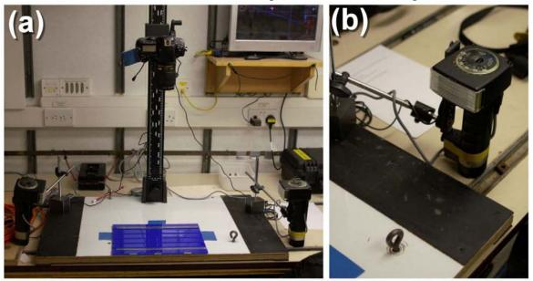
Figure 22. (a) Krill photography setup with magnetically mounted flash guns, camera stand and krill board. (b)
