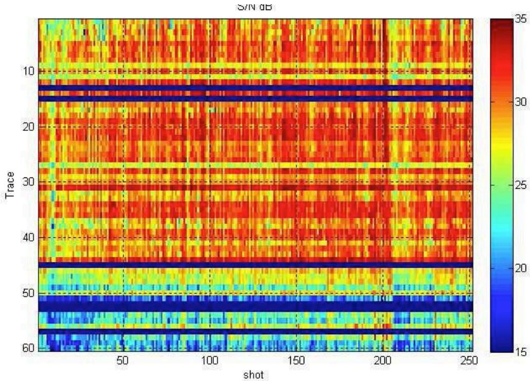
**Figure 10.12: Signal to noise ratio computed from profile JCR269-19 Shot 500 to 750 – Filter 25-350 Hz**
