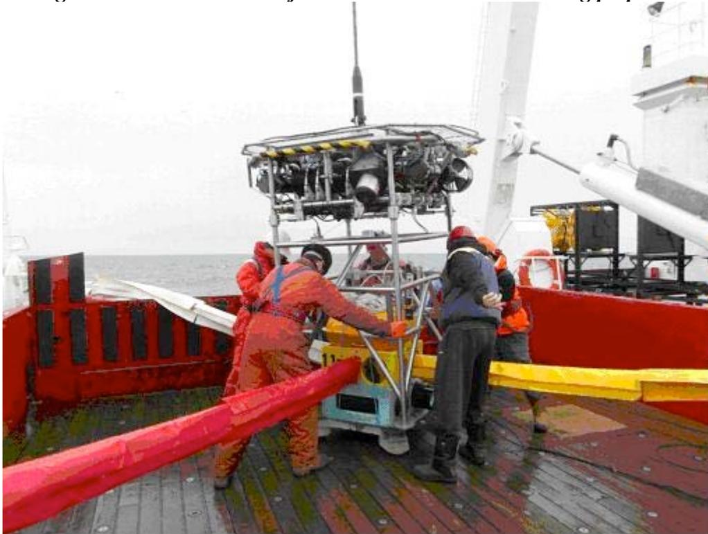
*Figure 11.17: Securing the EM Instrument to HyBIS*
