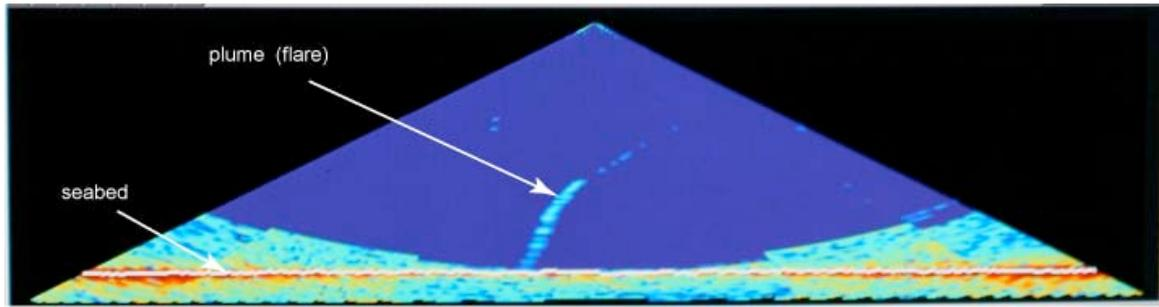
**Figure 7.1:** Screen image from the EM 122 of acoustic flare emanating from the seabed at a pockmark on the Vestnesa Ridge. Water depth approx 1200 m.
