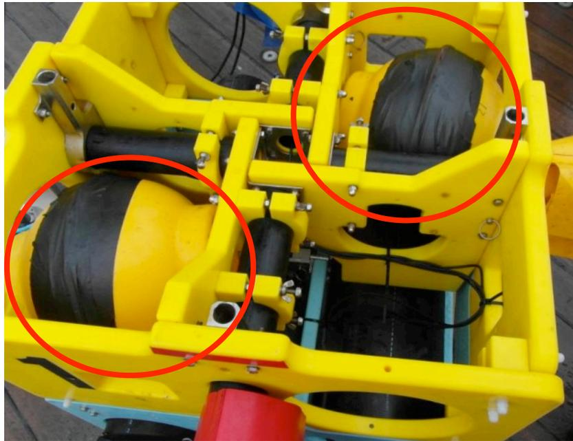
*Figure 11.3: Floats mounted inside the EM Chassis*
