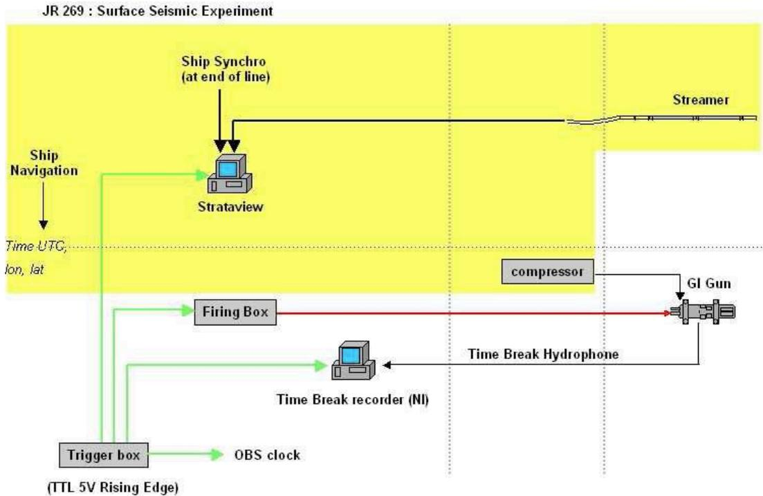
*Figure 10.1 : Surface seismic equipment operated during the JR269 cruise*
