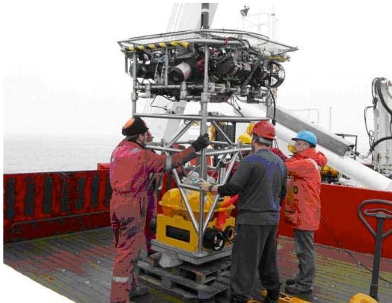
**Figure 11.7: Securing the OBS to HyBIS**
