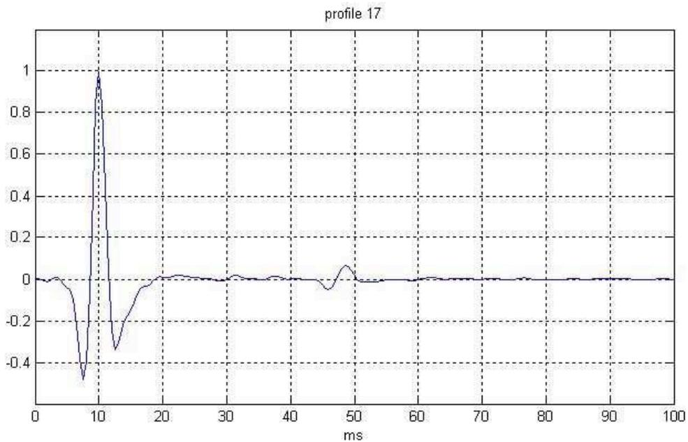
*Figure 10.15: Mean seismic signature from the sea floor (profile 17). The secondary arrival corresponds to the injector blast, 40 ms delayed from the generator blast; relative amplitude is 6.5 % of the primary blast.*
