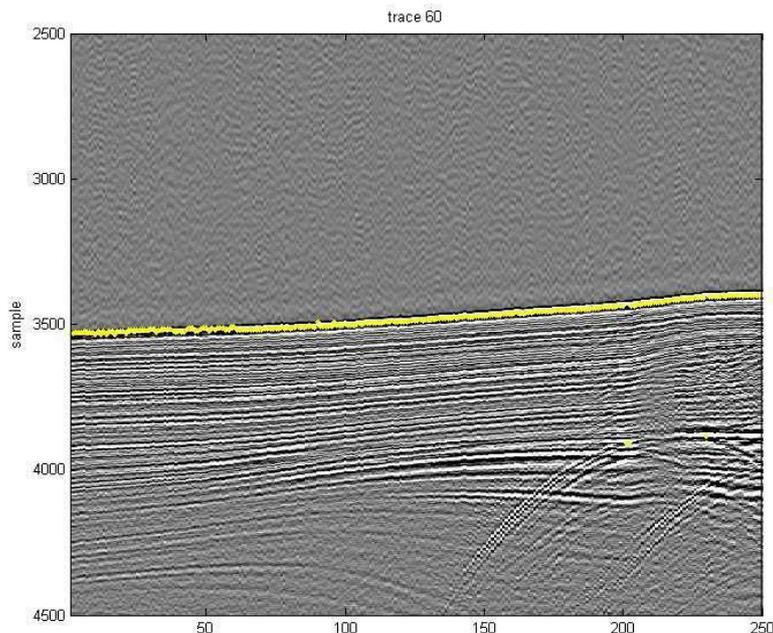
**Figure 10.11: Example of CRG (#60) – automatic picking of the sea floor (yellow points) to define start of the signal window (400 samples long) – filter 25-350 Hz. Mean signal ratio for this trace is 21.5 dB**
