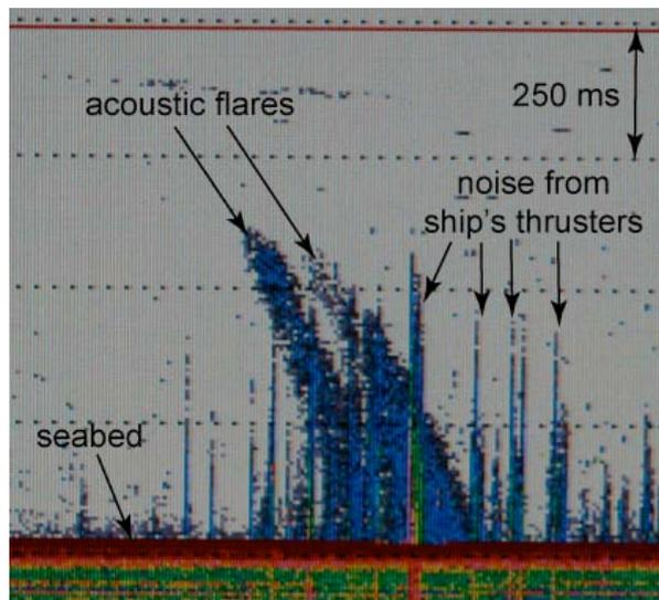
**Figure 7.6:** EK60 image at 38 kHz of two acoustic flares from pockmark on the Vestnesa Ridge. The flares lean to the left because of the effect of the current. Noise bursts from the ship's thrusters are vertical and extend beneath the seabed.
