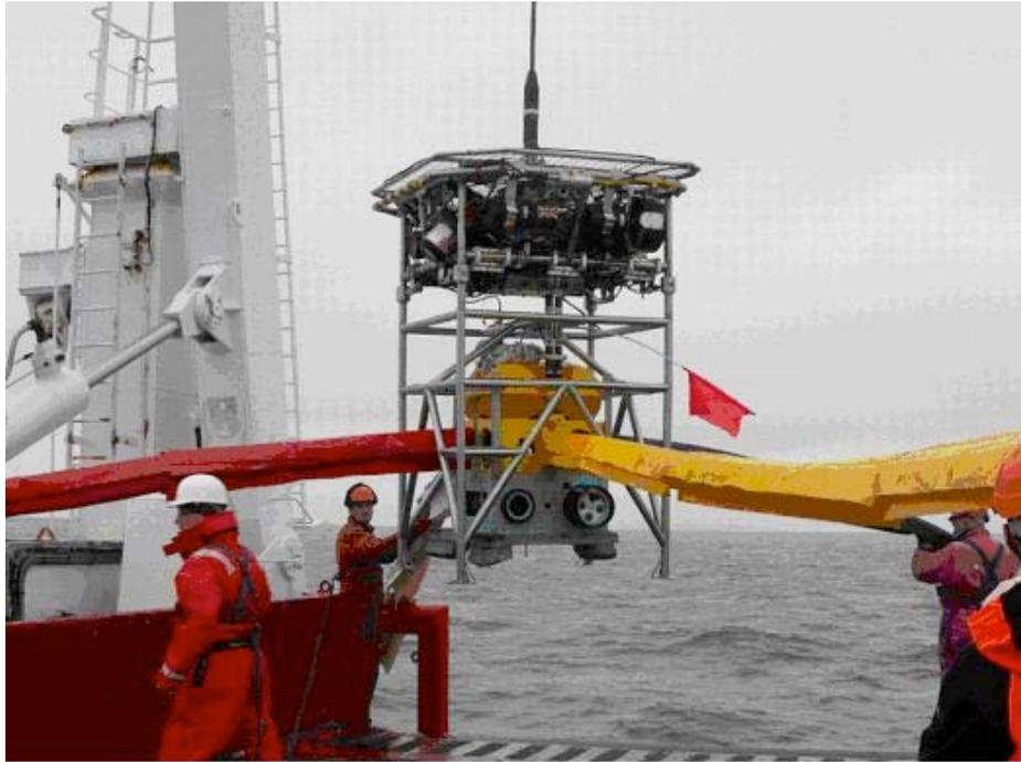
*Figure 11.18: Deploying EM Instrument with HyBIS*
