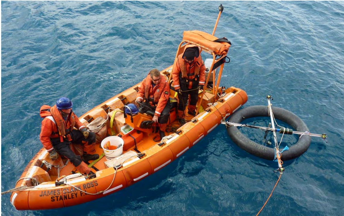
Figure 10. Deployment of the inflatable platform, suspending the echo sounder in the water.
