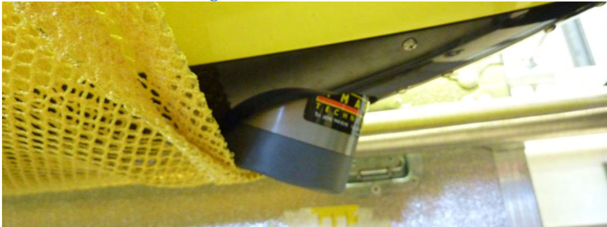
Figure 11. ES853 unit 5706 integrated into the ogive fairing of Seaglider 565
