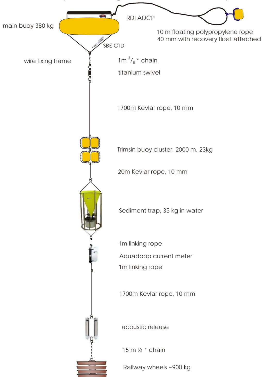
**Figure 27: Schematic illustration of the mooring sediment trap.**
