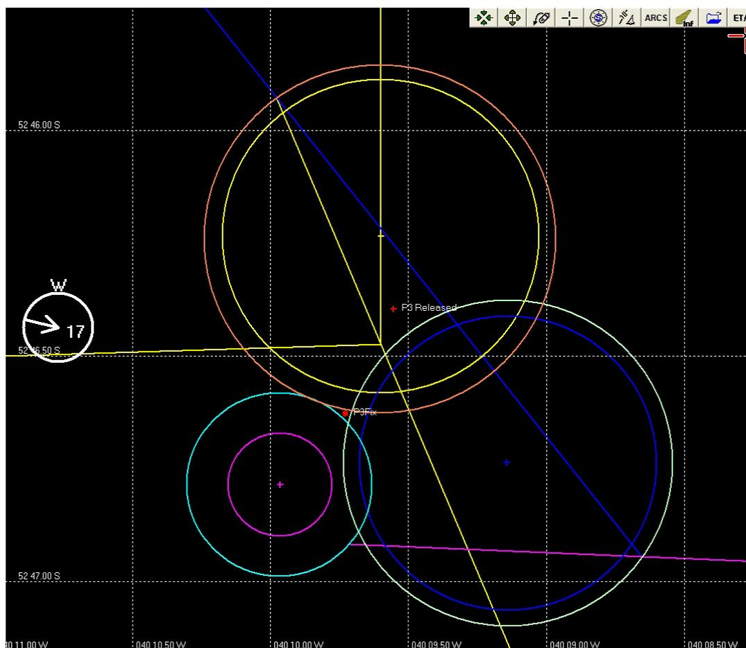
Figure 26: Microplot screenshot of mooring triangulation.
