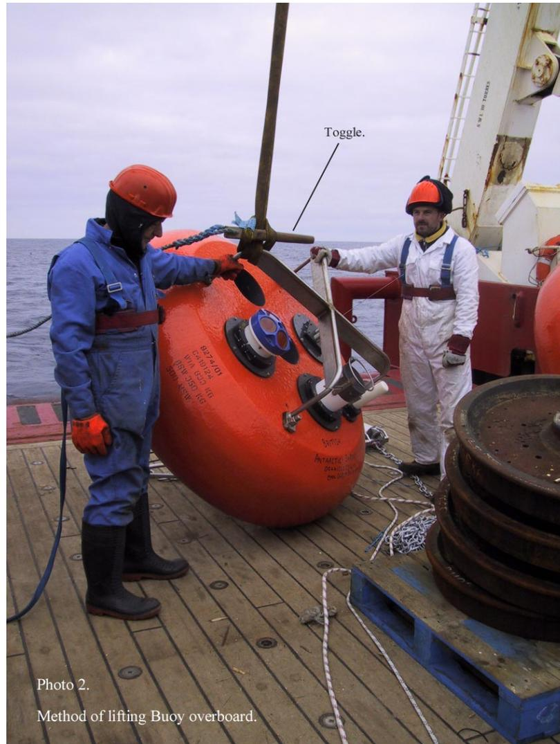
A HEAVING LINE WAS ALSO BE ATTACHED TO THE SHACKLE TO PREVENT THE HEAVY WIRE CRASHING TO THE DECK AS SOON AS THE WEIGHT OF THE BUOY IS RELEASED. Once the buoy was floating the toggle was pulled out, (not all that easy because of the weight of the Gilson wire maintains a tension.)
