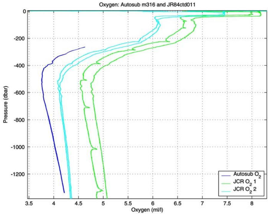
**Figure 37:** Comparison of Autosub and ship’s CTD dissolved oxygen values.
