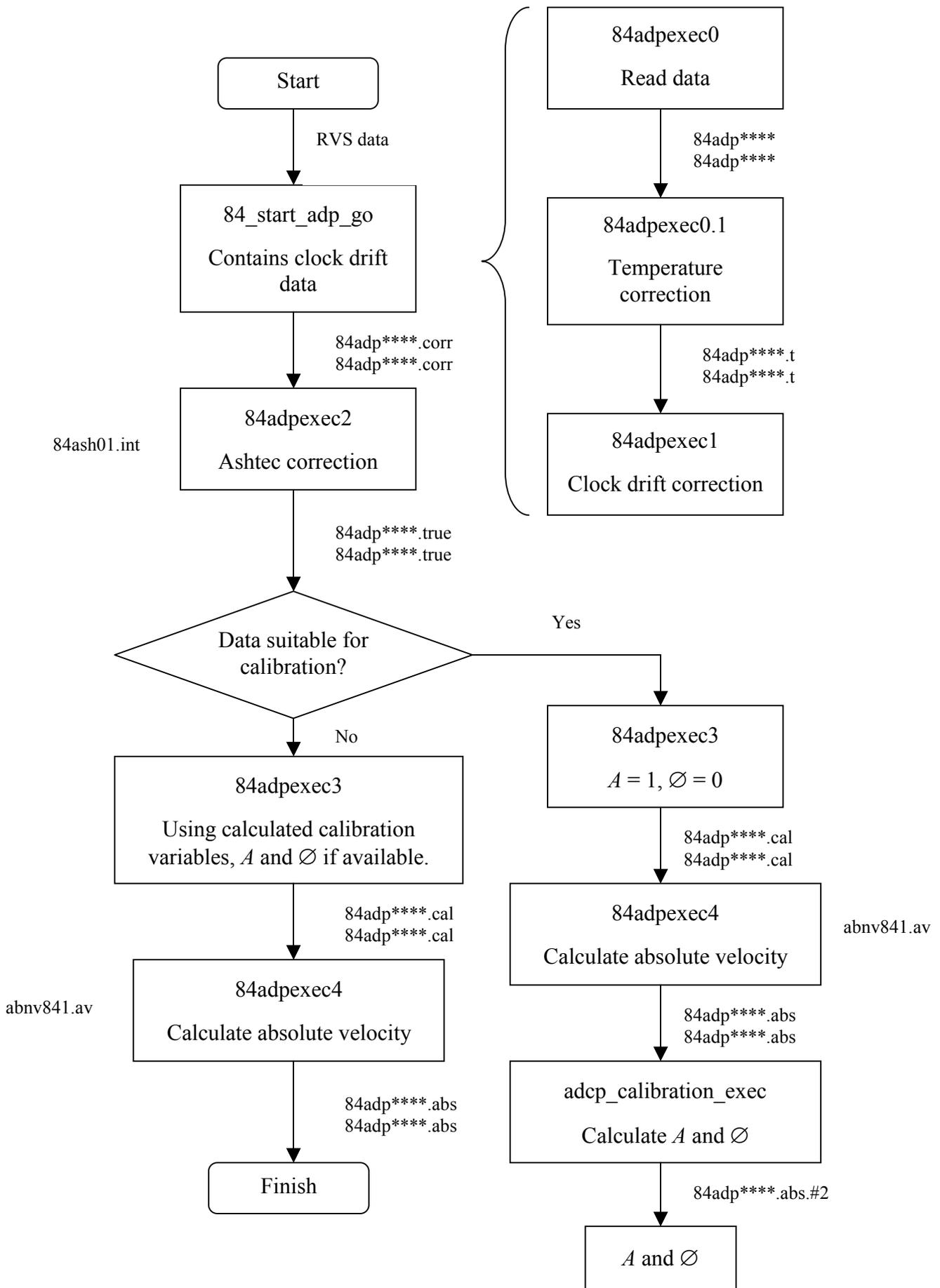
Figure 14: ADCP Processing Flow-Chart
