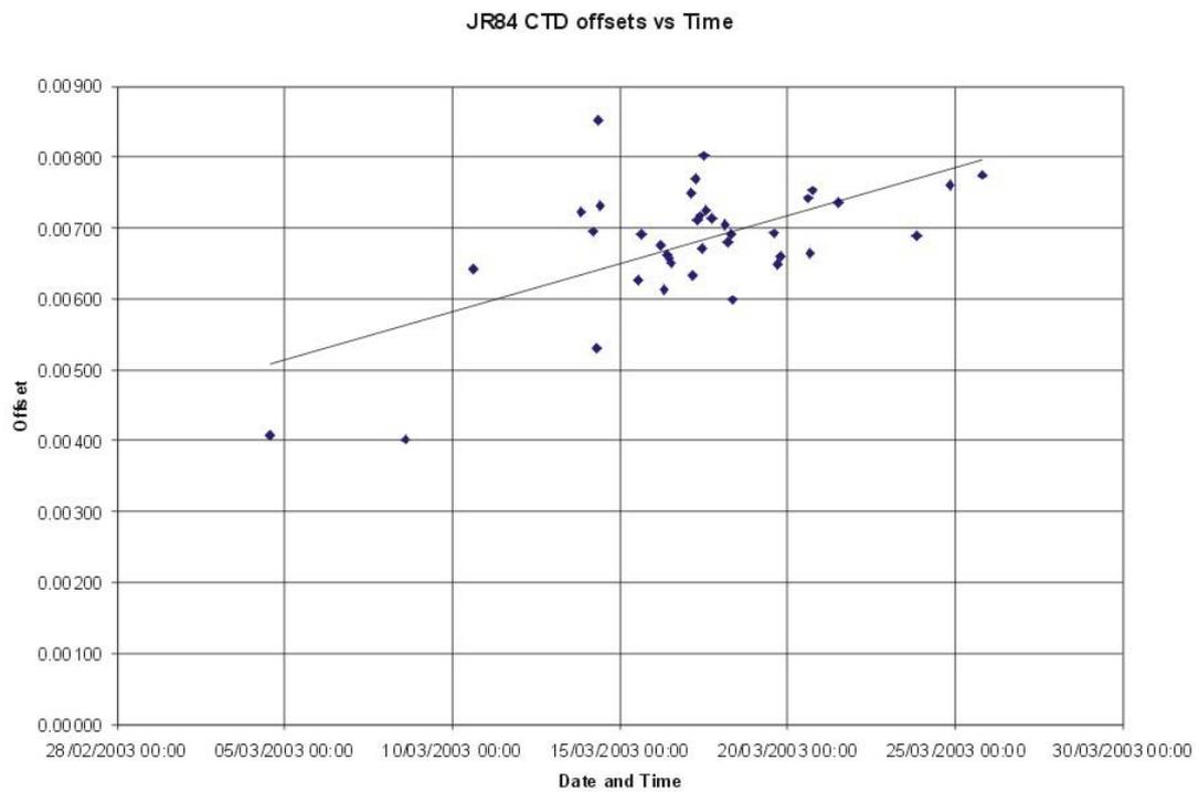
**Figure 11:** Conductivity offsets versus time for JR84.
