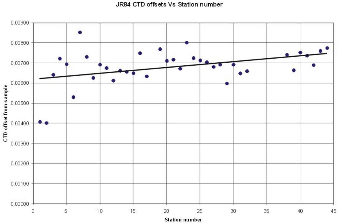
**Figure 10:** Conductivity offsets versus station number for JR84.
