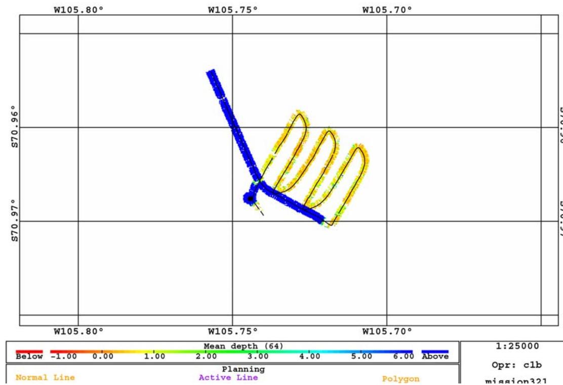
**Figure 34:** Results of Raw Multibeam Sonar Analysis of Ice Draft for Autosub Mission 321 for Survey Area
