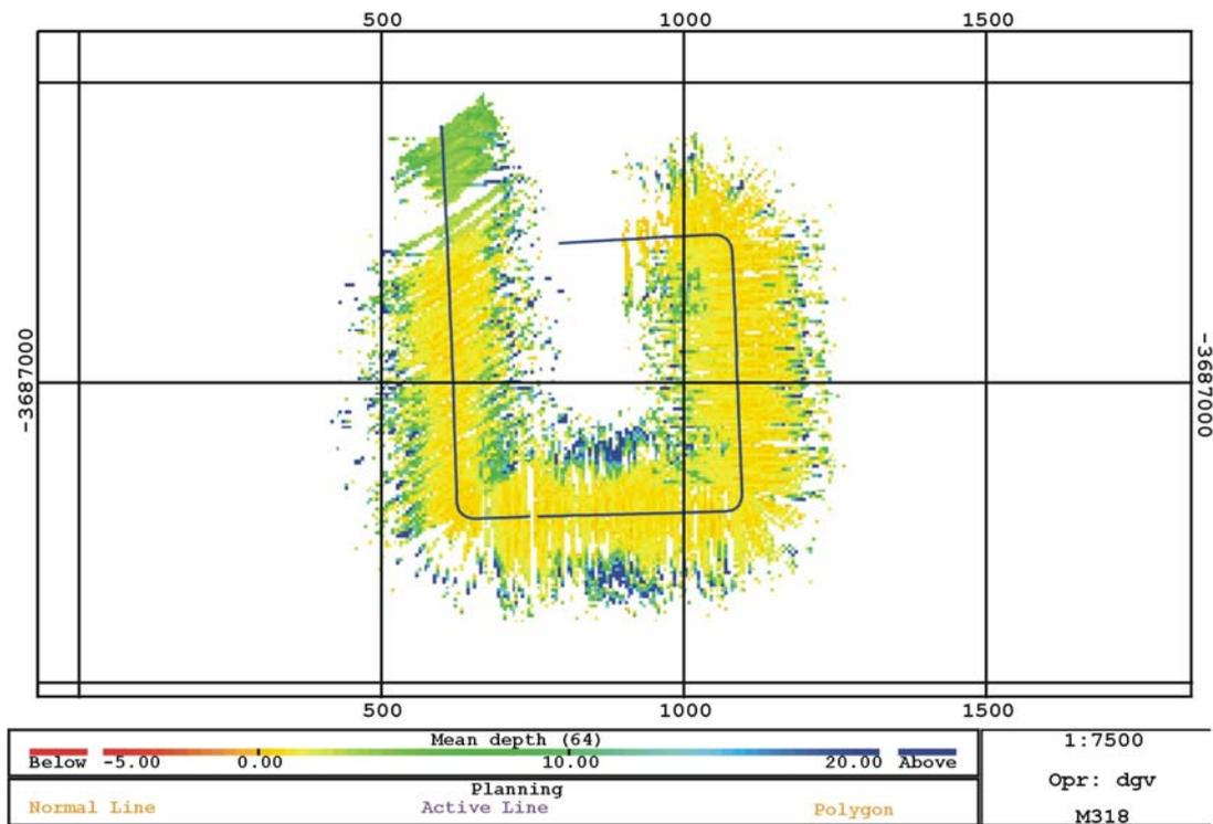
**Figure 30:** Autosub EM2000 data from Mission M318, showing strong sea surface return.
