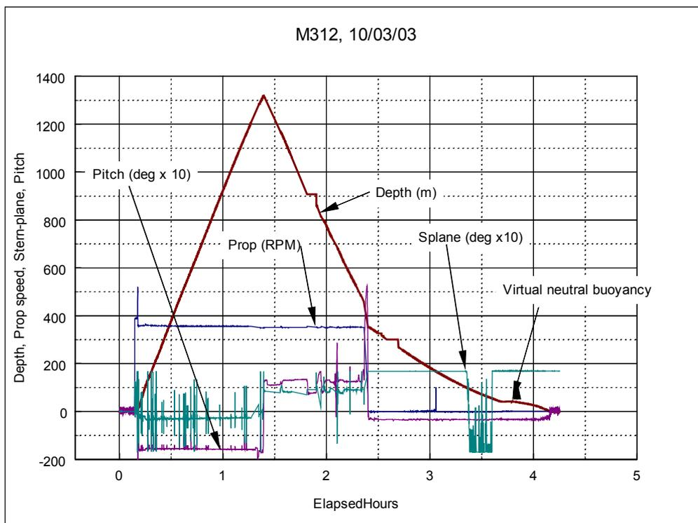
**Figure 18:** Mission 312 prior to adding more buoyancy
