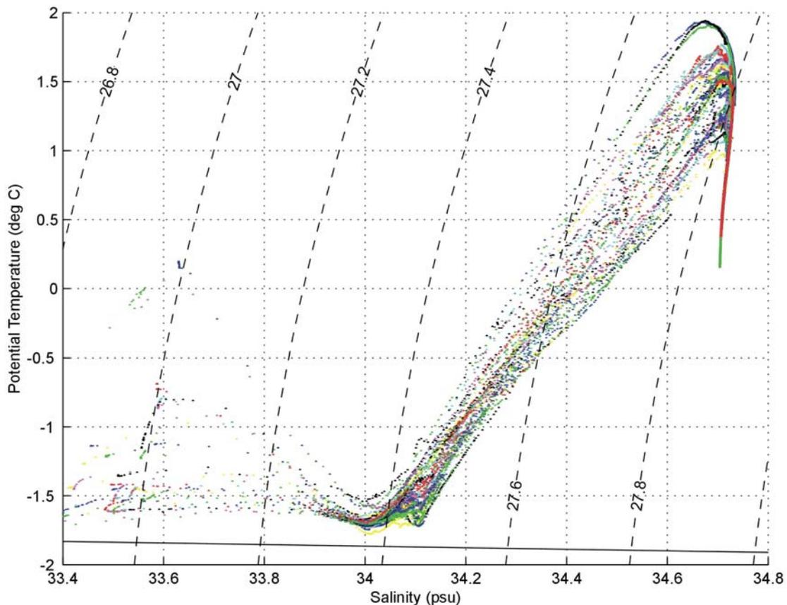
**Figure 7:** Scatter plot of potential temperature versus salinity data (2 dbar averages) from CTD stations 2 to 44. The solid black line indicates the surface freezing point, the labelled, dashed lines are isopycnals referenced to surface pressure
