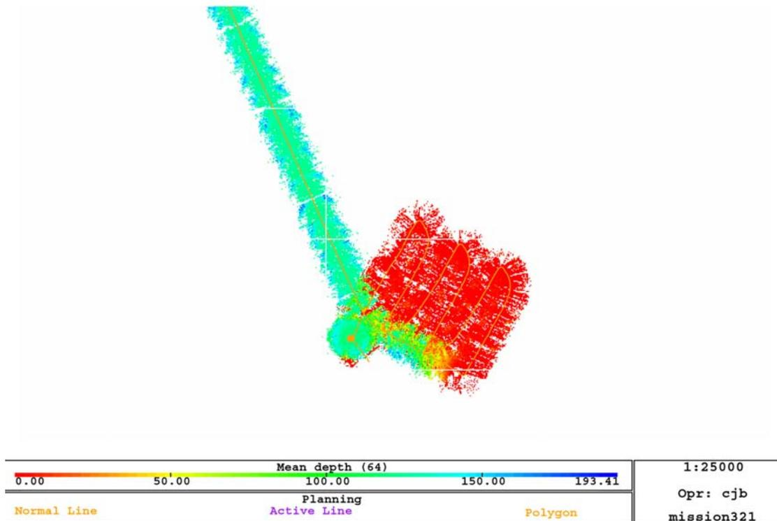
**Figure 33:** Results of Raw Multibeam Sonar Analysis of Ice Draft for Autosub Mission 321
