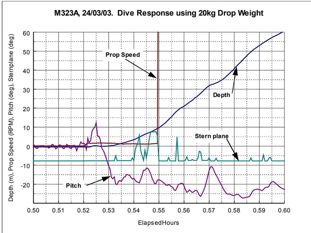
**Figure 19:** Vehicle Dive Response using the sink weight
