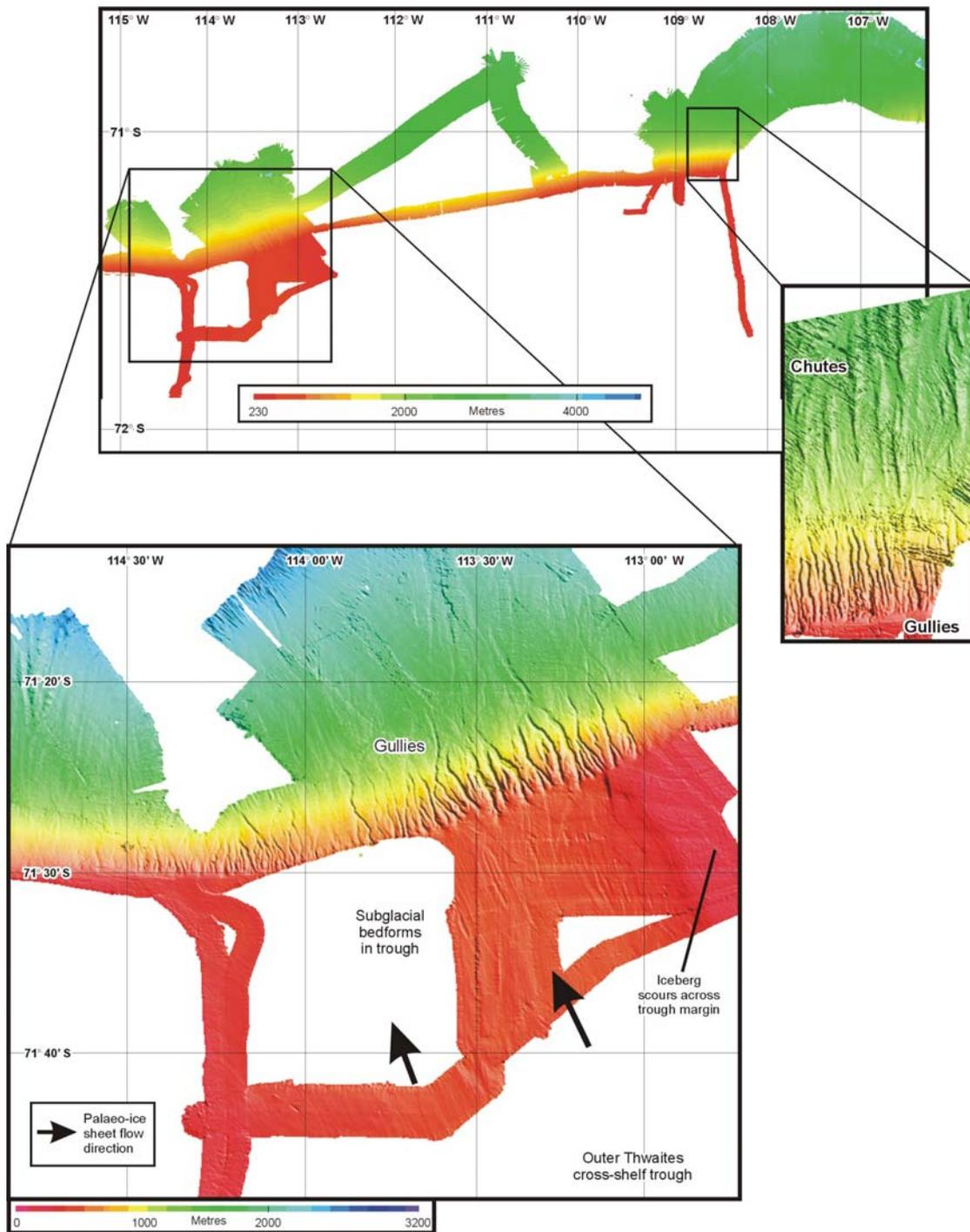
**Figure 2:** JR84 swath-bathymetric coverage between 107° and 115 W° on the Amundsen Sea continental margin offshore of Pine Island Bay. Gullies and chutes can be seen on the upper continental slope. The outer shelf is scoured by icebergs at shallower depths, and glacial lineations are also observed in the 'Thwaites Trough'.
