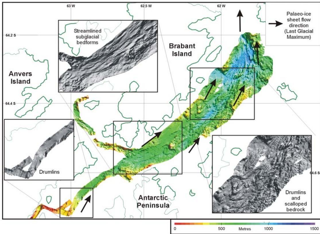
**Figure 4:** Swath bathymetry of the Gerlache Strait, western Antarctic Peninsula. Streamlined glacial erosional and depositional forms are illustrated and are used to infer the direction of past ice flow.
