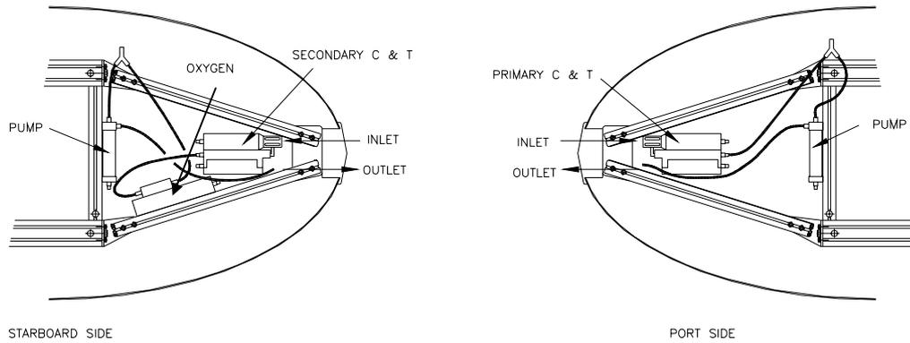
**Figure 21:** Configuration of CTD and associated sensors after mission 319
