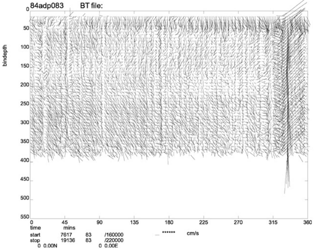
**Figure 17:** Arrow graph plot of .abs file ADCP data for duration of CTD deployment
