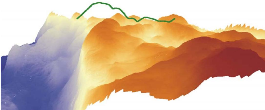
**Figure 22:** Autosub 100m altitude terrain following track over Gerlache Strait Bathymetry
