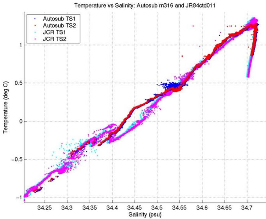
**Figure 38:** Comparison of Autosub and ship’s CTD temperature/salinity values.
