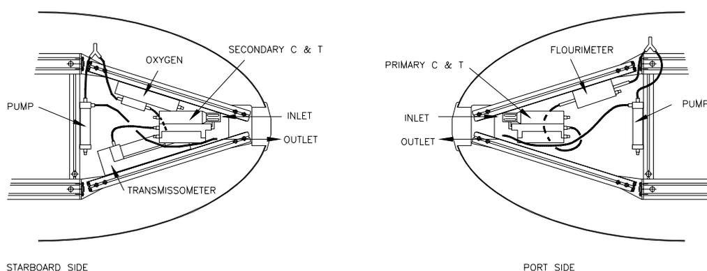
**Figure 20:** Configuration of CTD and associated sensors for missions 307 to 319 inclusive
