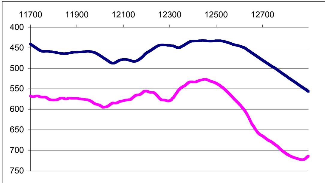
**Figure 28:** Comparable segment showing Autosub track (top) and bathymetry from shipborne EM120 system. Here y-axis is depth in metres, x-axis is tracenumber.
