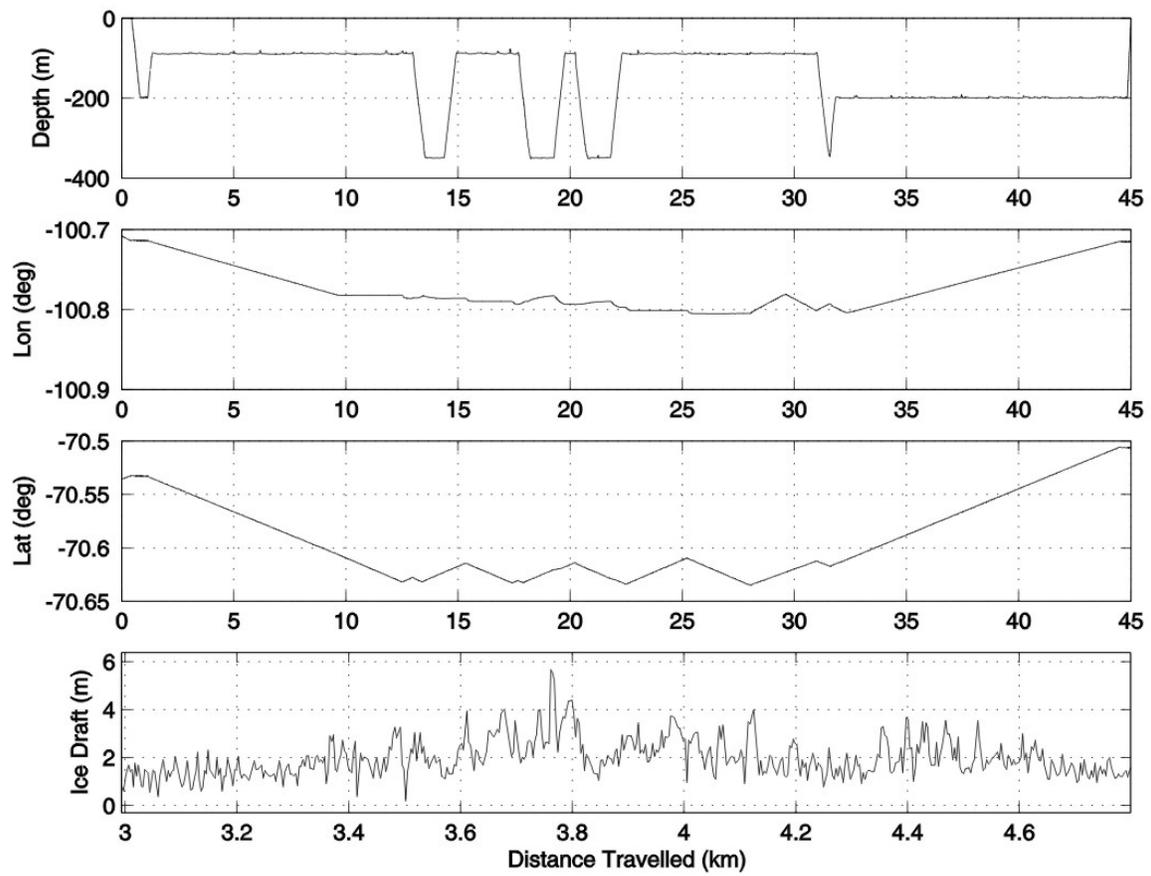
**Figure 40:** Autosub position and derived ice draft during M323.
