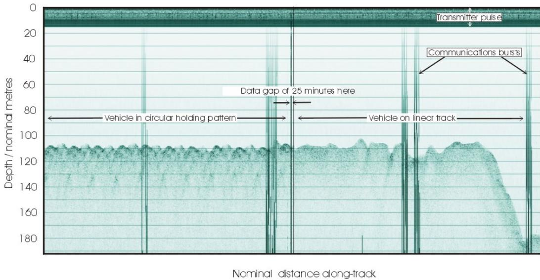
**Figure 24:** Jstar captured data from M309, and then tarted up in Coreldraw, showing the main features of the record.
