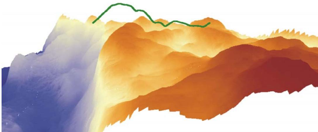
**Figure 22:** Autosub 100m altitude terrain following track over Gerlache Strait Bathymetry
