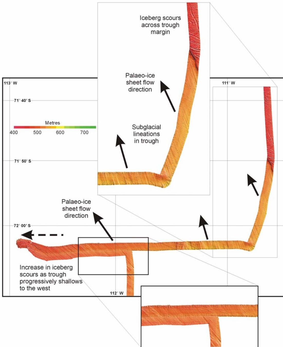
**Figure 3:** Swath bathymetry showing glacial lineations in sediments of the Thwaites Trough. The direction of past glacier flow can be inferred from the orientation of the lineations. Icebergs scours are present in shallower areas.
