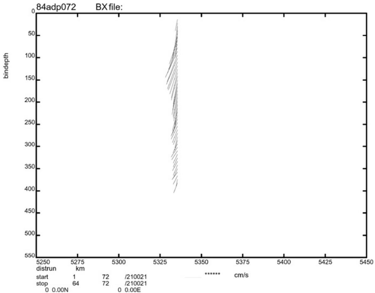
**Figure 16:** Arrow graph plot of time averaged on-station ADCP data
