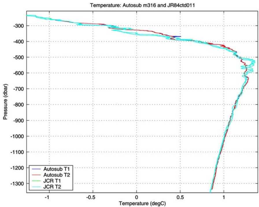
**Figure 36:** Comparison of Autosub and ship's CTD temperatures.
