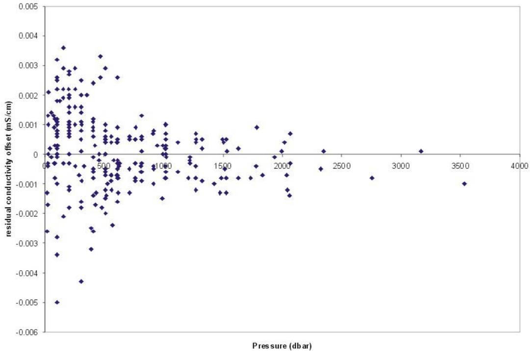
**Figure 12:** Residual offsets of the corrected CTD data against pressure for the JR84 data set.
