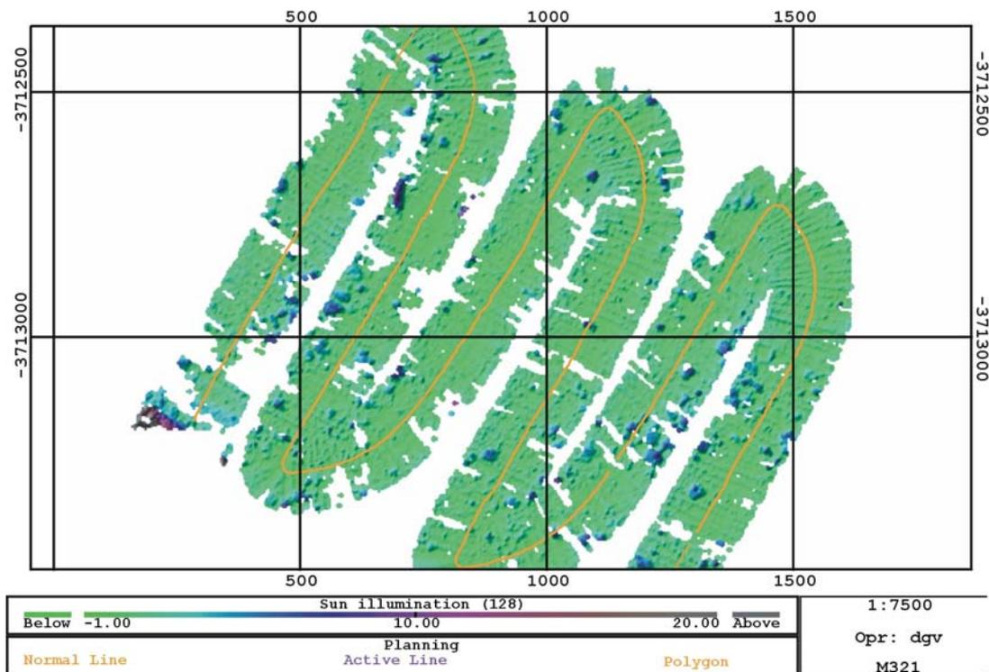
**Figure 31:** Autosub EM2000 swath bathymetry data from the underside of sea ice collected during M321.
