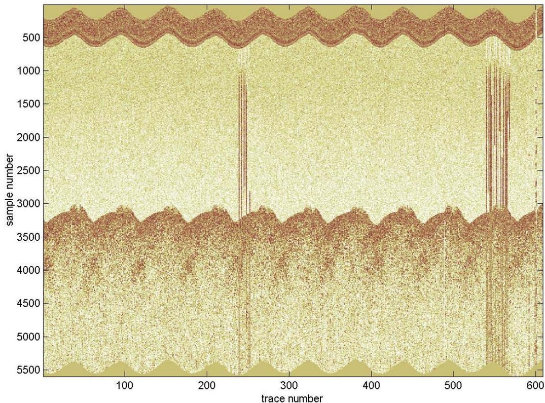
**Figure 15:** First segment from M309 corrected for sub depth. The upper lines is the transmitter pulse reflecting the changing vehicle depth and the bottom line is the seabed reflection.
