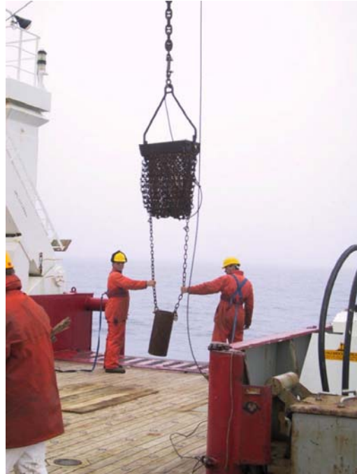
Fig. 5 Dredge deployment from aft deck
