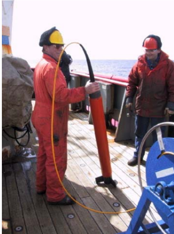
Fig. 7 Seaspy towfish and cable reel
