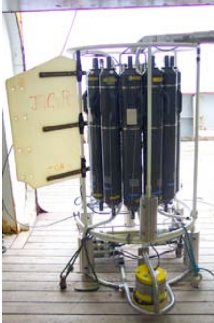
Figure 3.1: Positioning of the LADCP unit on the CTD frame.
