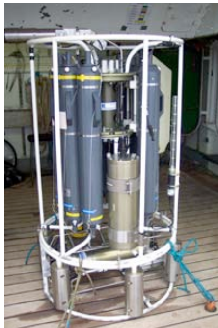
Figure 3.2: Positioning of the battery pack on the CTD frame.
