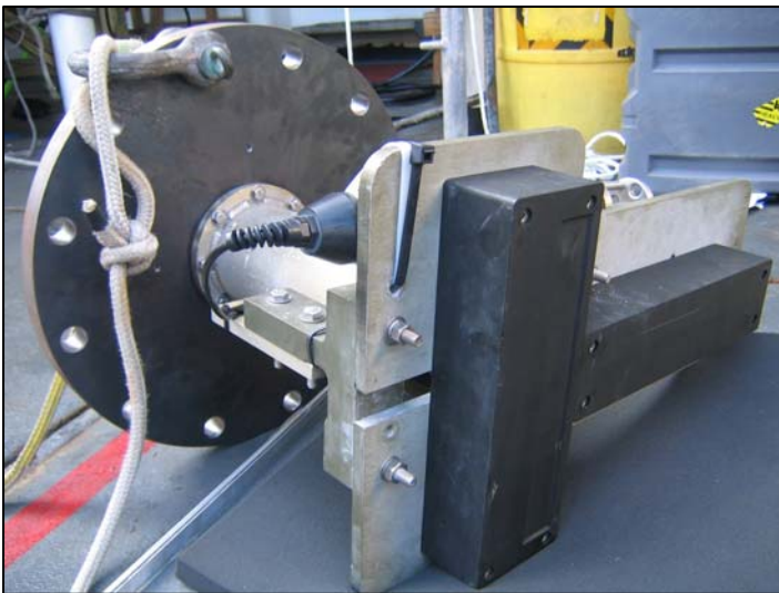
Fig 3: 8124 transducer w/moon pool flange mount
