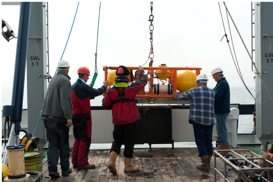
Figure 2. First instrumented deployment of the new sea bed frame.
