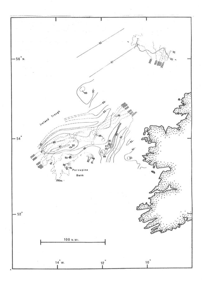
A further belt of magnetic high values runs parallel to, and slightly to the west of, the 200 metre isobath. This is a linear feature of maximum amplitude about 500 gammas, of width about 30 km, and length 100 km.
