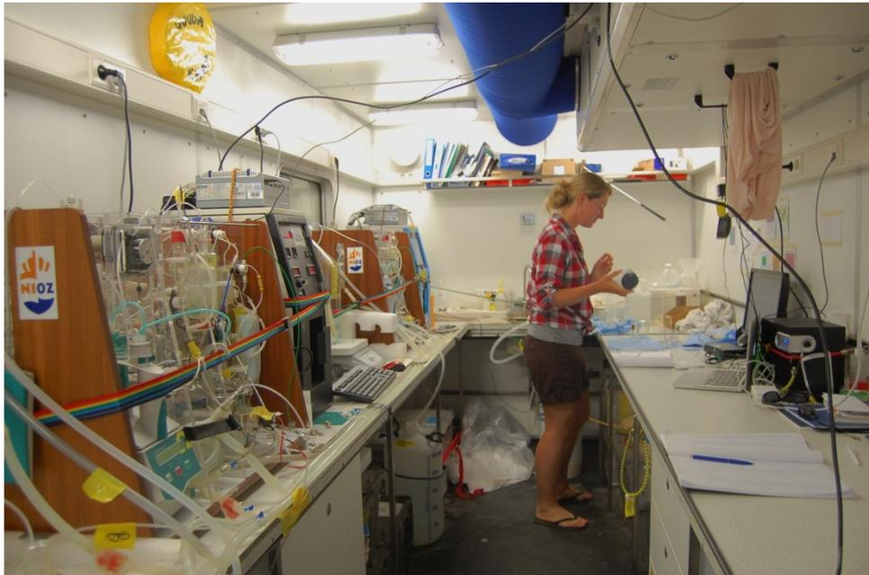
Figure 34. Lesley measuring DIC and alkalinity in the dedicated CO<sub>2</sub> container.
