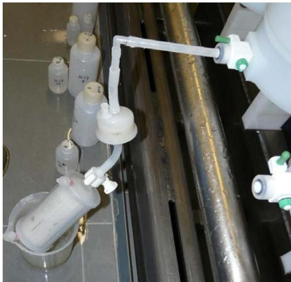
Figure 25. Ultrafiltration of seawater samples directly from the UCC CTD bottles.
