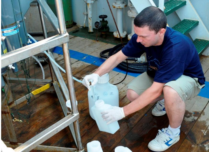
Figure 30. Damien sampling seawater from the 12L CTD for particles.
