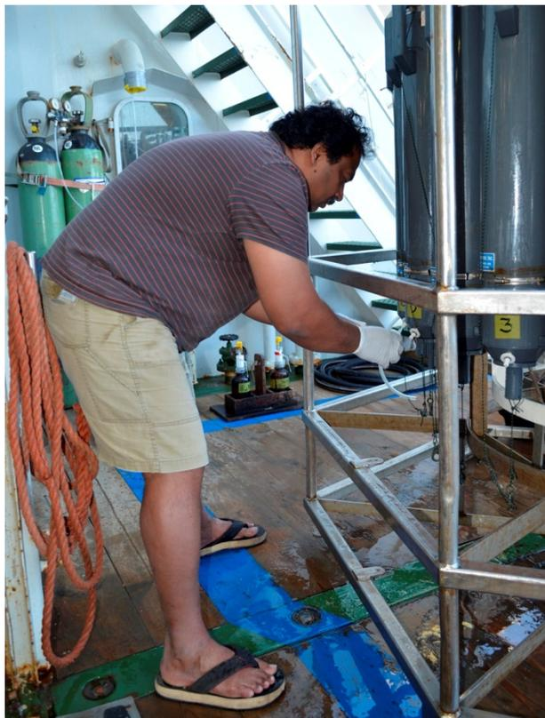
Figure 32. Raja sampling seawater from the standard 12L CTD to collect particles.
