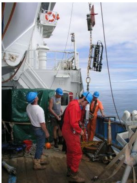
Fig. 6. The SAMS mooring ready to be deployed. Hanging in the air are the current meter and the datalogger with fluorometer and OBS.
