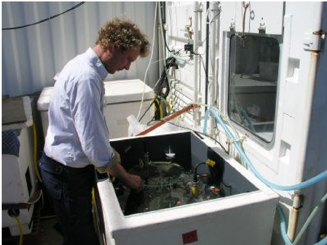
Fig. 10. Rob Witbaard busy with his oxygen consumption measurements of live coral in a thermostated aquarium.
