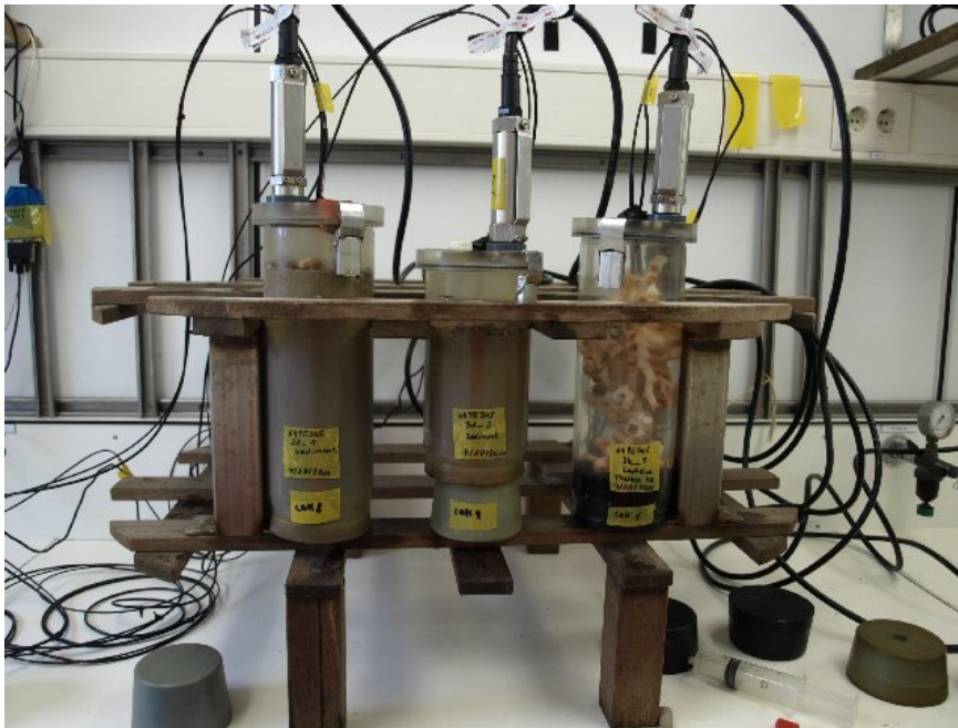
The incubation set-up in the cool container with 2 sedimentcores and one with coral.
