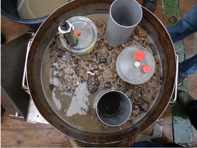
Fig. 5: Boxcore sample with inserted incubation chambers.
