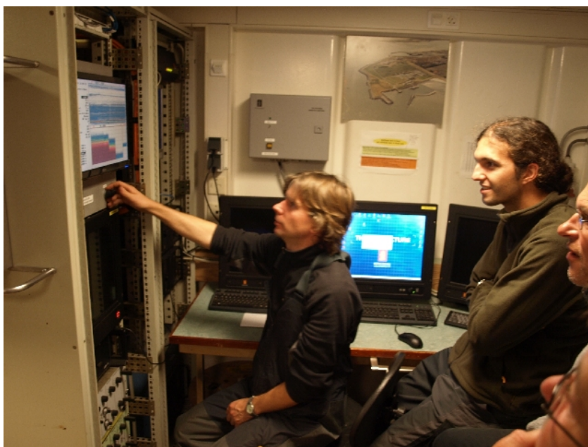
Fig. 9 The Simrad EK 500 fishery research echo sounder in operation.
