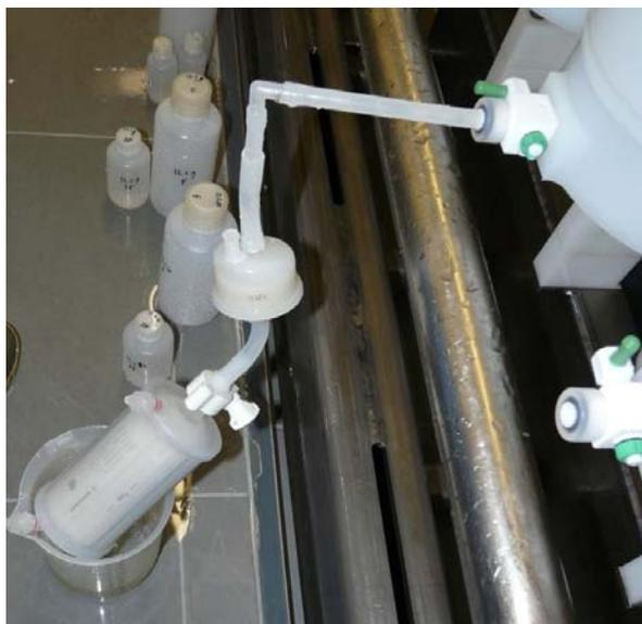
Figure 23. Ultrafiltration of seawater samples directly from the UCC CTD bottles.
