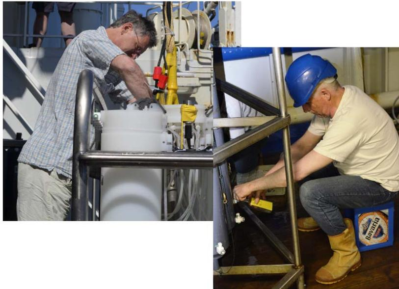
Figure 21. Ruud Groenewegen (left) prepares the UCC for deployment and Sven Ober (right) takes samples for salinity from the 25L CTD frame 64PE370.
