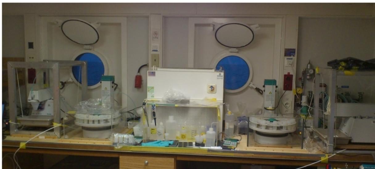
Figure 25) Equipment setup to measure the organic complexation of Fe using voltammetry during 64PE370
