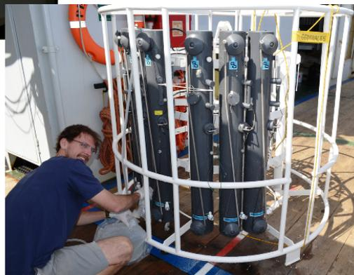
Figure 15. The sample equipment used to take trace metal clean and non-trace metal clean water samples during 64PE370.
