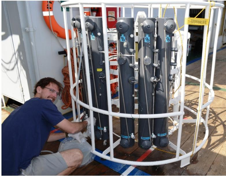
Figure 20. John Rolison sampling for metal isotopes from the brine frame deployed in the Bannock basin during 64PE370.
