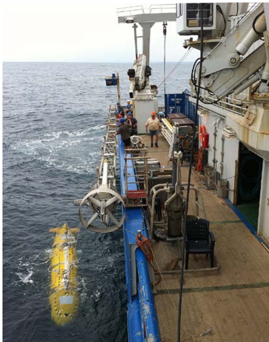
Autosub3 being recovered (left) and the EdgeTech sidescan sonar (right)
