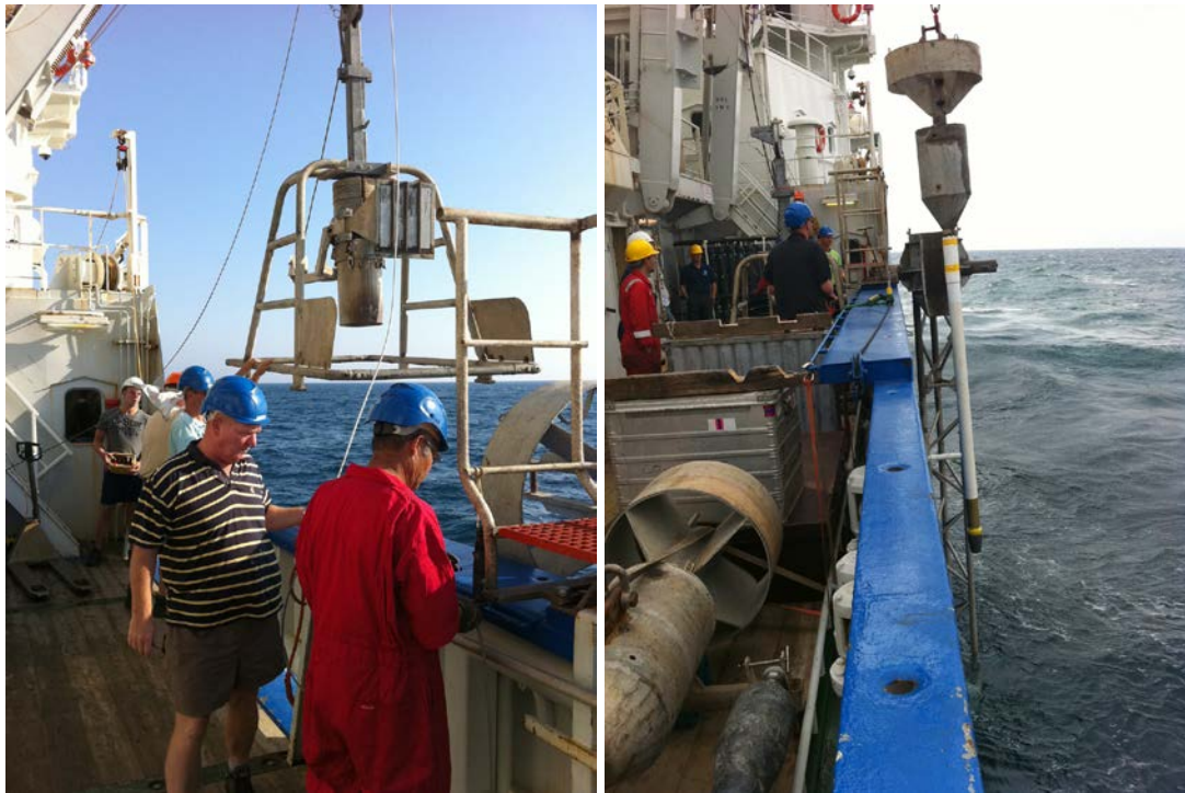
The NIOZ box corer (left) and gravity corer (right)
