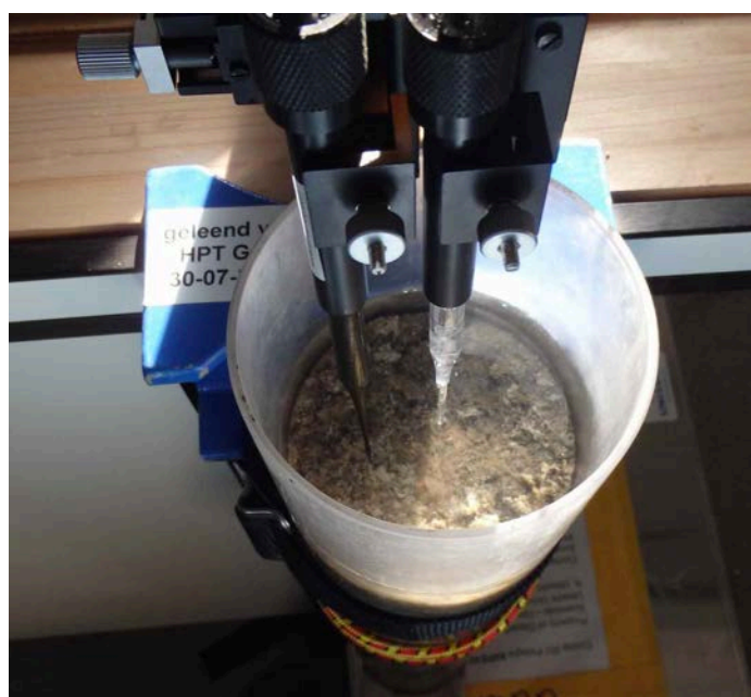
Figure 19. Micro-electrode profiling set-up
