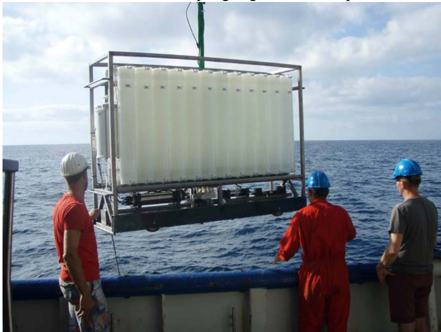
Figure 7 Deployment of ultraclean CTD
