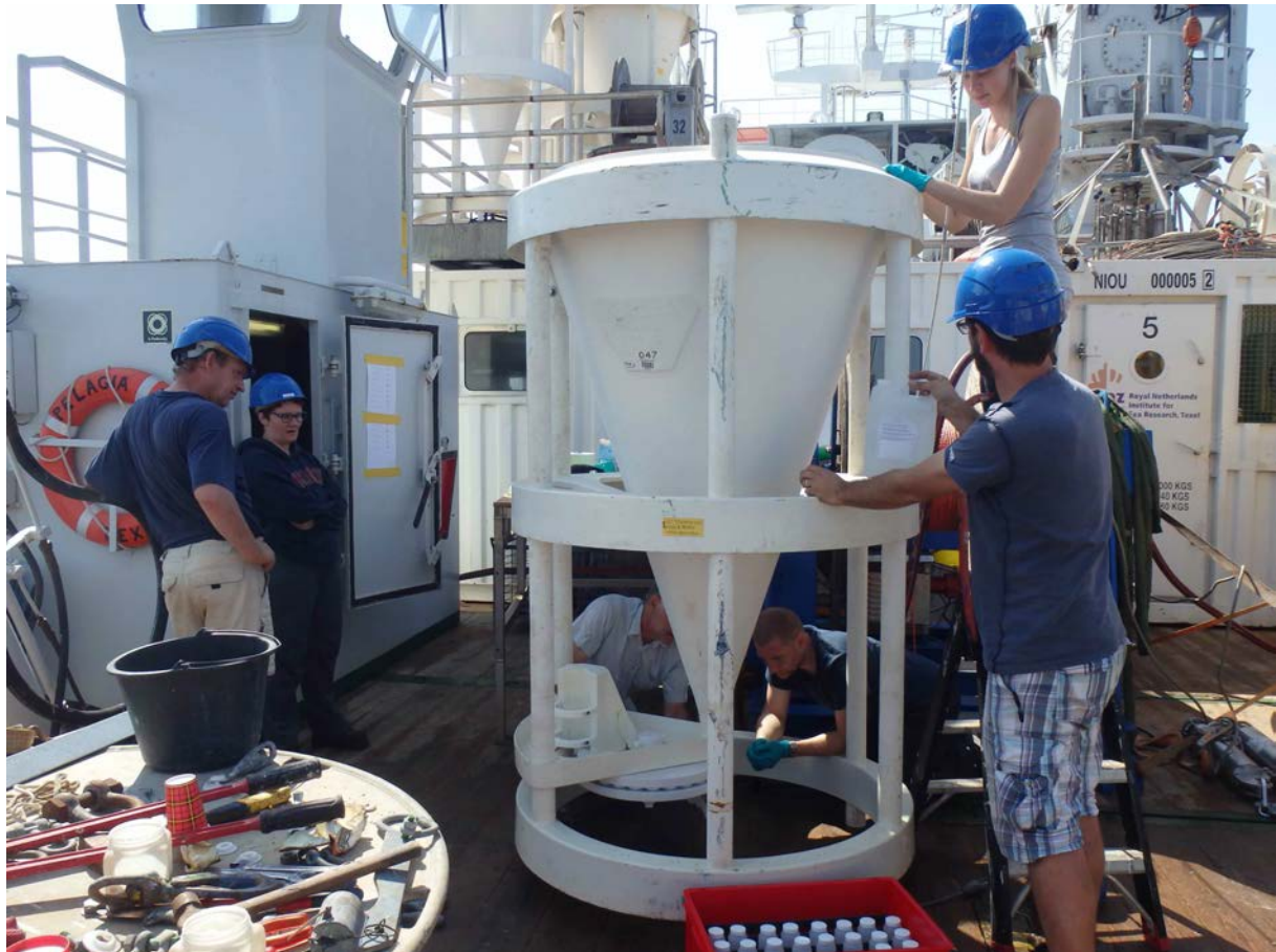
Figure 12. Preparing a sediment trap for deployment
