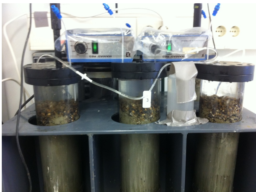
Figure 27. Setup of anoxic incubation experiment
