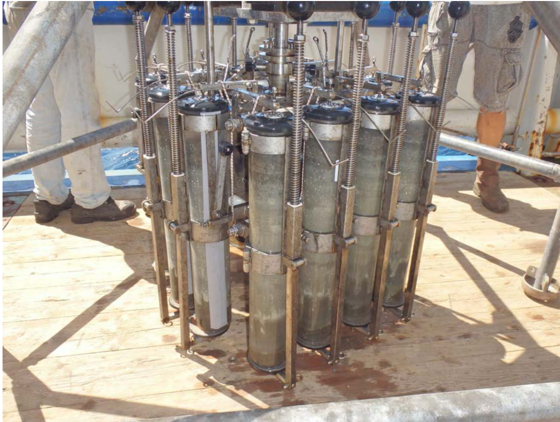
Figure 8. Multicore cast collected at station 1
