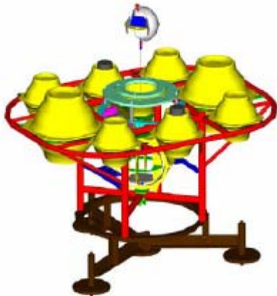
Figure 5.4. Schematic drawing of HOMER (without shear microstructure sensors)
