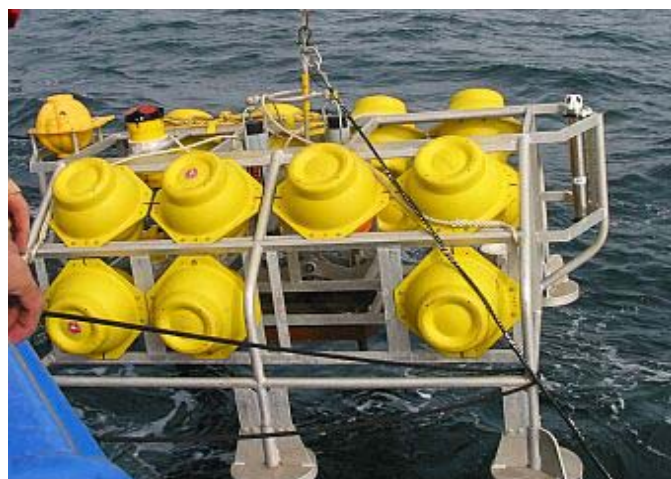
Figure 5.5b. NIOZ bottom lander, with ARGOS transmitter (far top-left) 300 KHz ADCP (top-left) and 2 extra battery containers below ADCP (difficult to see), AquaDopp (top far-right), 2 acoustic releases (grey/black cap central pipes) and free suspended dropping weight. The black cable attached to the central top and free hanging to the lower-right is the NIOZ thermistor string (leading to the buoy already in the water).
