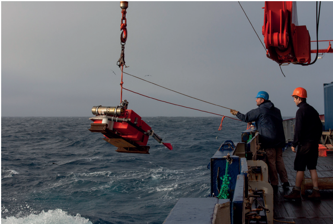
Fig. 3.2.2: Deployment of an OBS
