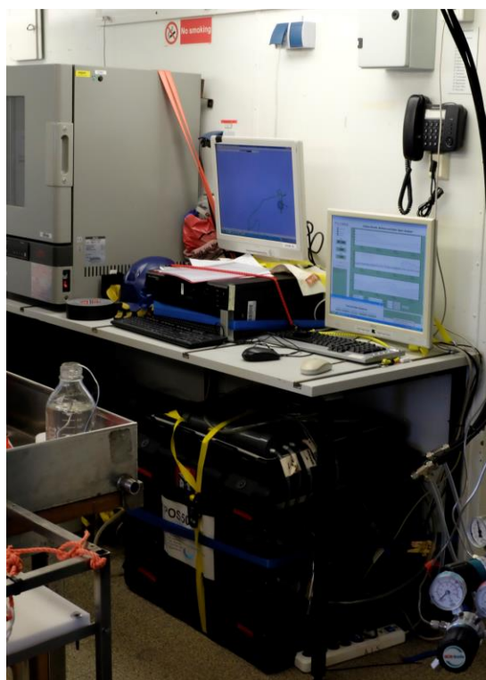
Fig. 32: Atmosphere intake system (AIS) with the Picarro measurement control computer (right computer screen) and the OFOP data logging computer (left computer screen) in the wet-lab.
