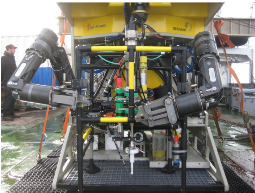
Fig. 11: The eddy covariance instruments on the ROV's porch just prior to deployment.
