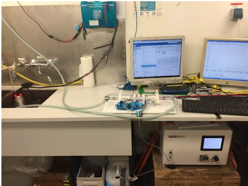
Fig. 18: Setup of the autonomous TA-System in the wetlab of RV Poseidon.
