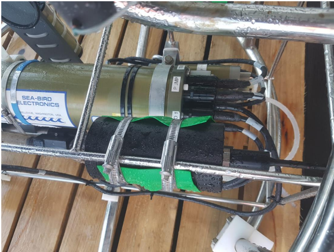
Figure 4. pH optode attached on the CTD frame
