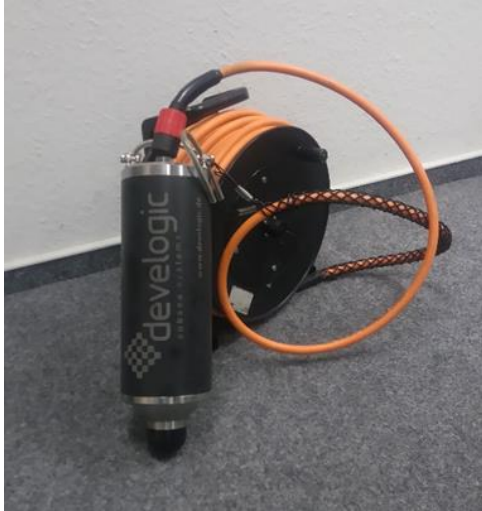
Figure 6. Surface hydro-acoustic modem for Develogic lander communication
