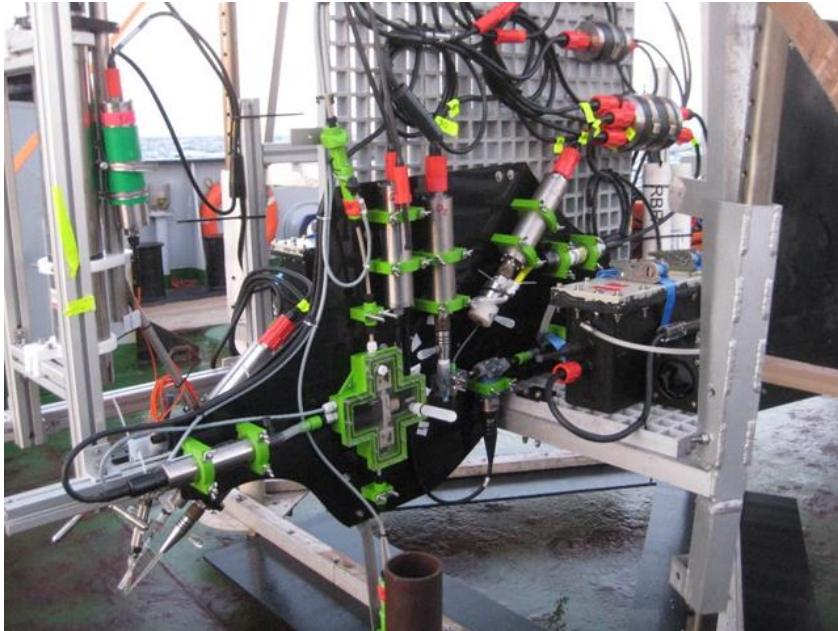
Figure 9. The gradient profiler developed to determine dissolved oxygen and pH at 0.1 m and 1.1 m above the seafloor in the benthic boundary layer.
