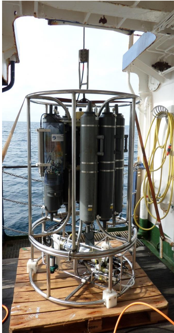
Figure 22. Alkalinity sensor (left) mounted on the CTD frame.
