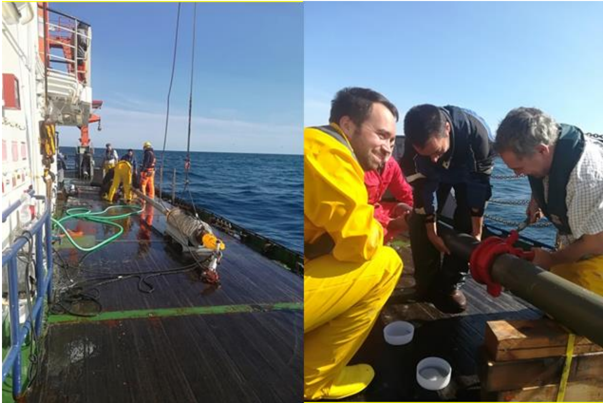
Figure 15. Left: Gravity core deployment; Right: cutting of the gravity core in 1 m sections
