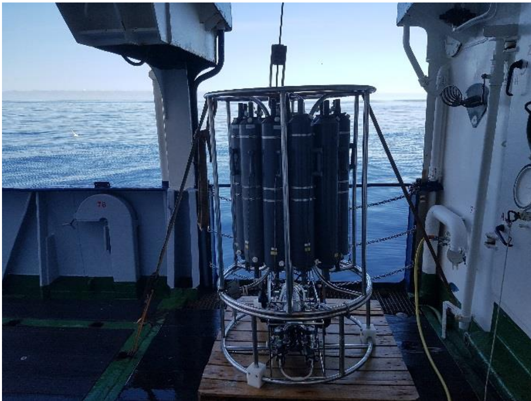
Figure 3 Water sampler (12x10 L Niskin) rosette and CTD sensors
