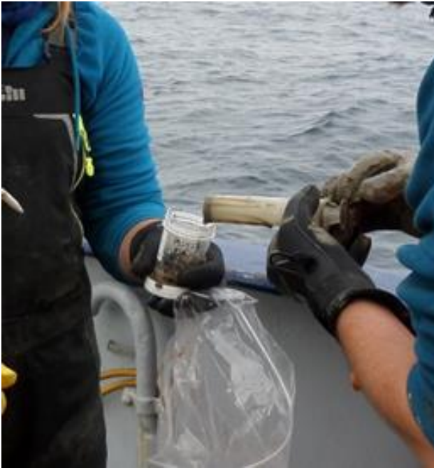
Figure 13. Subsampling of box corer for particle size analysis (PSA).
