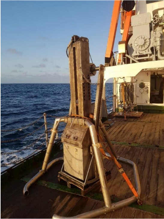
Figure 10. Box corer standing on deck of the Poseidon
