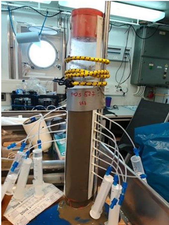
Figure 14. Pore water extraction with Rhizons in subsample of box core
