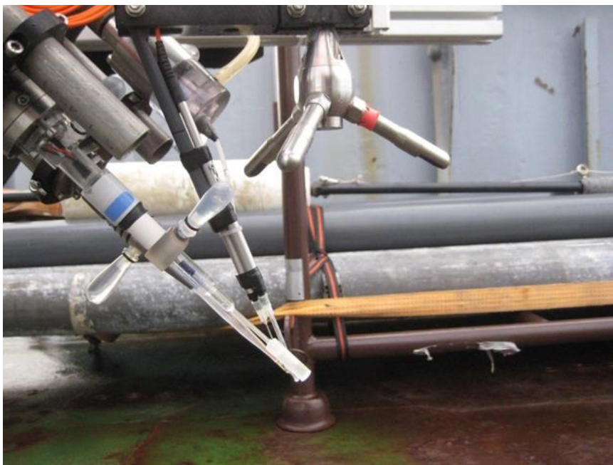
Figure 8. Eddy covariance oxygen and pH sensors positioned just outside the measuring volume of the acoustic Doppler
