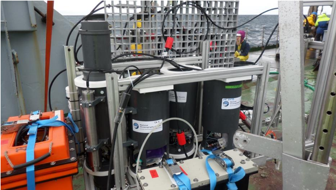
Figure 20. Four LOC sensors mounted on the MPI benthic boundary lander.
