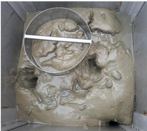
Figure 11. Sub-coring of box core after water is drained. Cracks in the sediment surface are a product of the force of the box-coring
