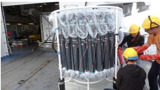
Clean rosette used in PEACETIME (left) Deployment preparation (right) Subsampling from clean rosette bottles respecting trace metal clean techniques (bottle were removed from the rosette and subsampling in clean container).
